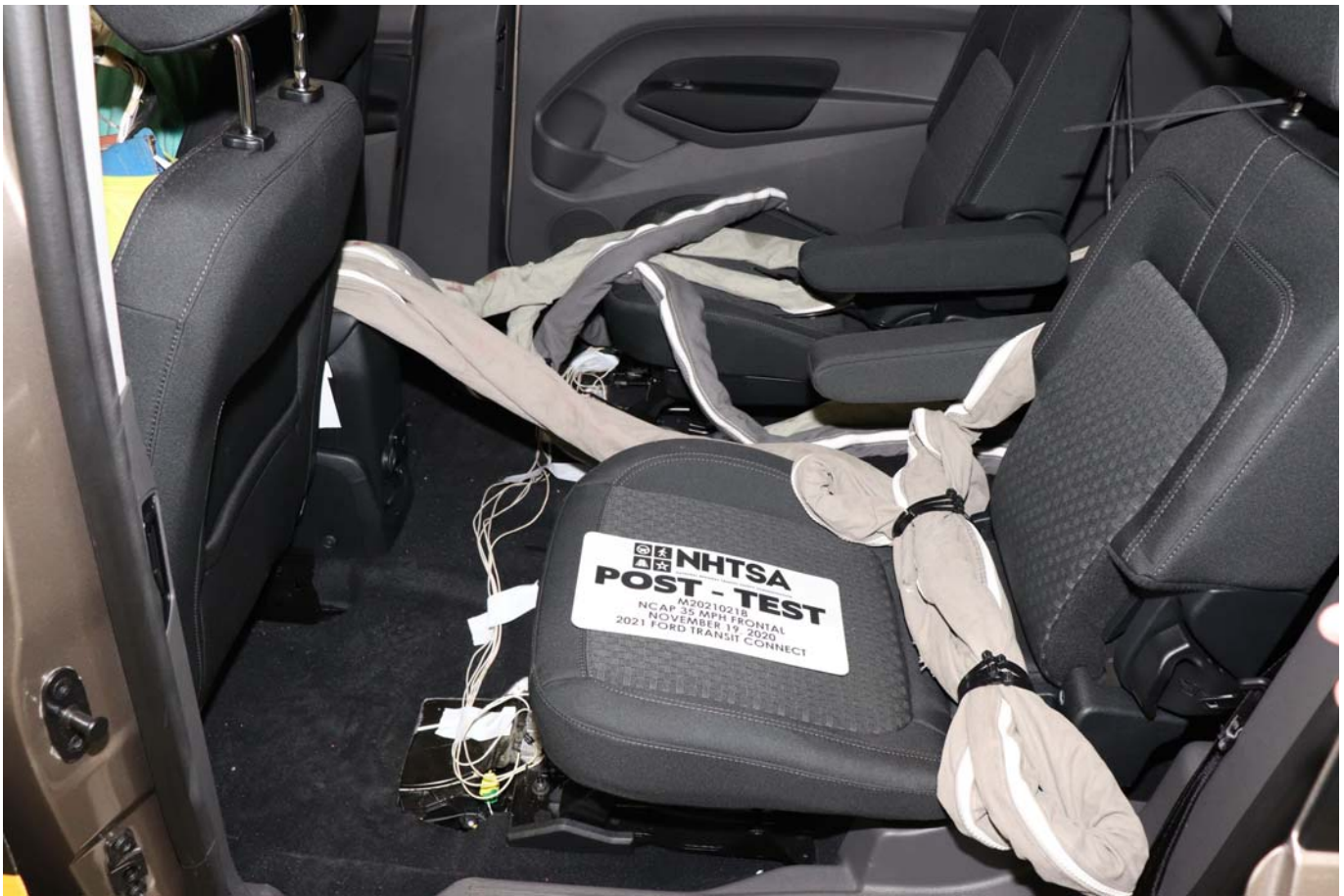
Photo No. 029 - Post-Test Dummy Cable Routing
