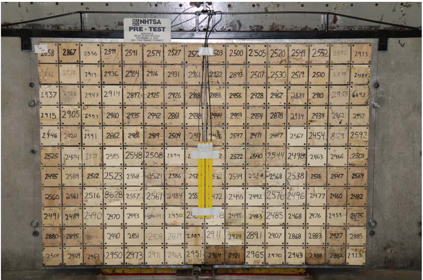
Photo No. 002 - Pre-Test Load Cell Wall
