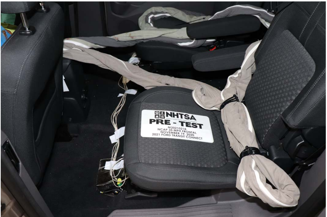
Photo No. 028 - Pre-Test Dummy Cable Routing
