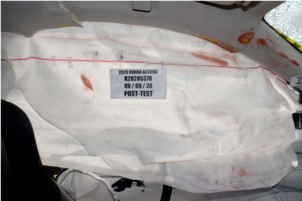
FIGURE 90. Post-Test Driver Dummy Contact with Side Airbag
