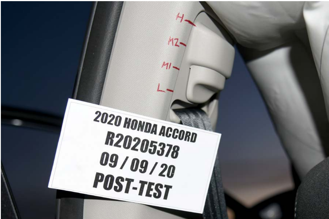
FIGURE 68. Post-Test Driver Adjustable D-Ring
