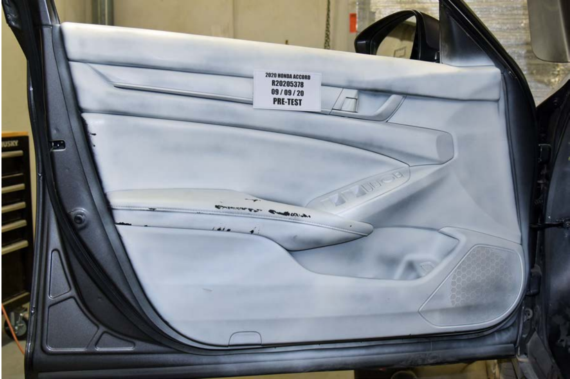
FIGURE 75. Pre-Test Driver Inner Door Panel
