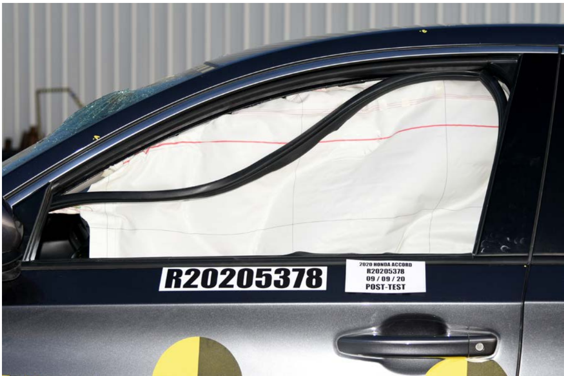
FIGURE 46. Post-Test Driver Side Front Window View
