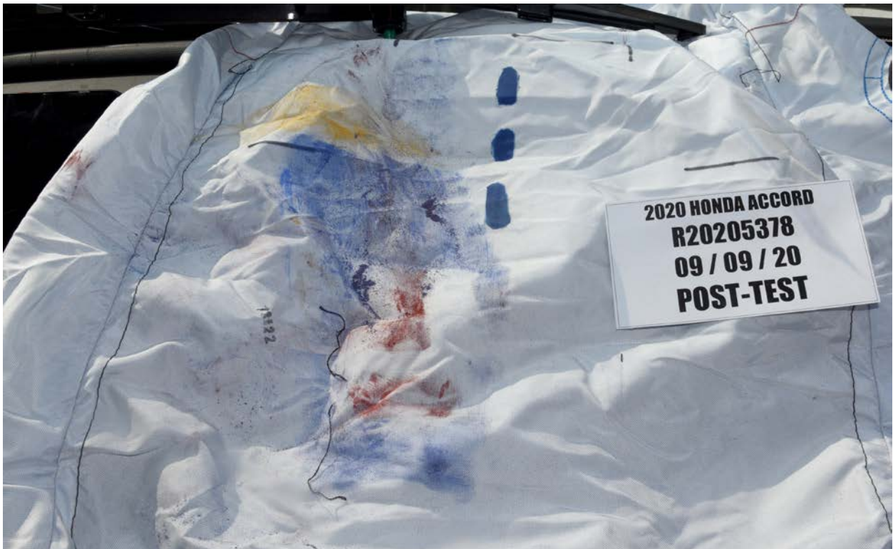
FIGURE 134. Post-Test Driver Dummy Contact with Front Airbag
