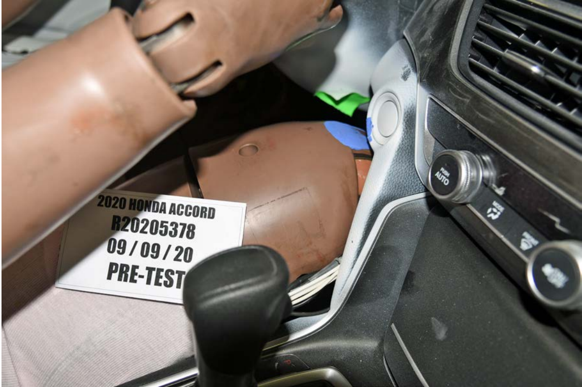
FIGURE 61. Pre-Test View of Driver Right Knee and Bolster
