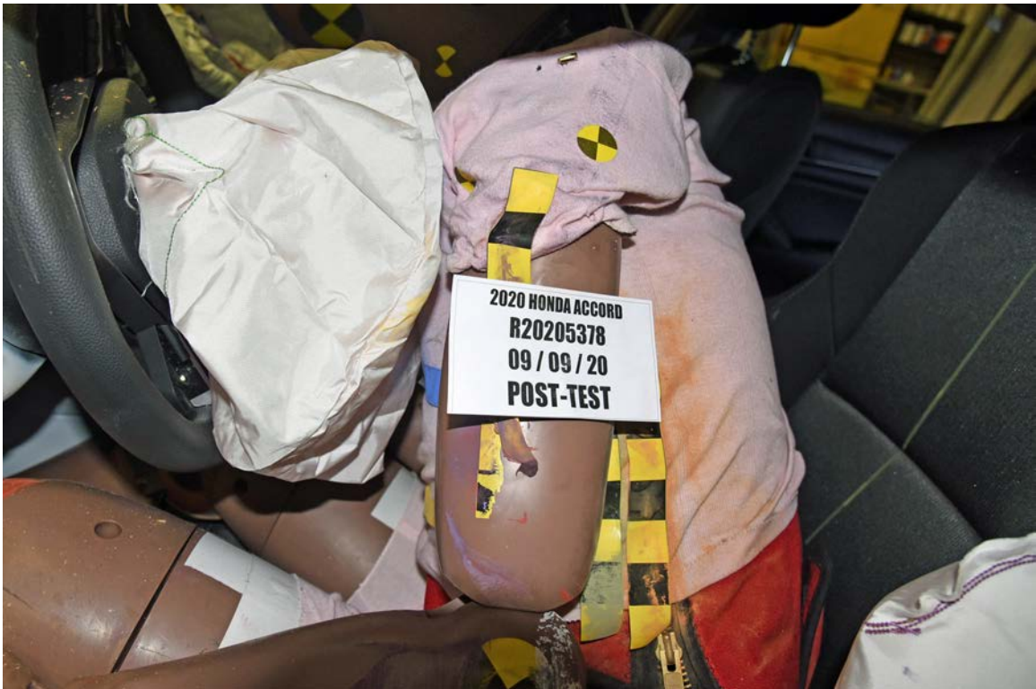
FIGURE 56. Post-Test View of Driver Abdomen
