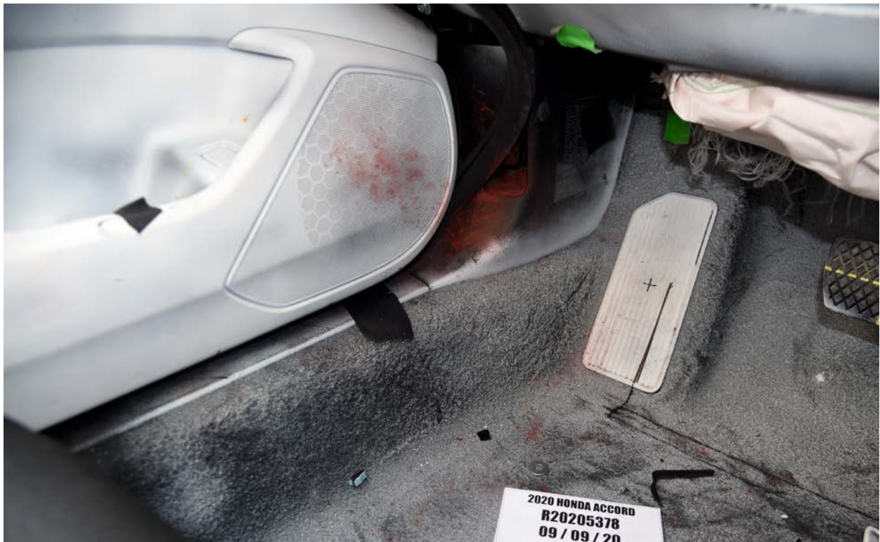
FIGURE 91e. Post-Test Driver Dummy Contact with Door Panel
