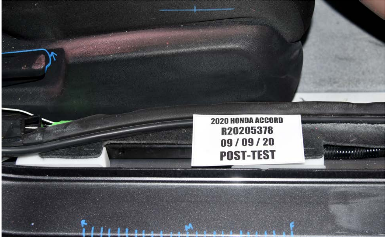
FIGURE 115. Post-Test Right Front Passenger Seat Fore-Aft Markings
