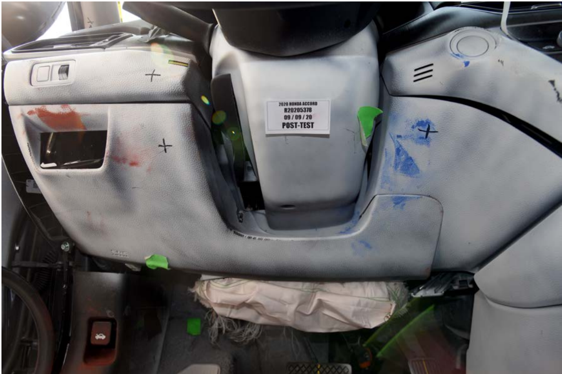
FIGURE 80. Post-Test Overall View of Driver Knee Bolster
