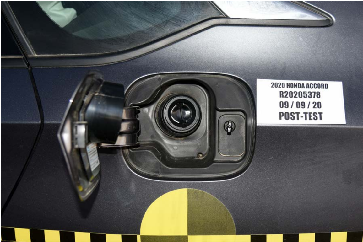
FIGURE 26. Post-Test Fuel Filler Cap View
