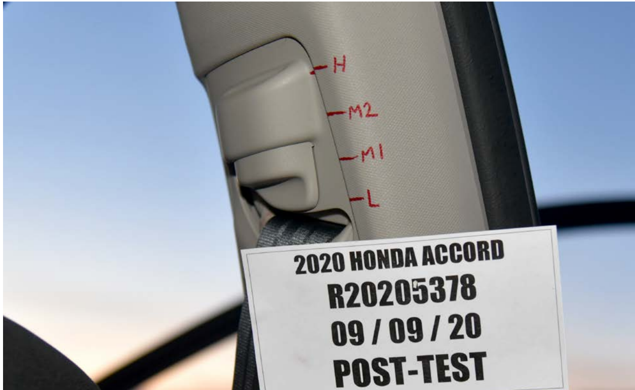
FIGURE 113. Post-Test Passenger Adjustable D-Ring
