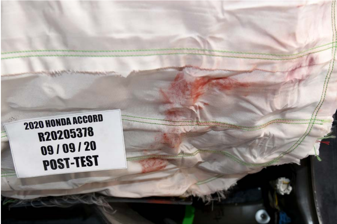
FIGURE 91. Post-Test Driver Dummy Contact with Knee Airbag
