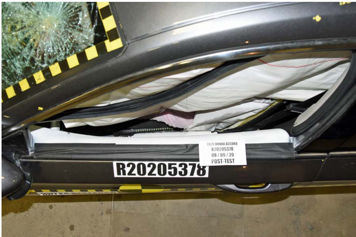
FIGURE 48. Post-Test View of Driver Door Clearance
