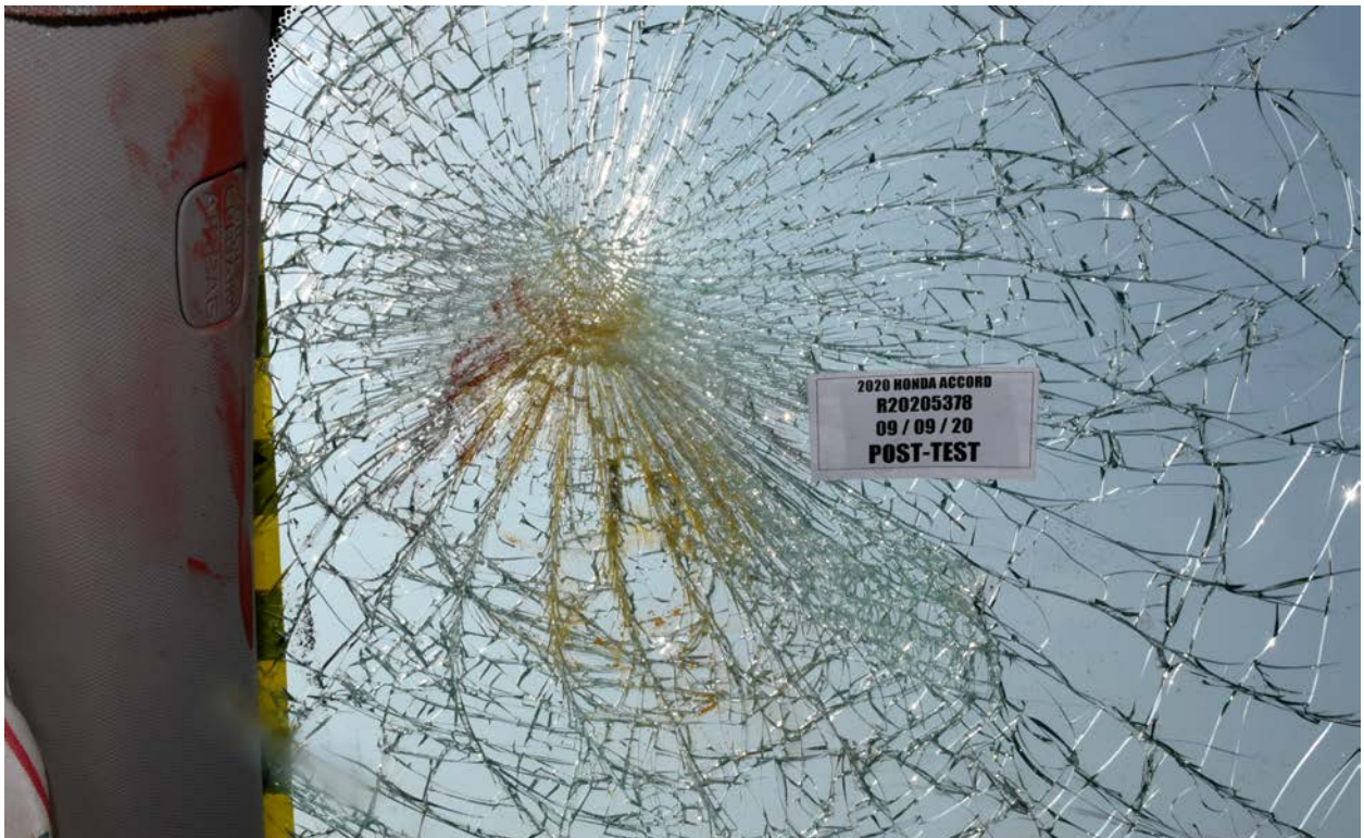
FIGURE 91c. Post-Test Driver Dummy Contact with Windshield
