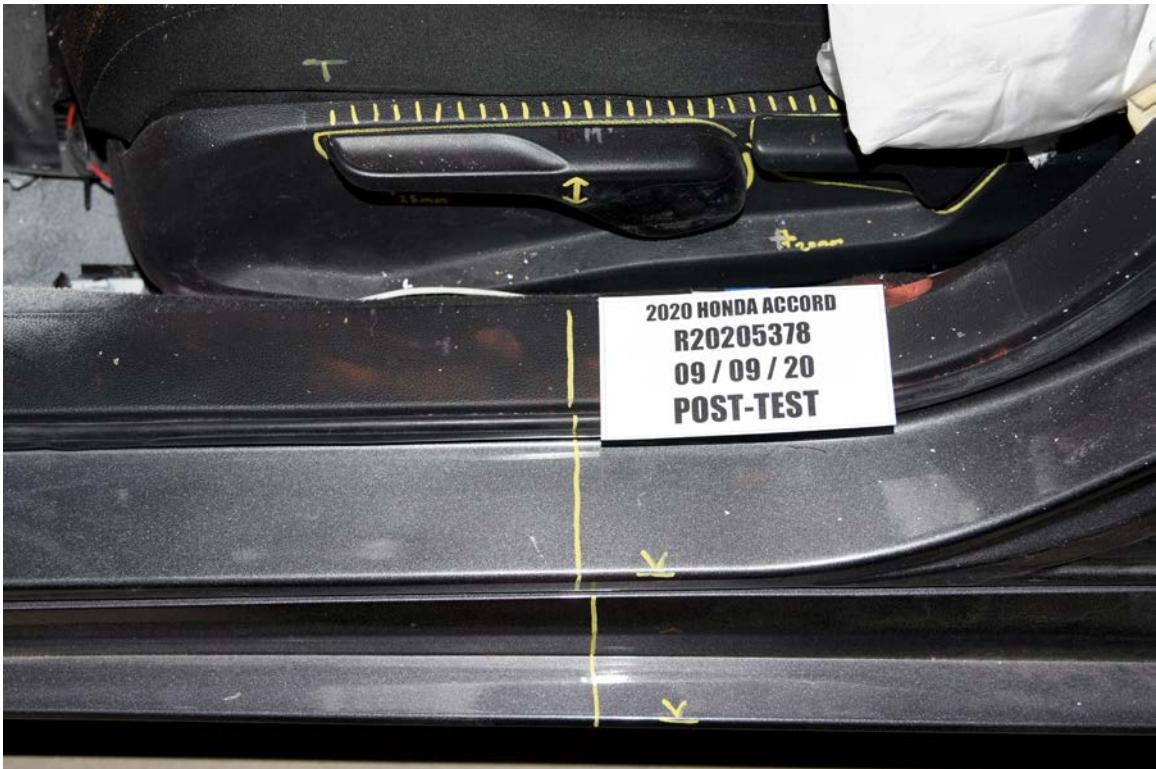
FIGURE 70. Post-Test Driver Seat Fore-Aft Markings
