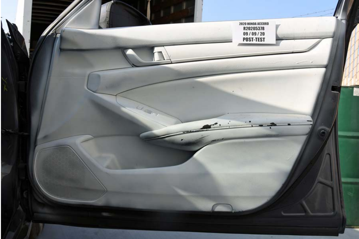
FIGURE 121. Post-Test Passenger Inner Door Panel
