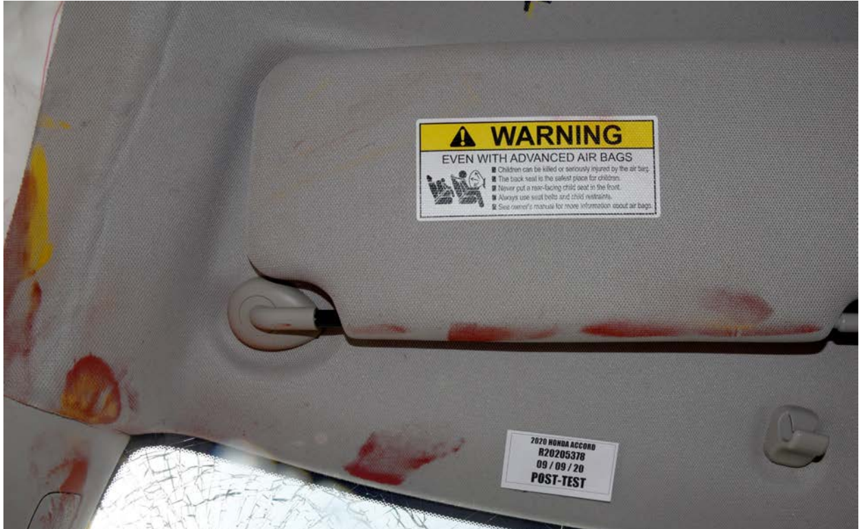
FIGURE 91d. Post-Test Driver Dummy Contact with Headliner
