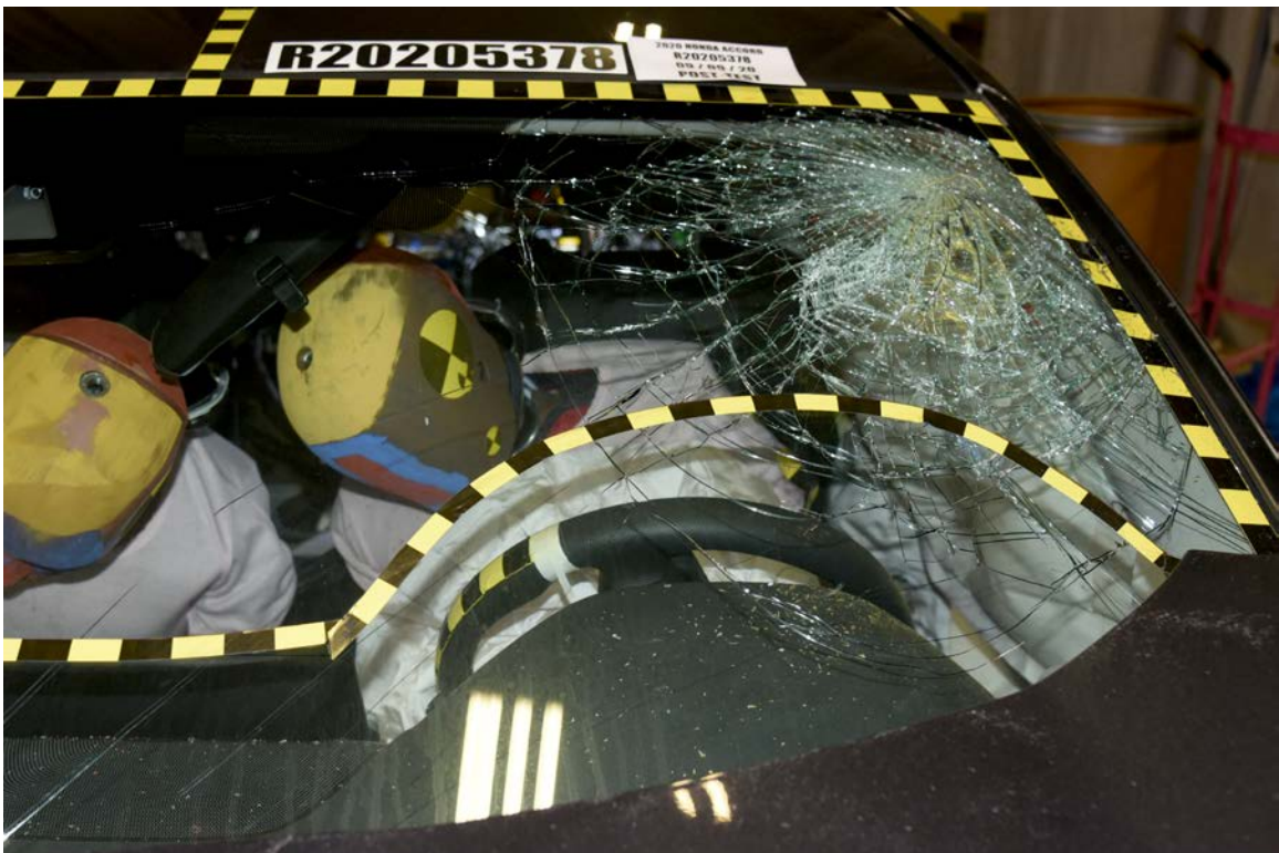
FIGURE 44. Post-Test Driver Front Windshield View
