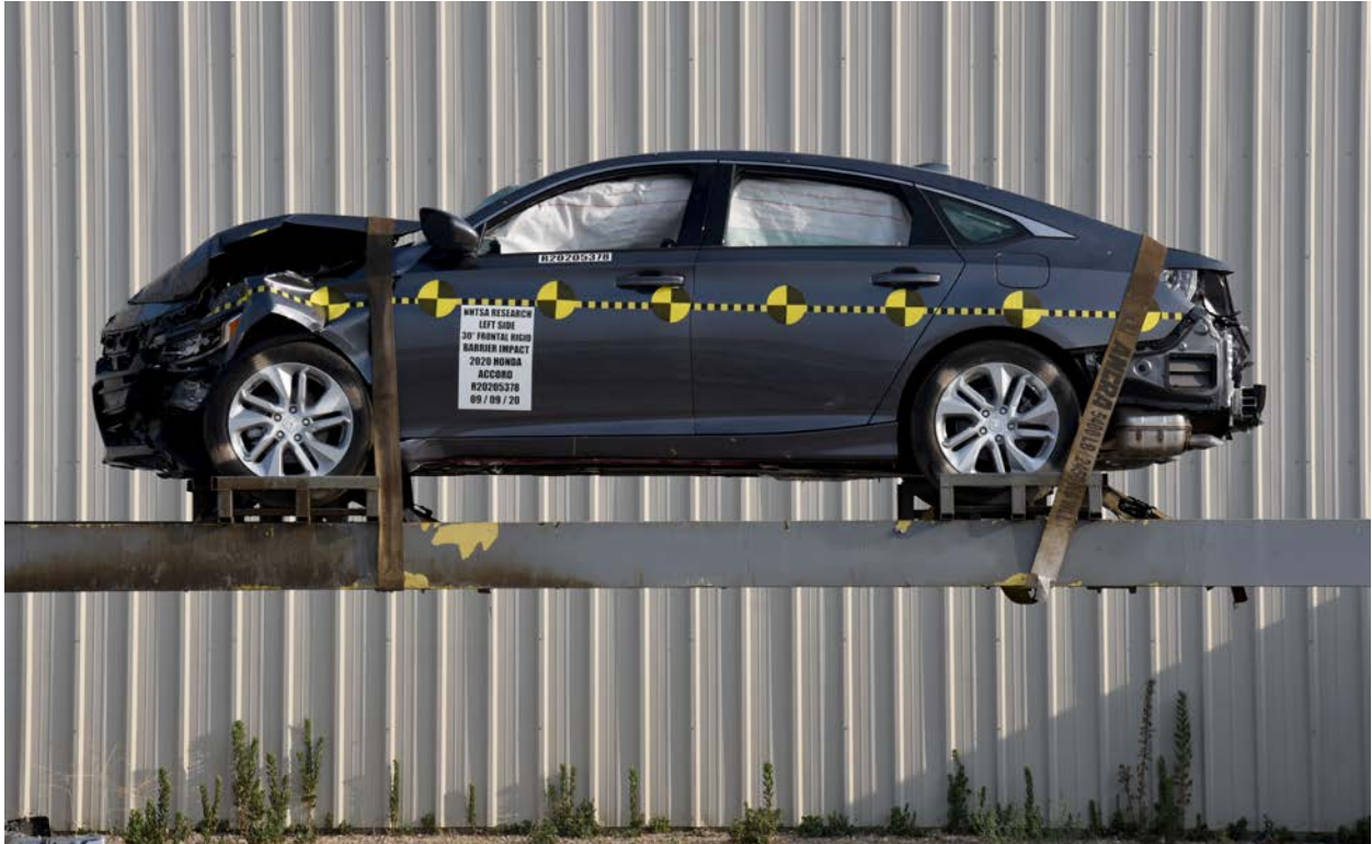
FIGURE 140. Vehicle at 0° on Static Rollover Device
