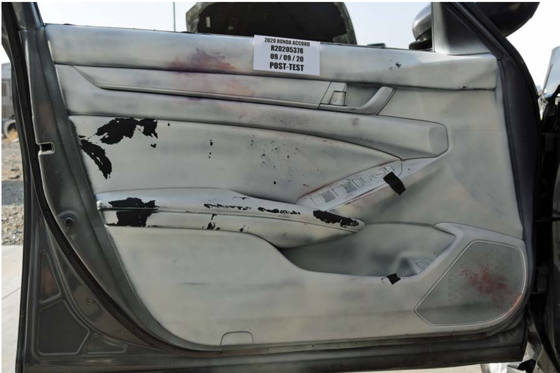
FIGURE 76. Post-Test Driver Inner Door Panel
