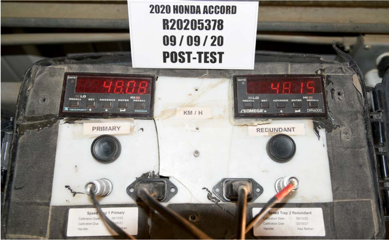
FIGURE 139. Post-Test Speed Trap Read-Out
