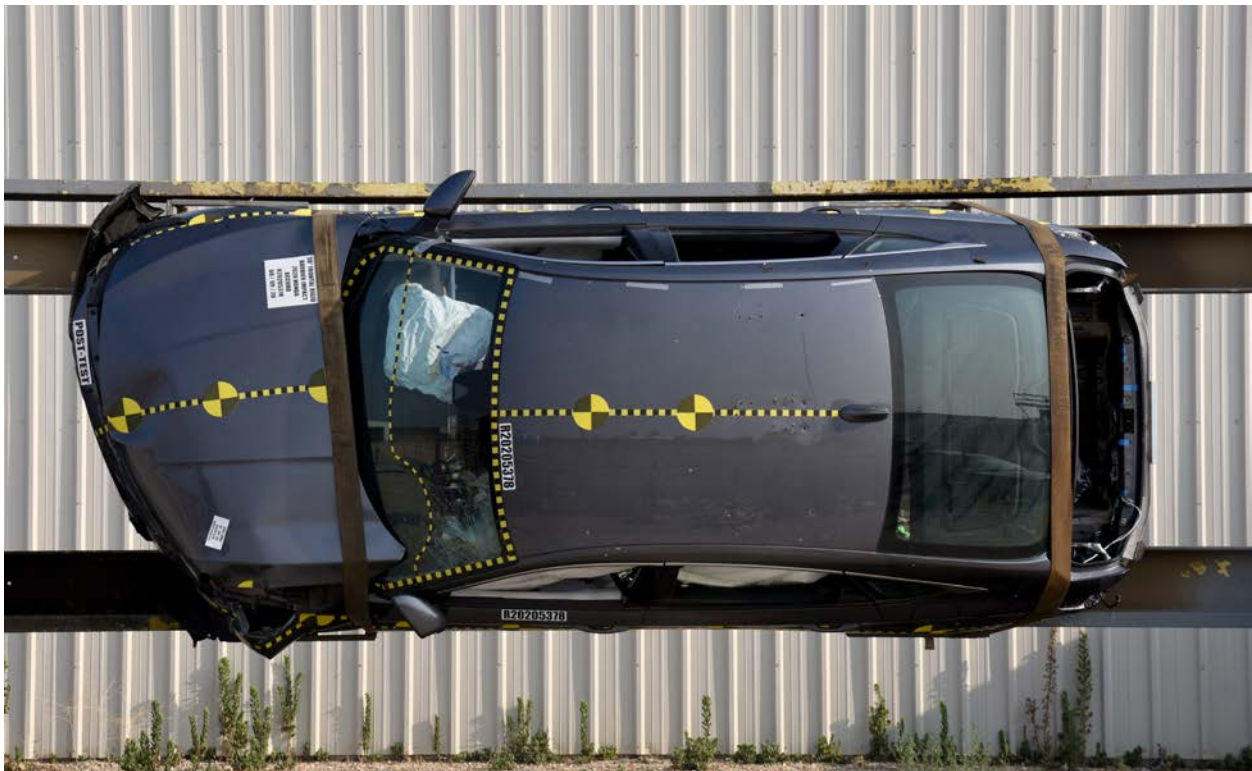
FIGURE 141. Vehicle at 90° on Static Rollover Device
