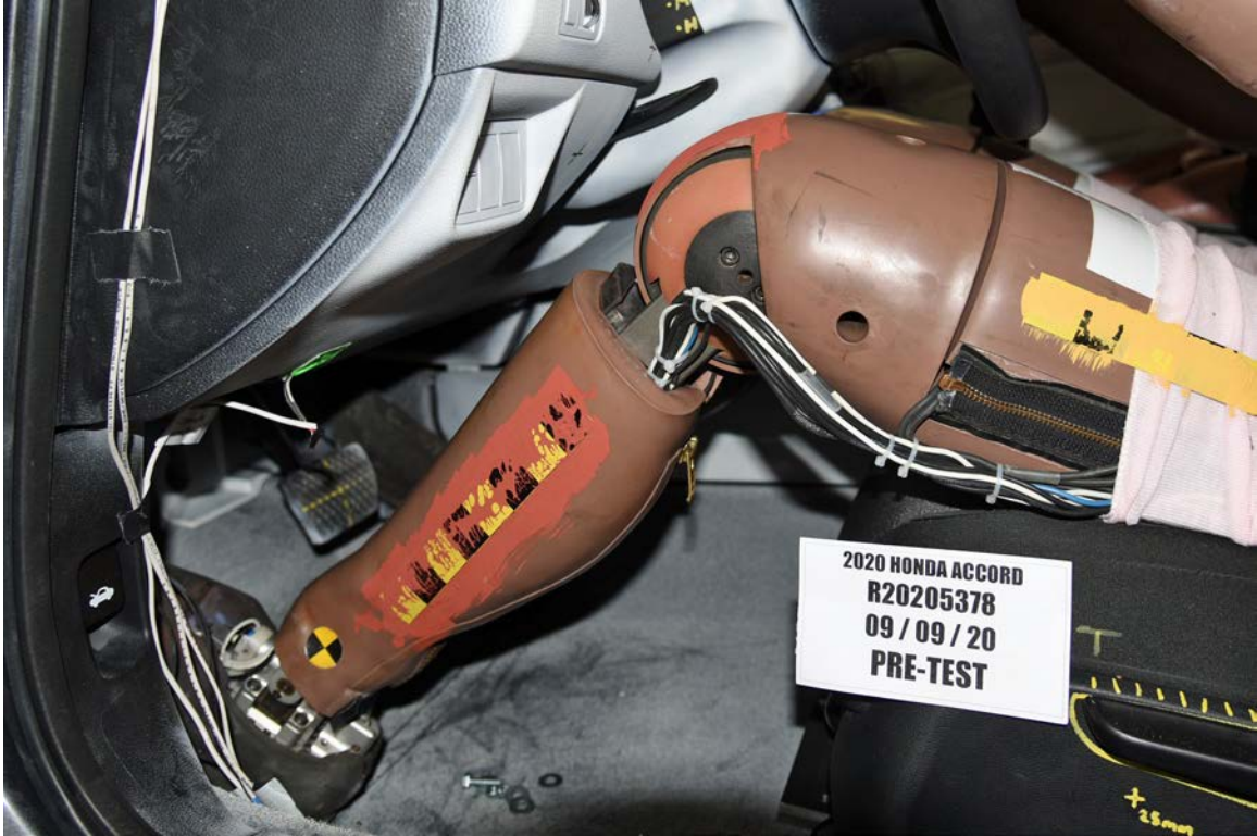
FIGURE 63. Pre-Test View of the Driver Left Leg
