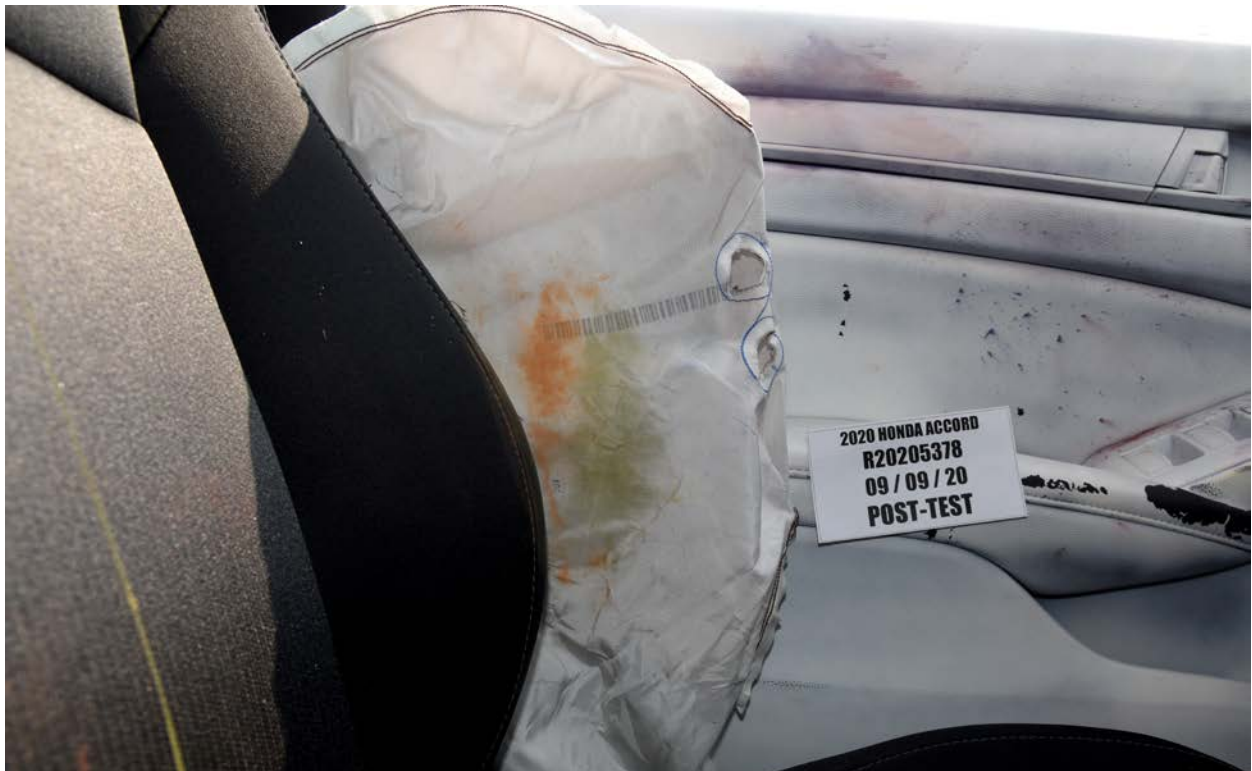
FIGURE 91a. Post-Test Driver Dummy Contact with Pelvis Airbag
