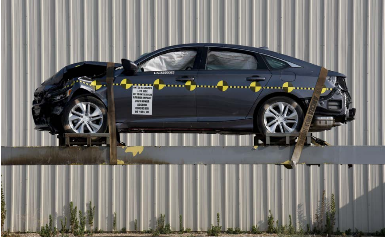
FIGURE 144. Vehicle at 360° on Static Rollover Device
