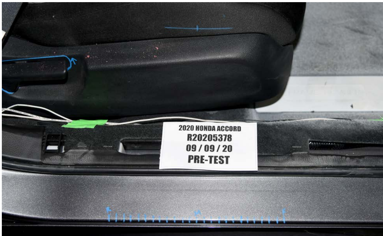
FIGURE 114. Pre-Test Right Front Passenger Seat Fore-Aft Markings
