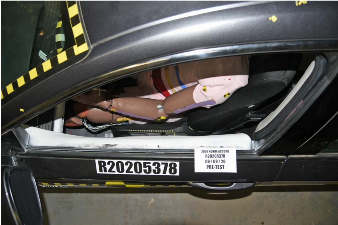
FIGURE 47. Pre-Test View of Driver Door Clearance
