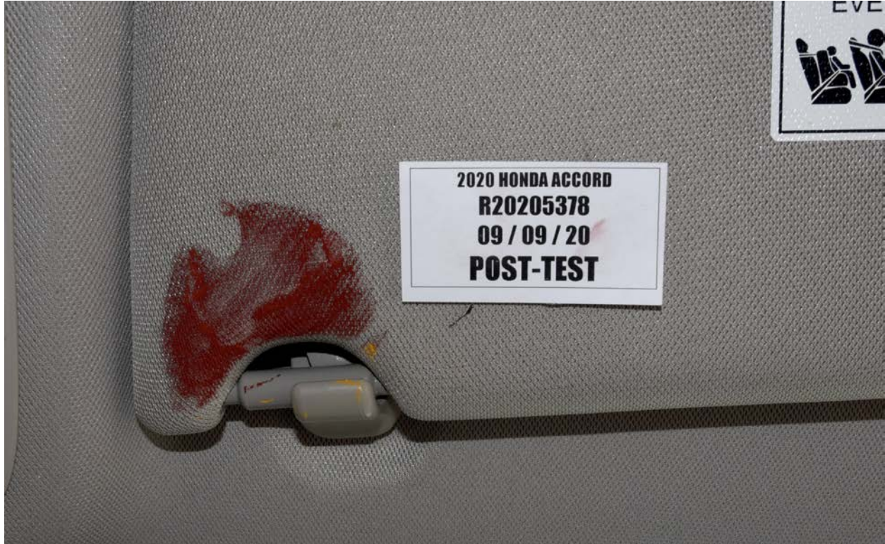
FIGURE 136a. Post-Test Driver Dummy Contact with Vehicle Interior
