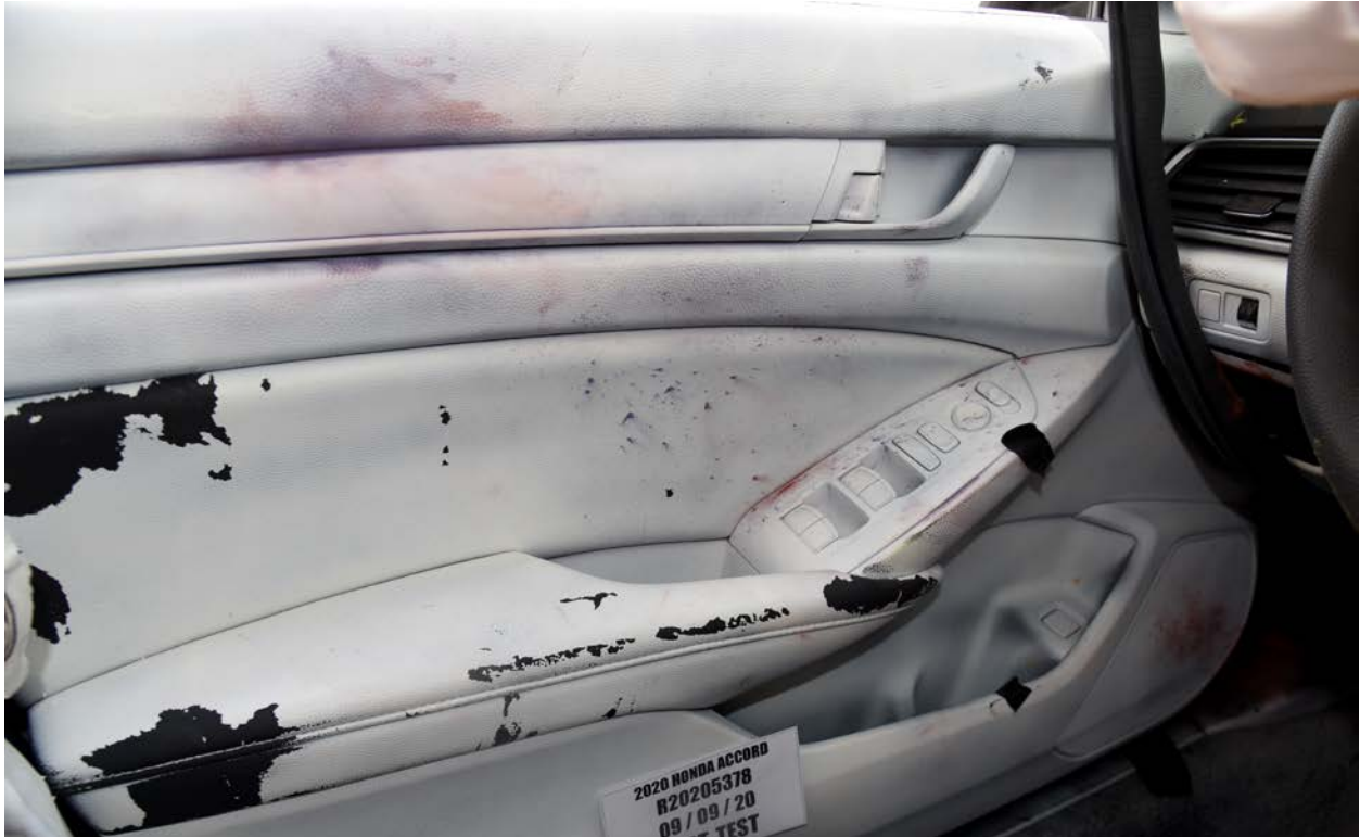
FIGURE 91f. Post-Test Driver Dummy Contact with Door Panel
