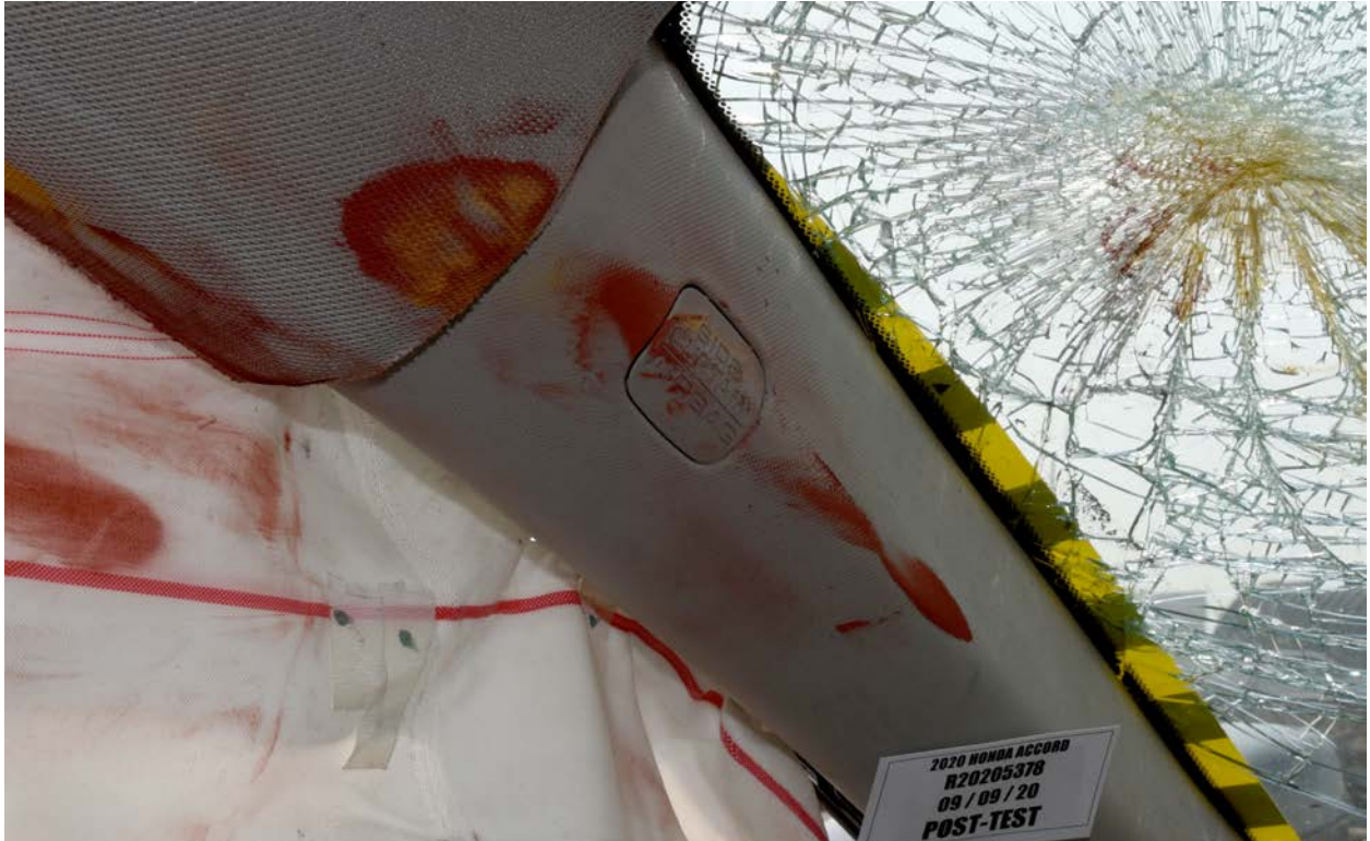
FIGURE 91b. Post-Test Driver Dummy Contact with A-Pillar
