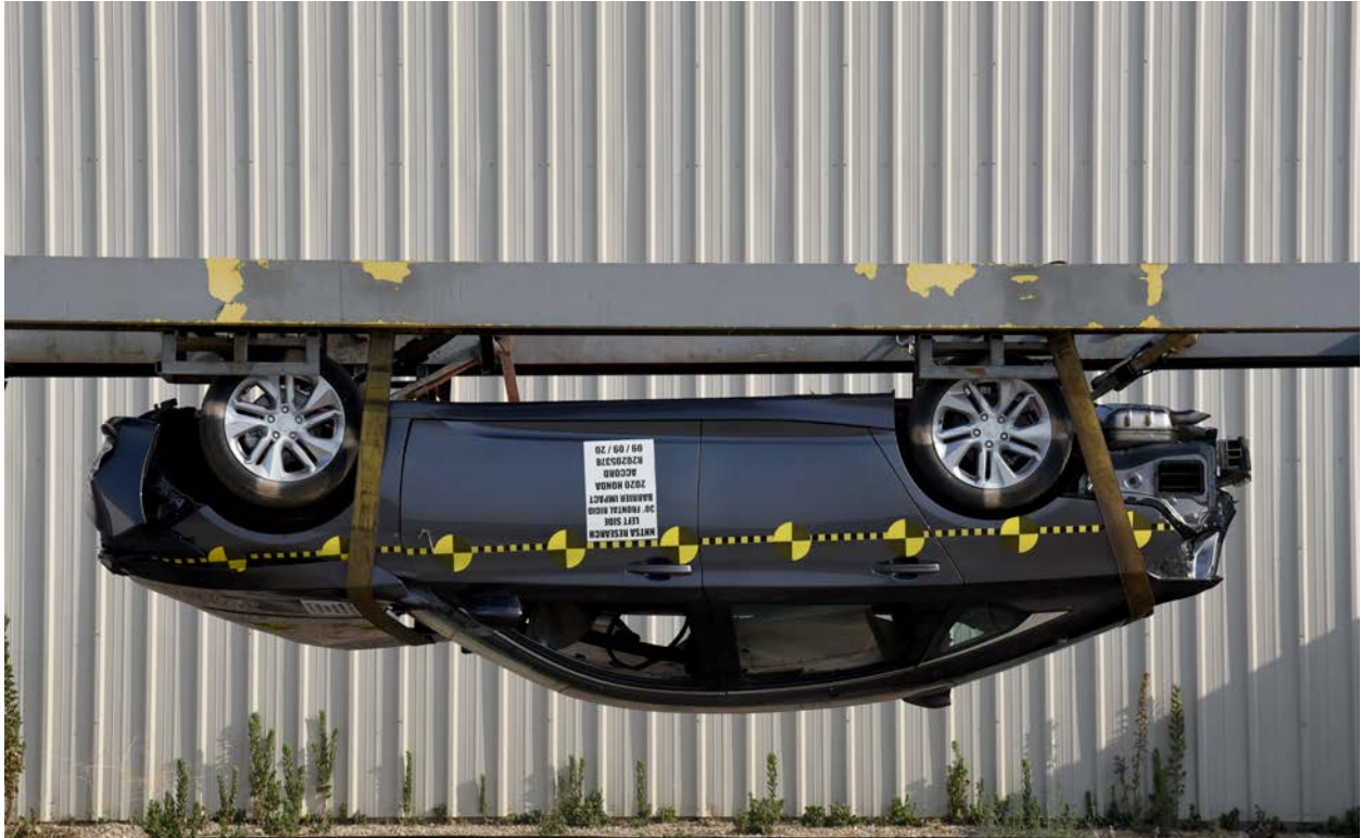
FIGURE 142. Vehicle at 180° on Static Rollover Device
