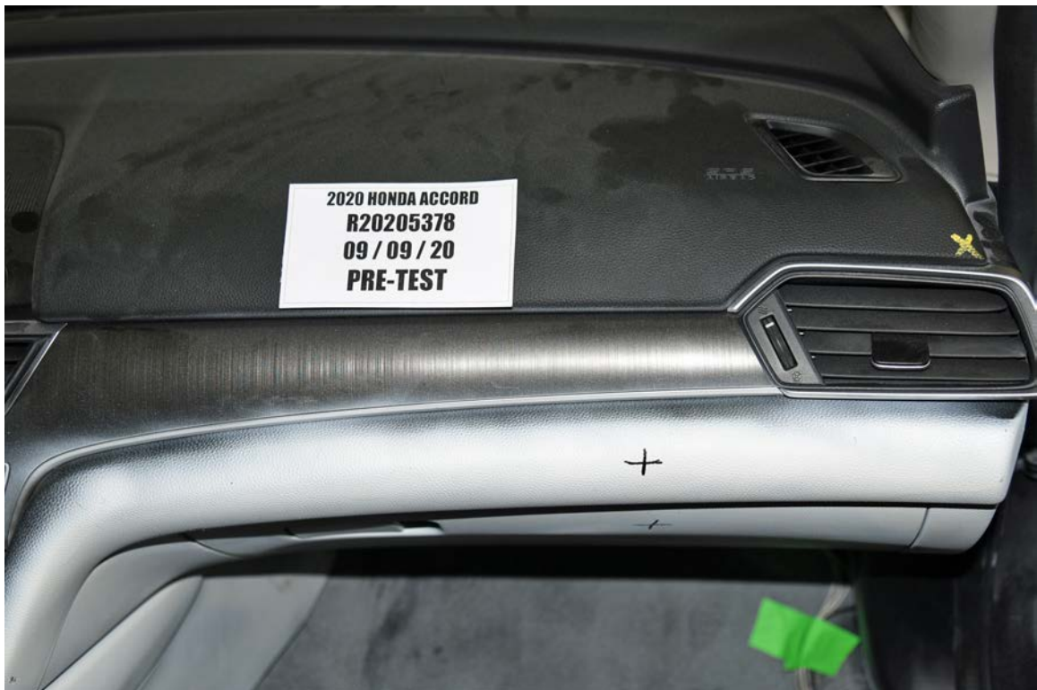
FIGURE 124. Pre-Test Center View of Passenger Knee Bolster
