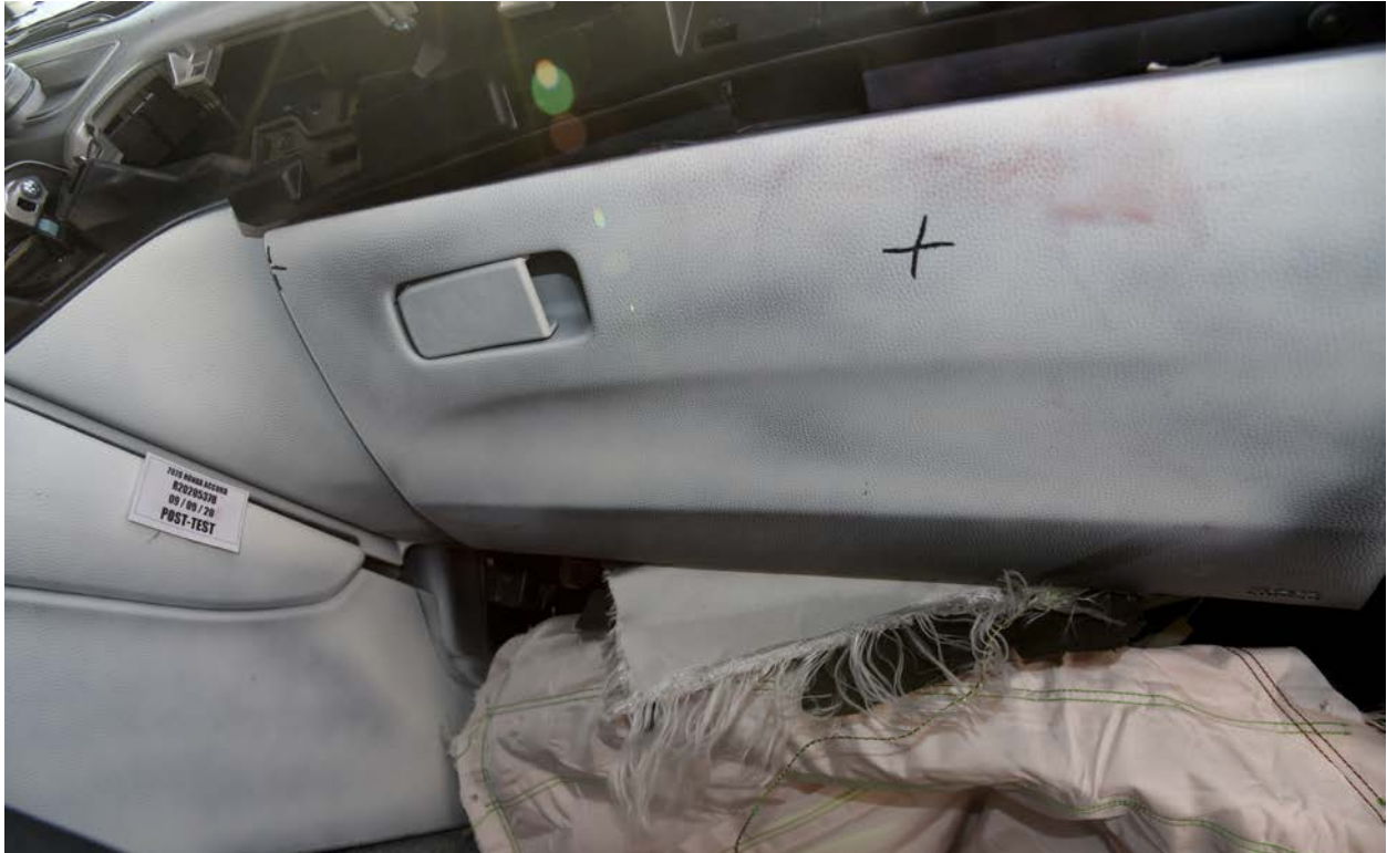
FIGURE 123. Post-Test Right Side View of Passenger Knee Bolster
