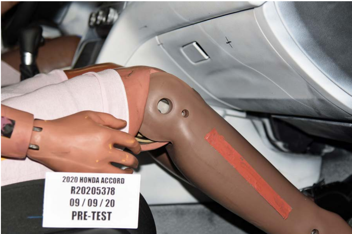
FIGURE 106. Pre-Test View of Passenger Right Knee and Bolster
