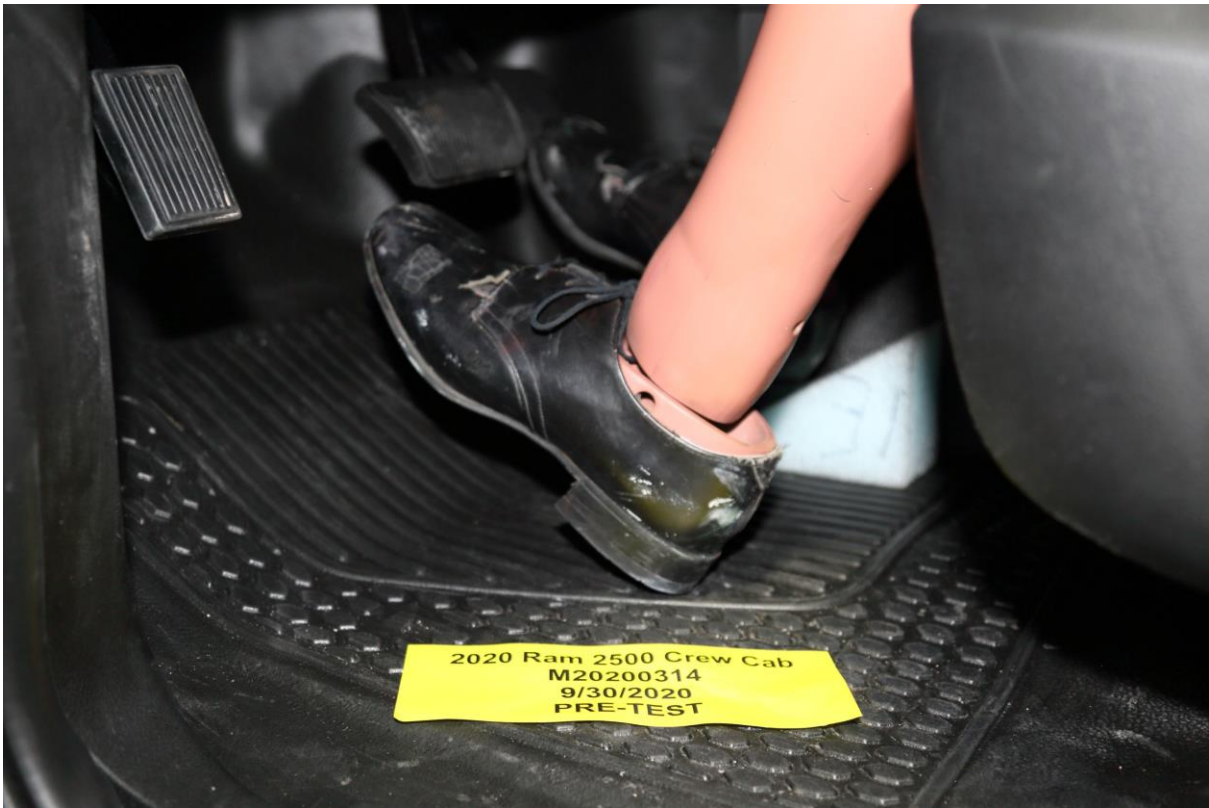
No. 032 Pre-Test Placement of Dummy Feet
