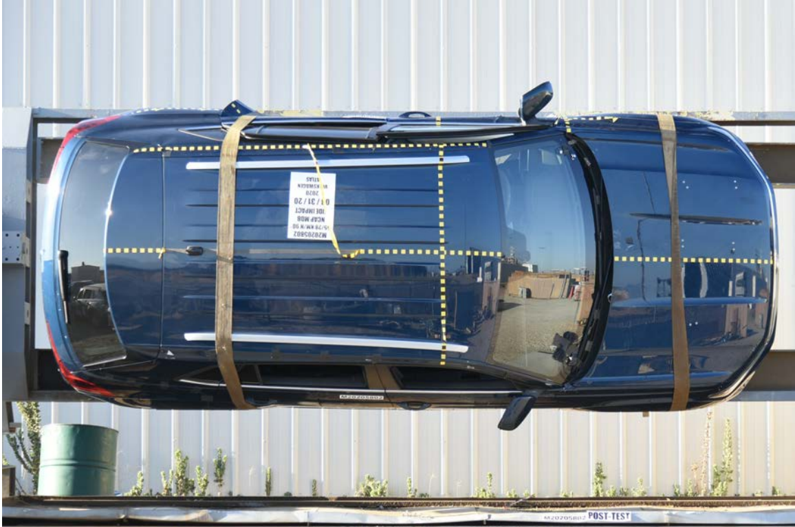
FIGURE 97. FMVSS No. 301 Static Rollover 90 Degrees
