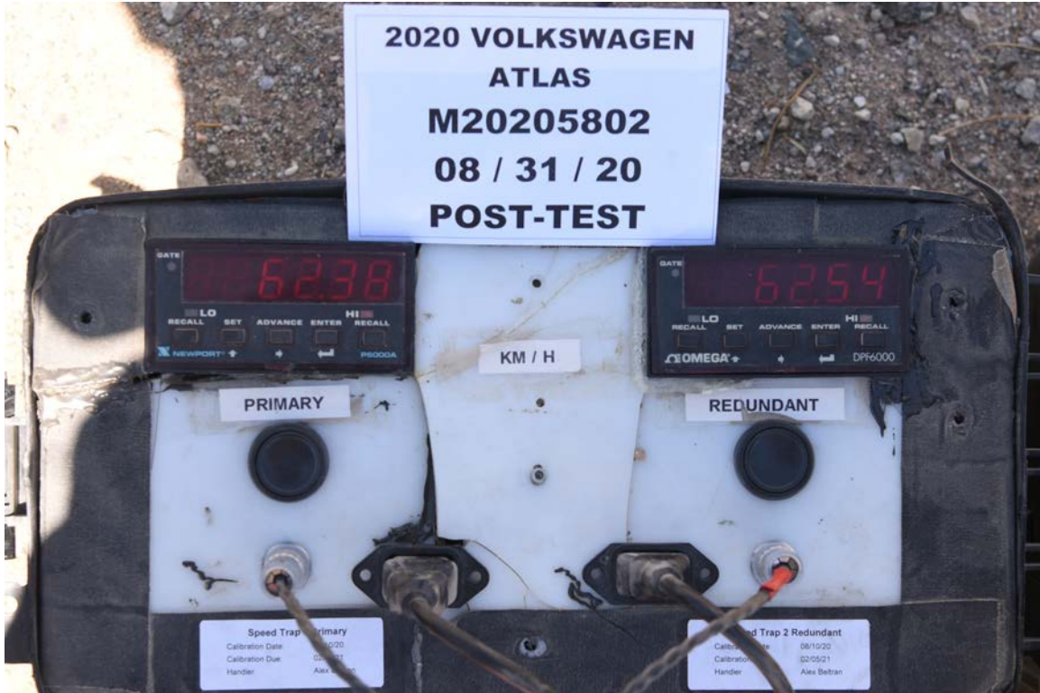
FIGURE 95. Post-Test Primary and Redundant Speed Trap Read-Out
