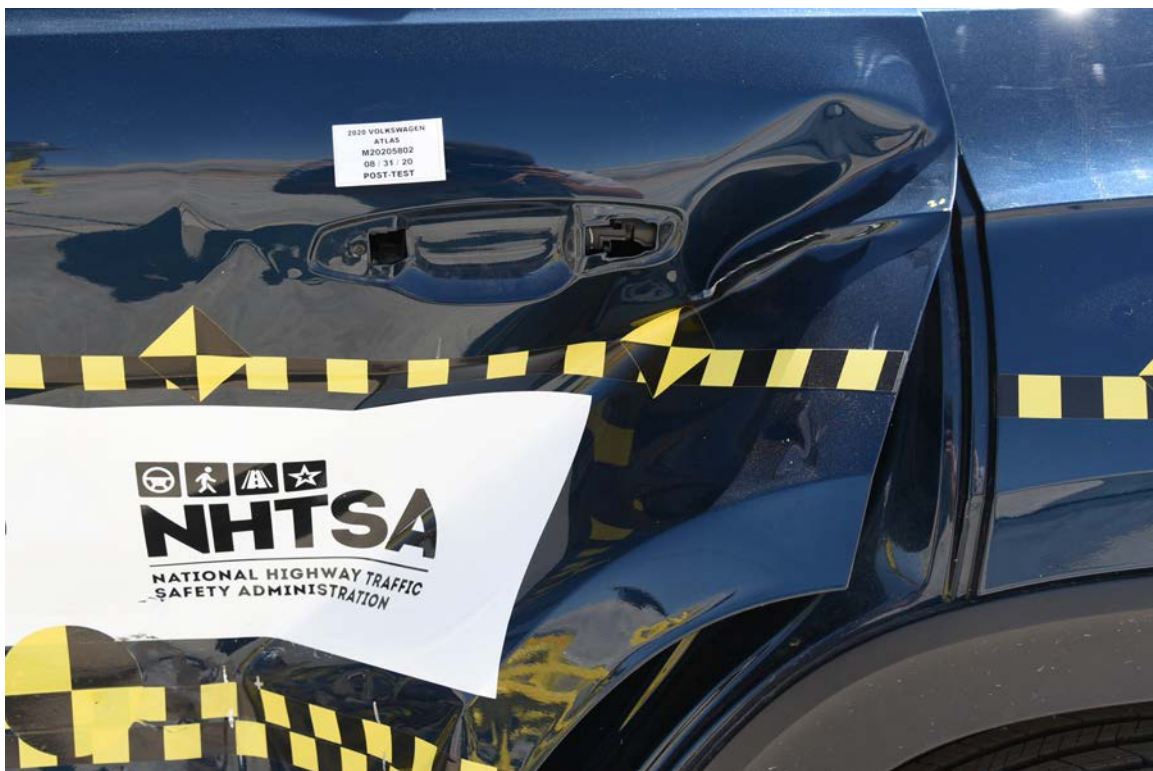
FIGURE 24. Post-Test Left Rear Door Latch Close-Up
