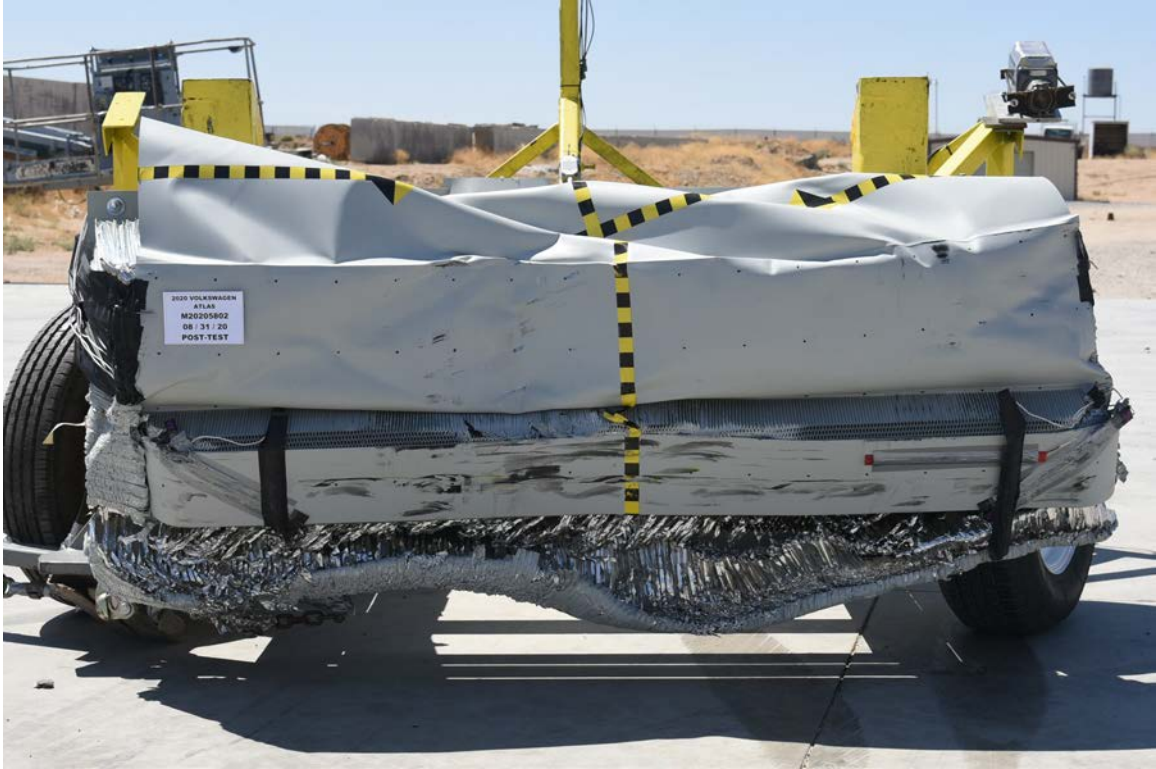
FIGURE 85. Post-Test Front View of MDB Impactor Face
