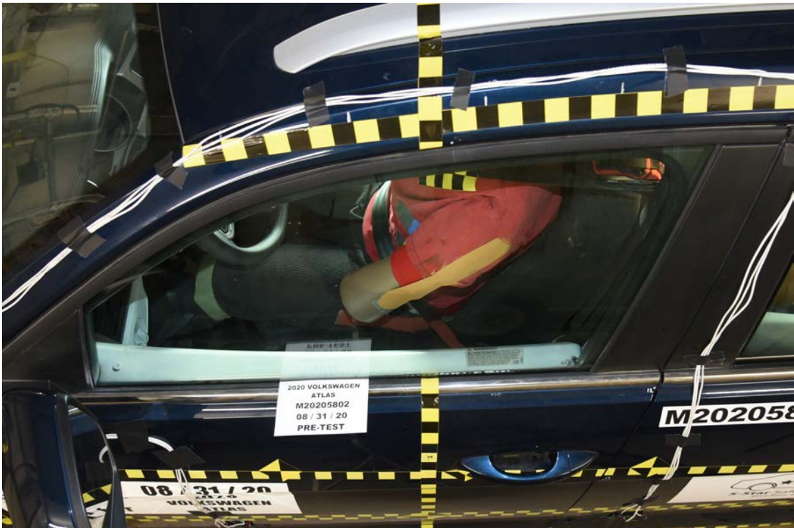
FIGURE 42. Pre-Test Driver Dummy and Door Clearance View
