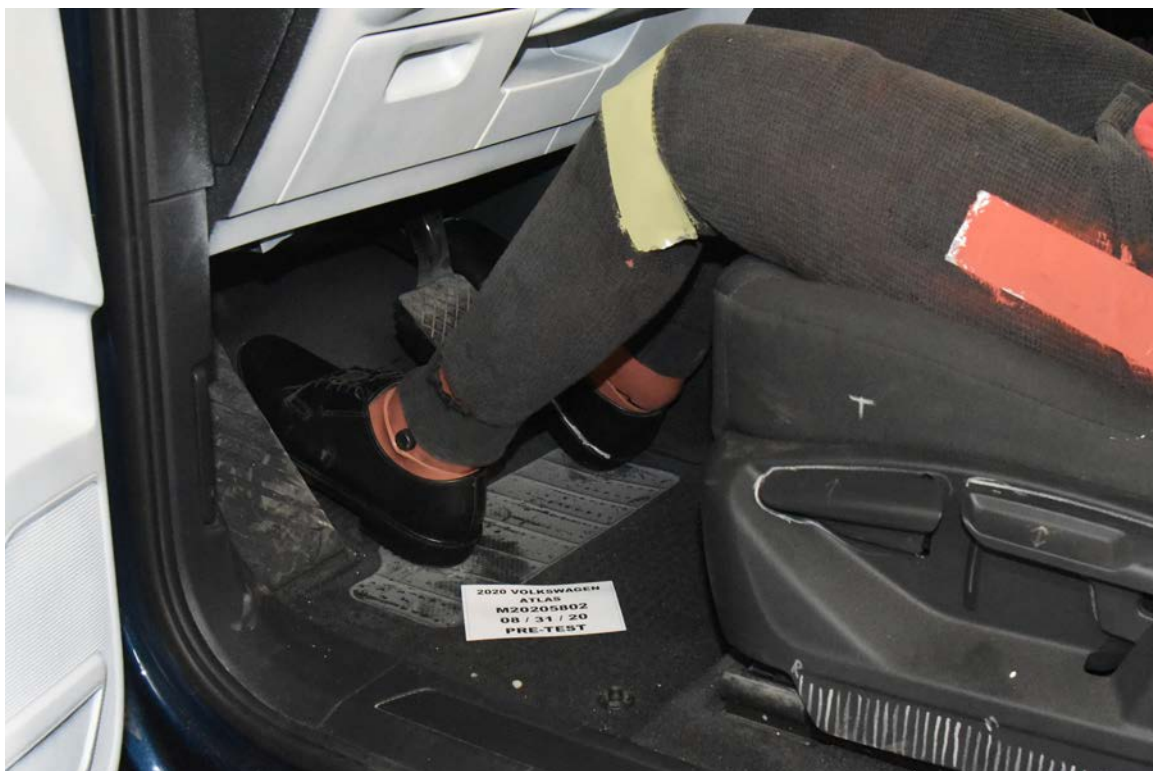
FIGURE 34. Pre-Test Placement of Driver Dummy's Feet
