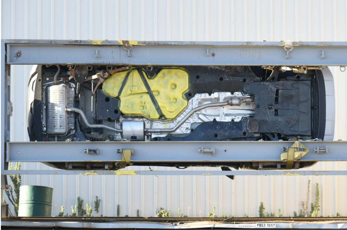
FIGURE 99. FMVSS No. 301 Static Rollover 270 Degrees
