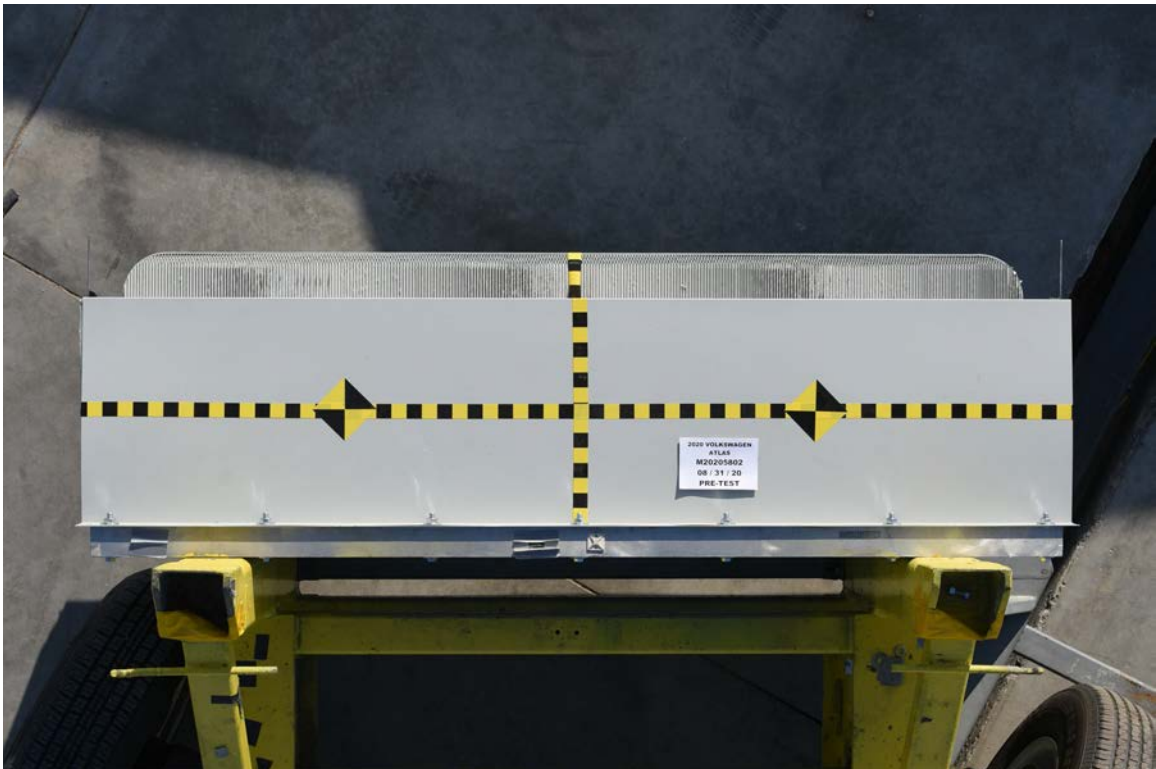
FIGURE 86. Pre-Test Top View of MDB Impactor Face
