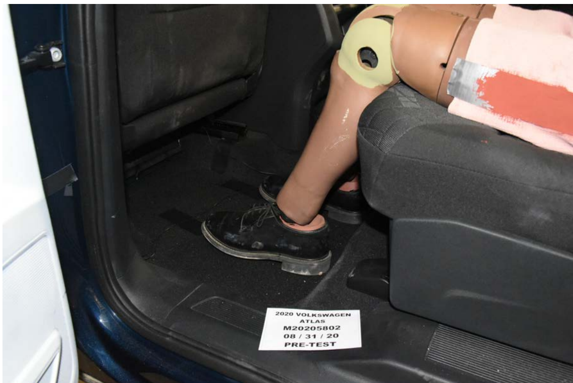
FIGURE 64. Pre-Test Placement of Rear Passenger Dummy's Feet
