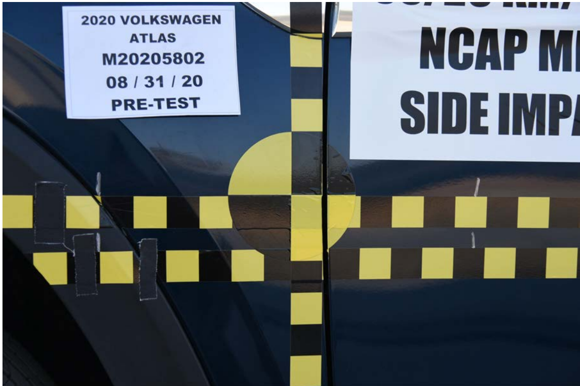
FIGURE 19. Pre-Test Close-Up View of Impact Point Target
