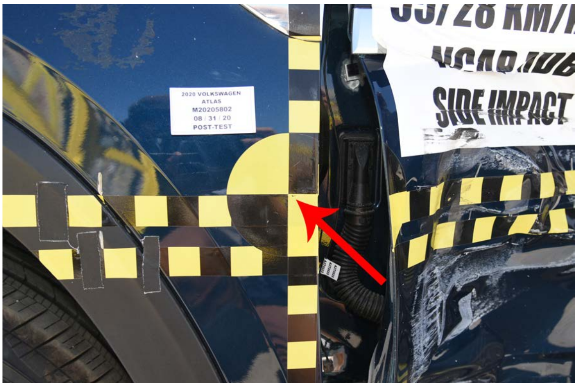
FIGURE 20. Post-Test Close-Up View of Impact Point Target
