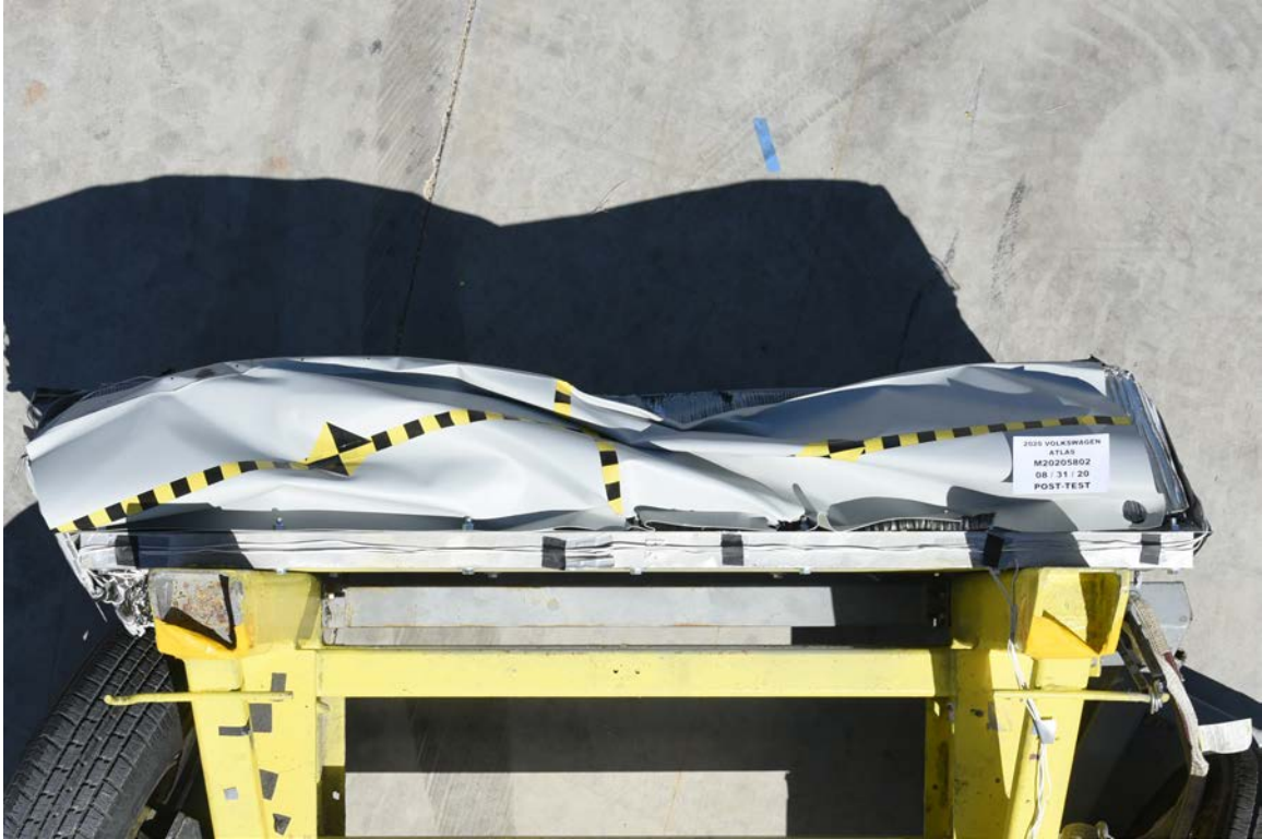
FIGURE 87. Post-Test Top View of MDB Impactor Face
