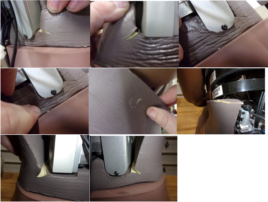
Broken Grounding Strap which connects the Pelvis to the Thorax.
