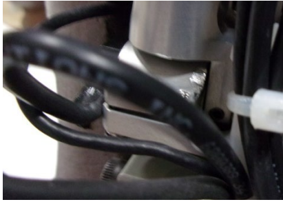
Damage done all along the Posterior Inferior edge of the shoulder covers.
