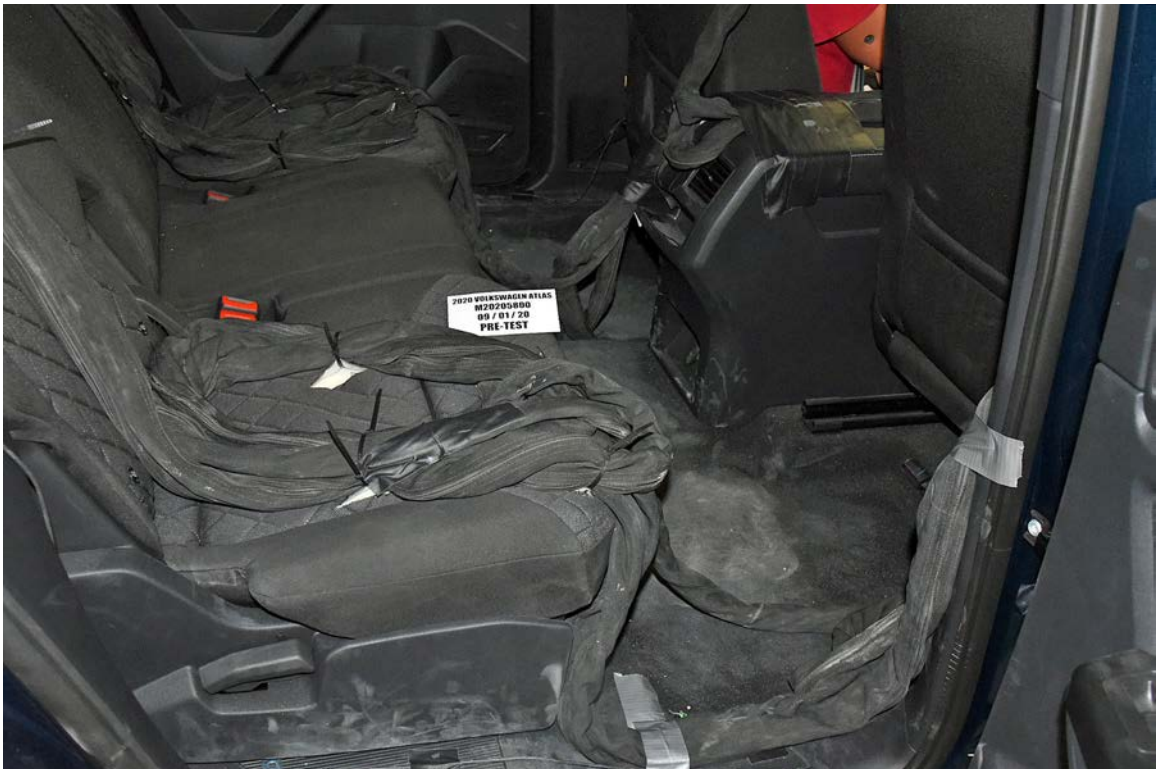
FIGURE 28. Pre-Test Dummy Cable Routing
