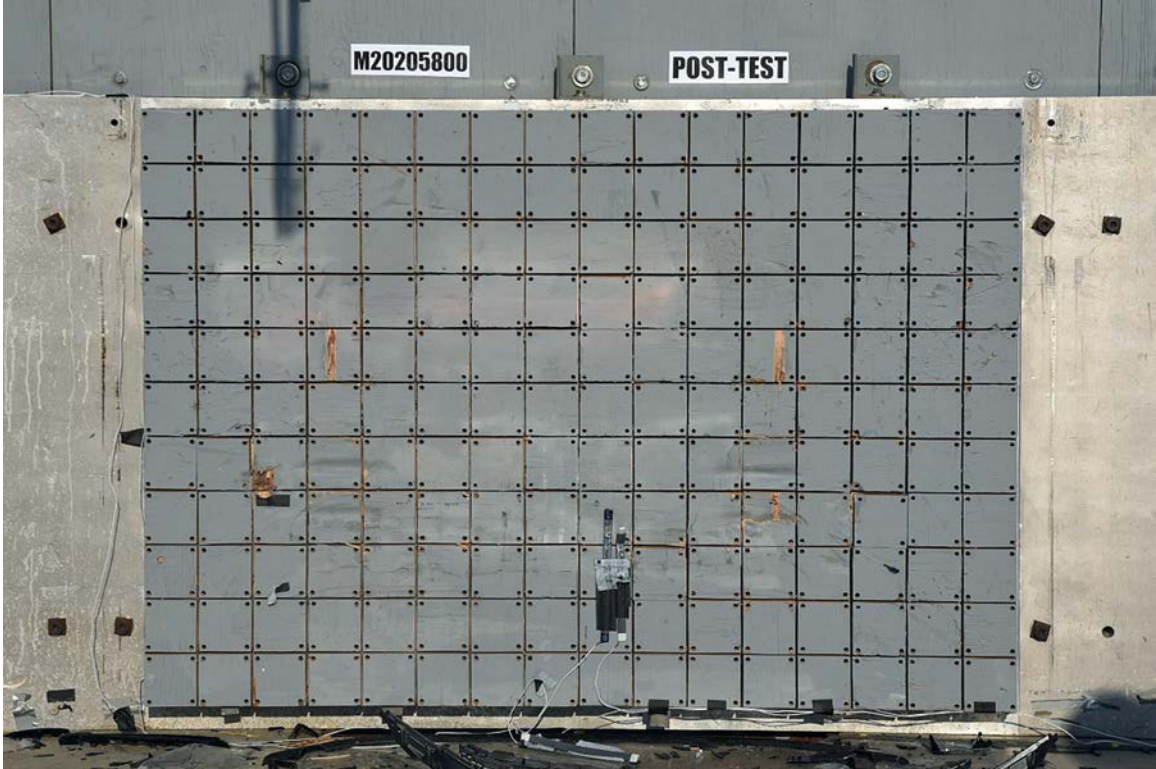
FIGURE 3. Post-Test Load Cell Wall
