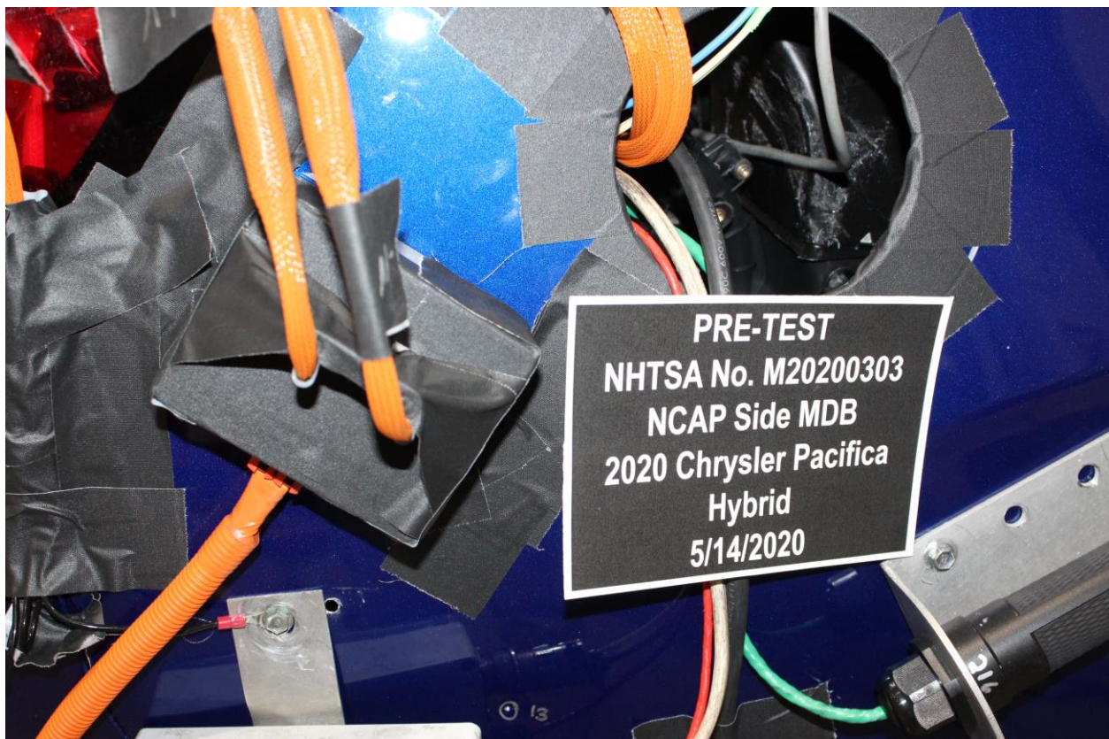
Figure 305-24: Pre-Impact View of Installed Test Interface Port
