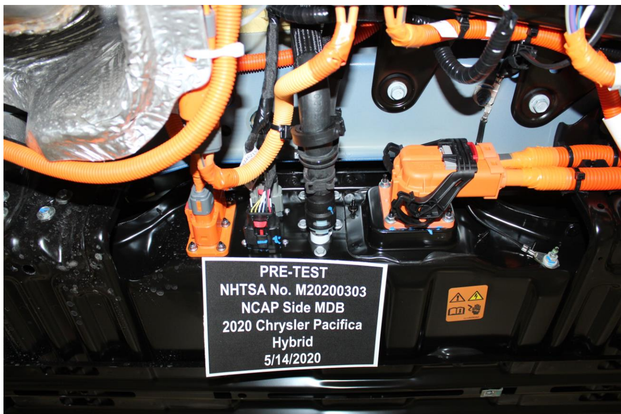
Figure 305-22: Pre-Impact View of High Voltage Leads Attached
