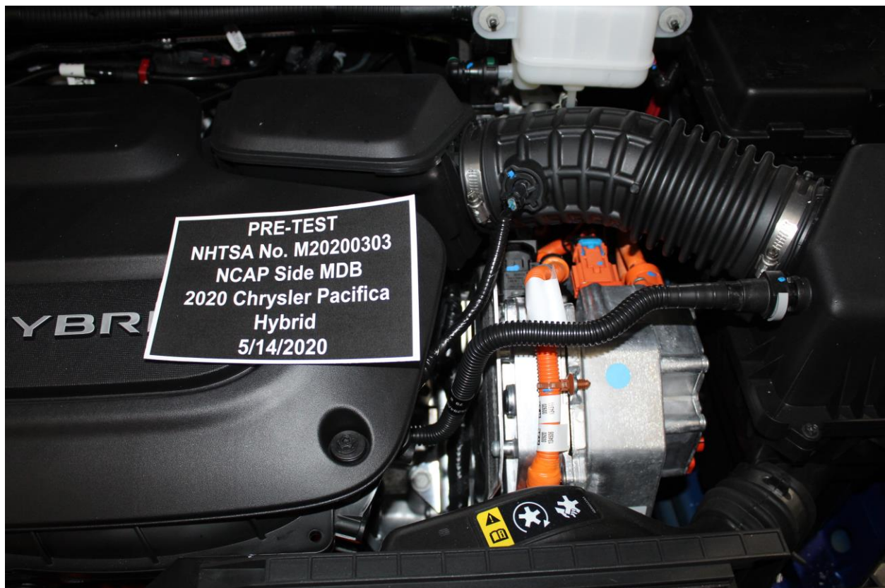
Figure 305-16: Pre-Impact View of Electric Propulsion Drive
