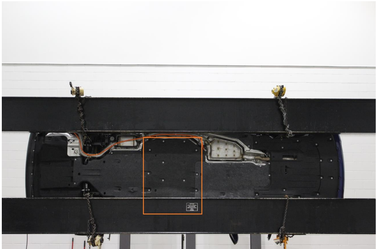
Figure 305-28: FMVSS No. 305 Static Rollover 90 Degrees
