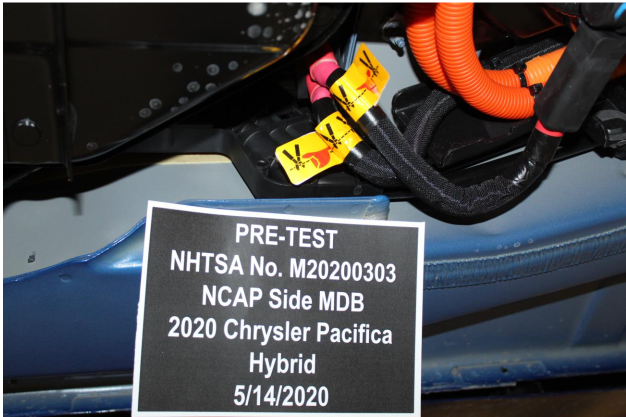
Figure 305-3 First Responder Warning Label
