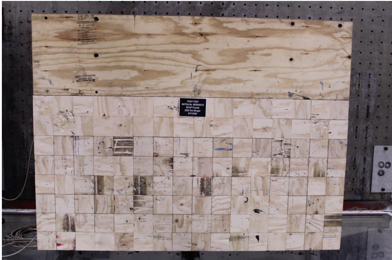
Figure A-3: Post-Test Load Cell Wall
