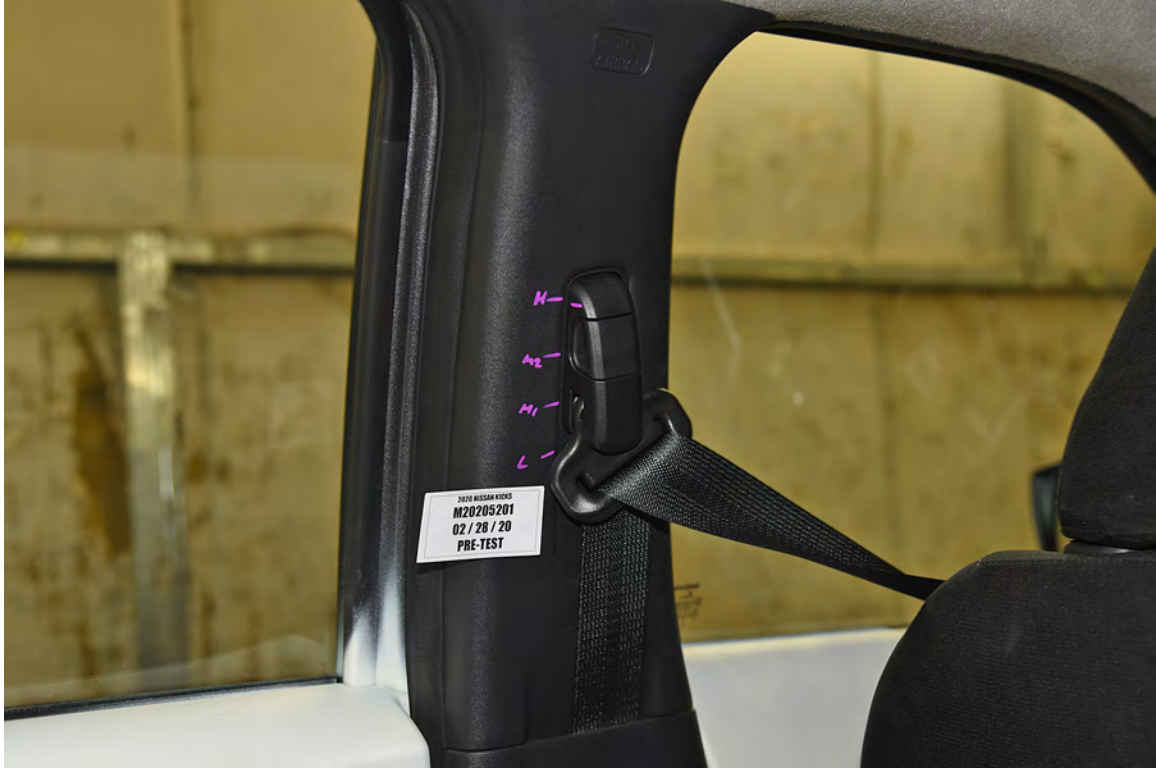
FIGURE 33. Pre-Test View of Belt Anchorage for Dummy
