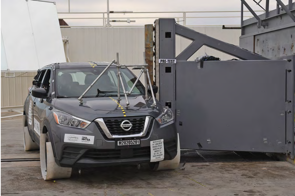
FIGURE 17. Pre-Test Left Side View of Pole Positioned Against Side of Vehicle
