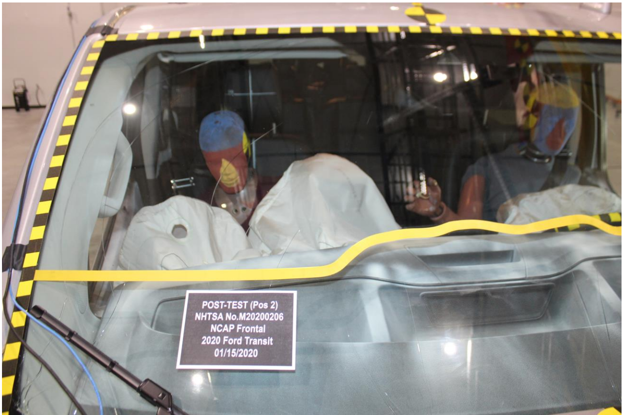
Figure A-54: Post-Test Passenger Dummy Front View
