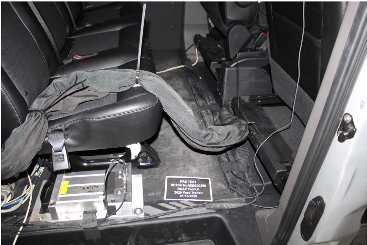
Figure A-28: Pre-Test Dummy Cable Routing
