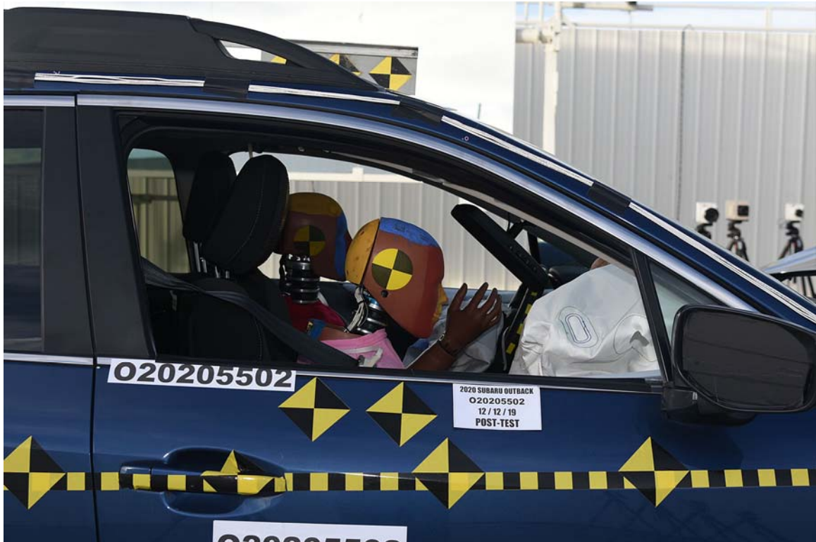
FIGURE 56. Post-Test Passenger Dummy Window View
