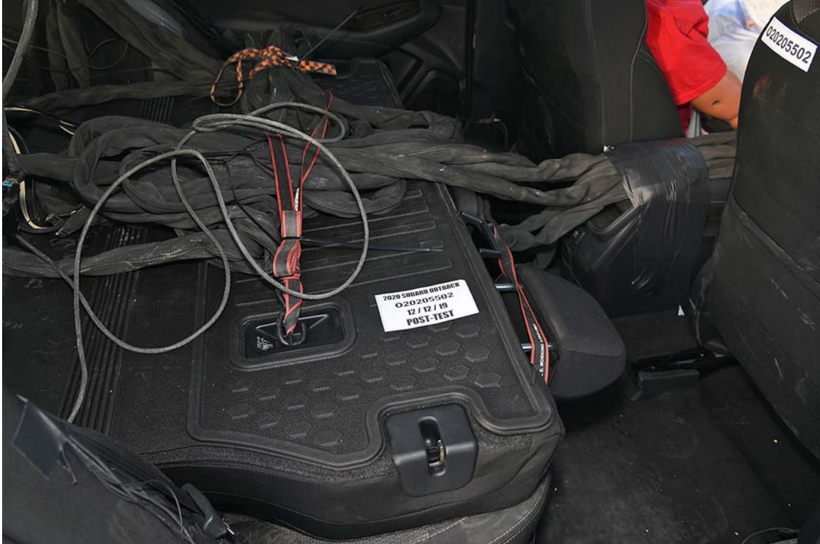
FIGURE 29. Post-Test Dummy Cable Routing
