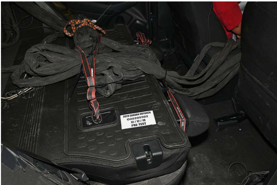
FIGURE 28. Pre-Test Dummy Cable Routing
