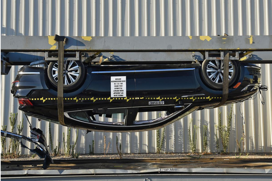
FIGURE 29. Test Vehicle at 180° on FMVSS 301 Static Rollover Device
