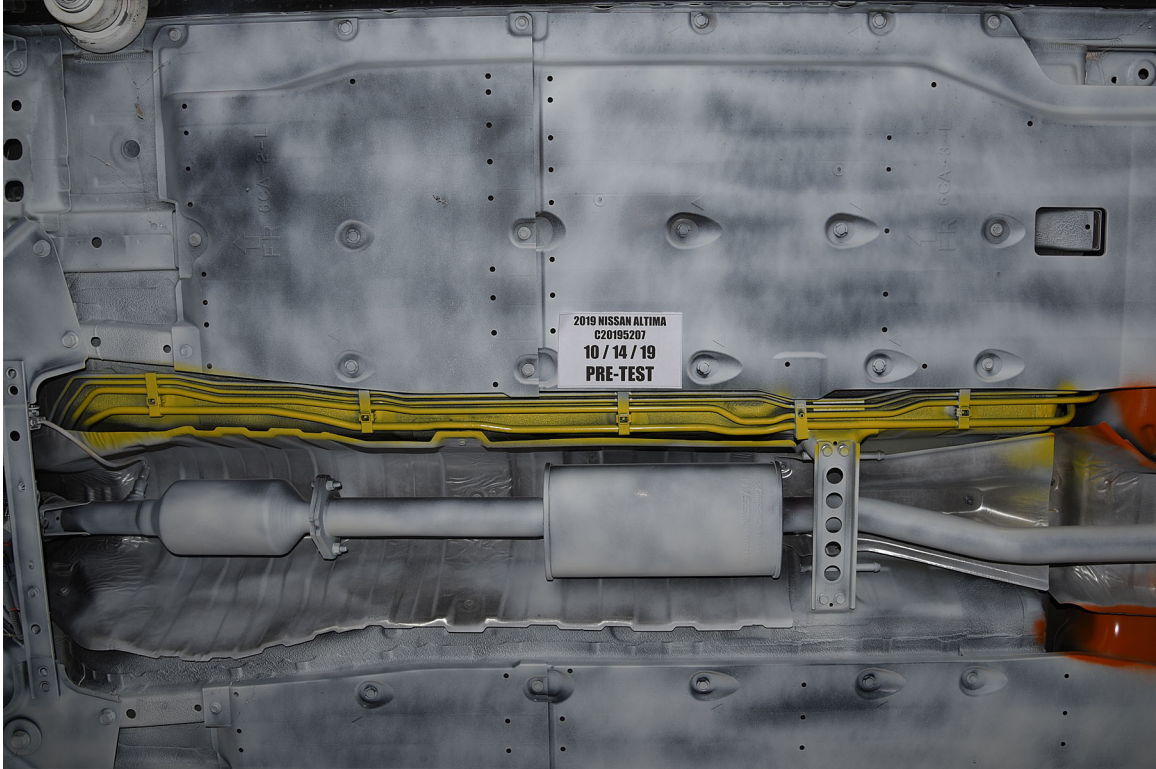
FIGURE 29. Pre-Test Underbody View of Fuel Lines
