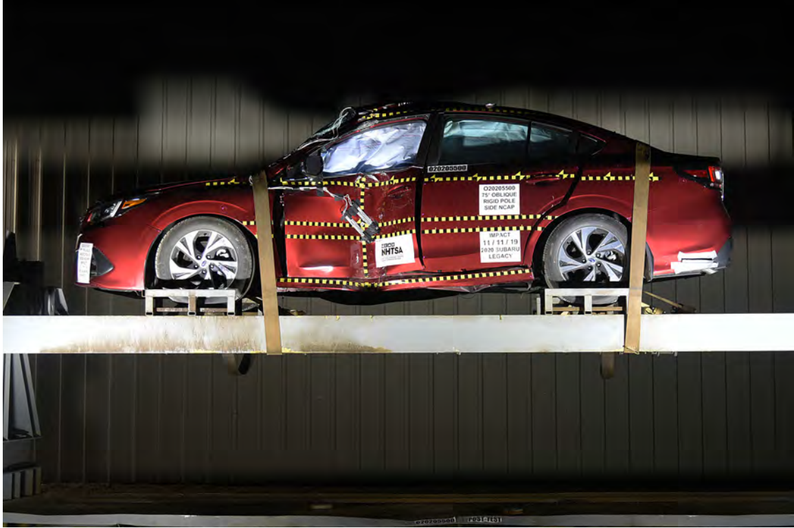
FIGURE 63. FMVSS No. 301 Static Rollover 0 Degrees
