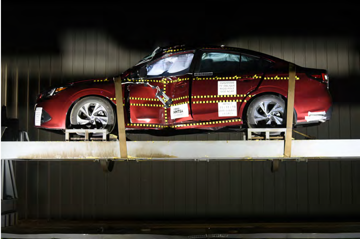
FIGURE 67. FMVSS No. 301 Static Rollover 360 Degrees
