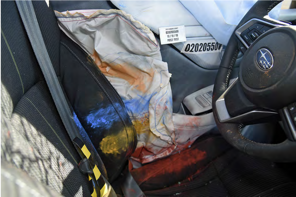
FIGURE 49. Post-Test Dummy Close-Up Torso Contact With Side Airbag View
