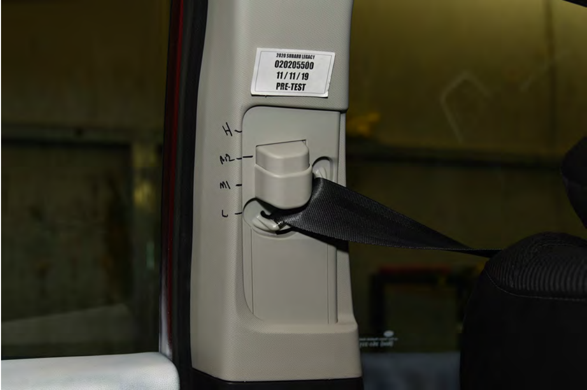
FIGURE 33. Pre-Test View of Belt Anchorage for Dummy
