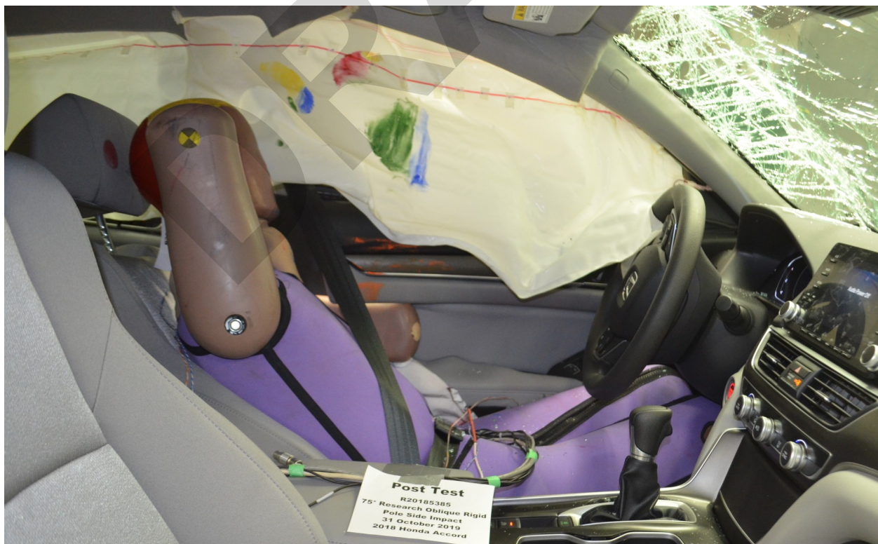
Figure A-42 Post-Test Right Side View of Dummy and Front Seat of Occupant Compartment
