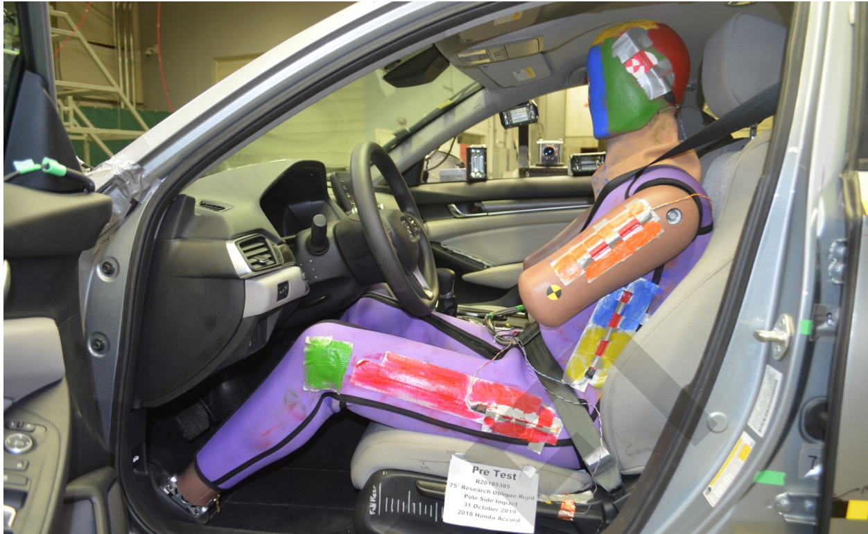
Figure A-23 Pre-Test Left Side View of Dummy Showing Belt and Chalking
