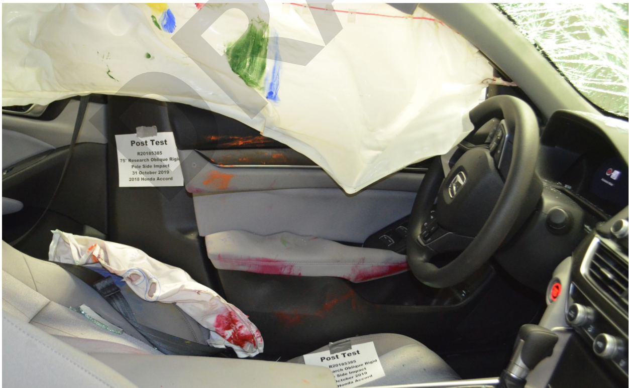
Figure A-44 Post-Test Inner Door Panel View
