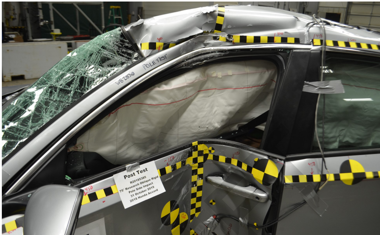
Figure A-25 Post-Test Left Side View of Dummy Shoulder and Door Top View View
