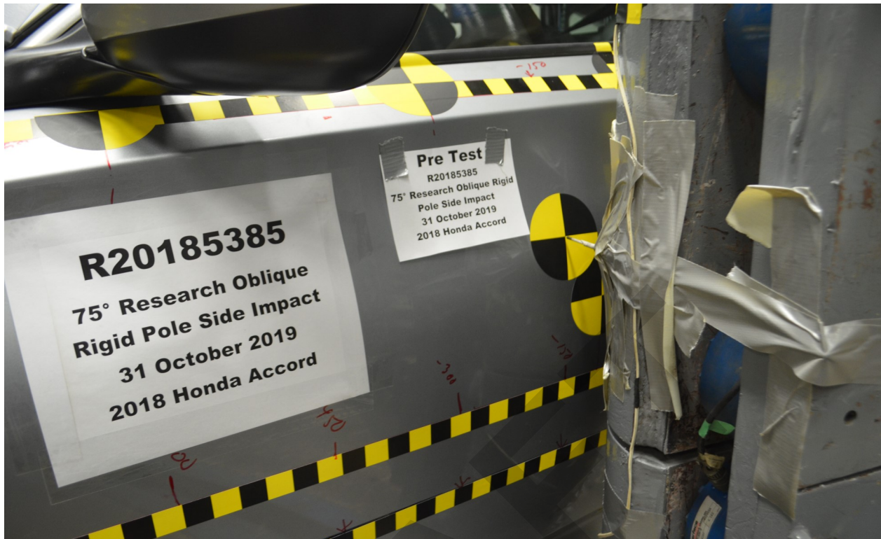
Figure A-17 Pre-Test Left Side View of Pole Positioned Against Side of Vehicle
