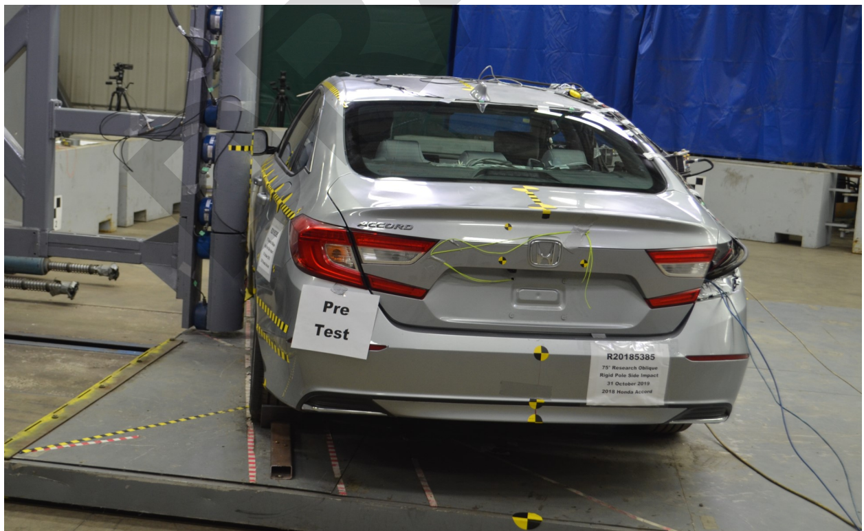
Figure A-18 Pre-Test Right Side View of Pole Positioned Against Side of Vehicle
