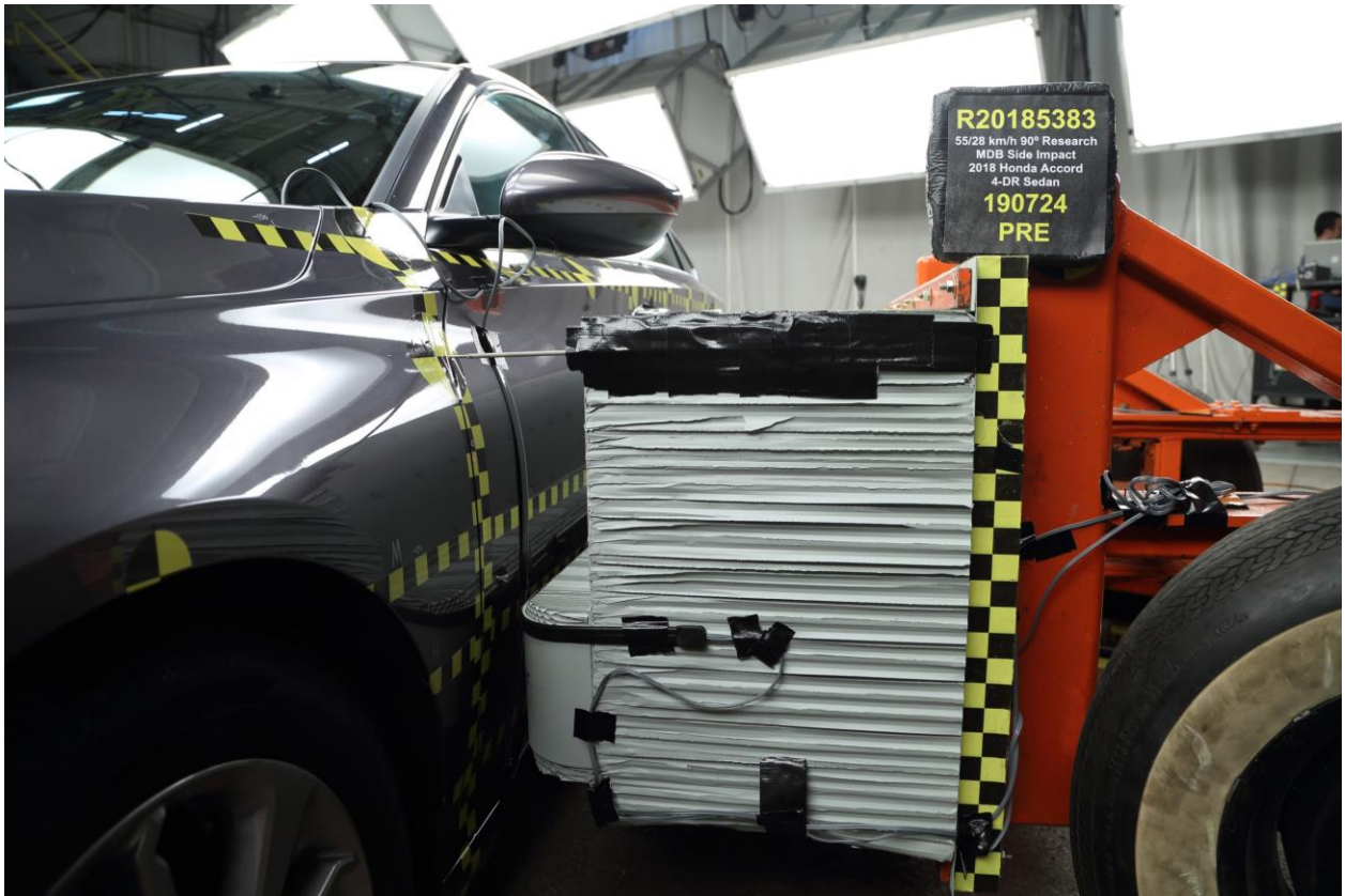
017 Pre-Test Left Side View of MDB Positioned Against Side of Test Vehicle
