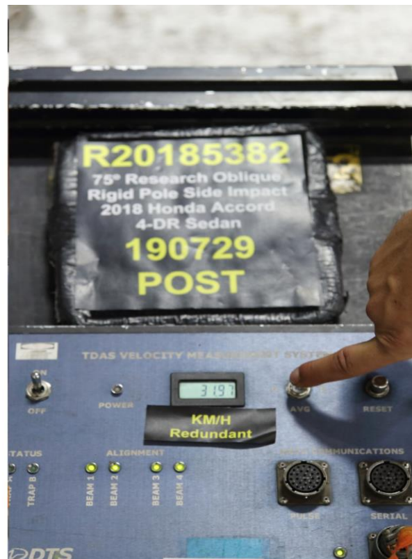
No. 063 Post-Test Primary and Redundant Speed Trap Read Out
