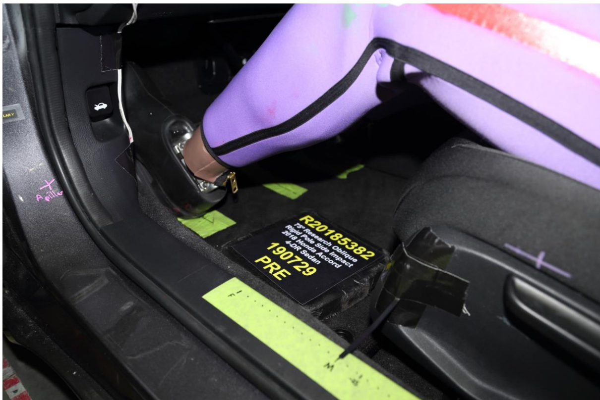
No. 032 Pre-Test Placement of Dummy Feet
