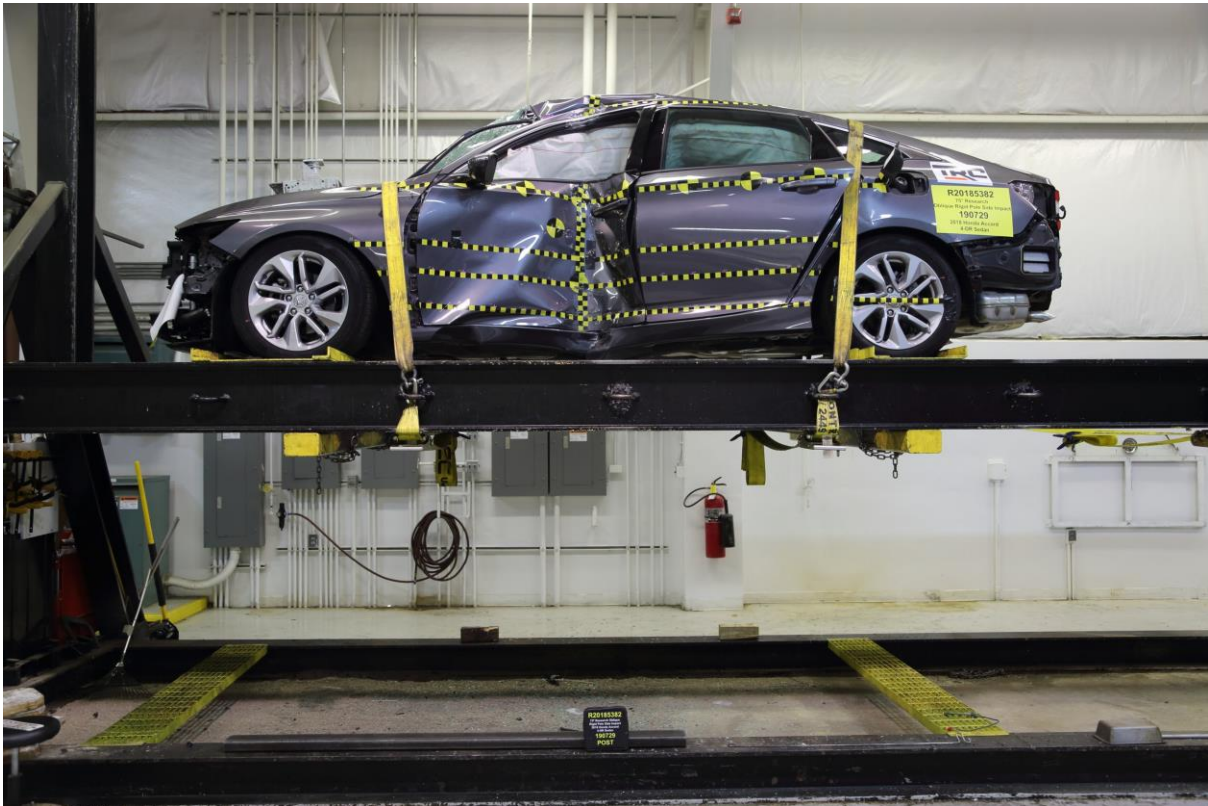
No. 068 FMVSS No. 301 Static Rollover 360 Degrees
