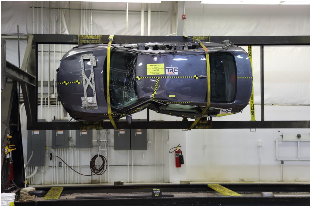
No. 065 FMVSS No. 301 Static Rollover 90 Degrees
