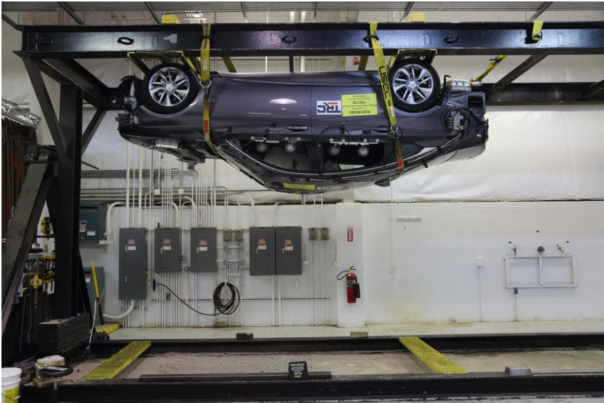
No. 066 FMVSS No. 301 Static Rollover 180 Degrees
