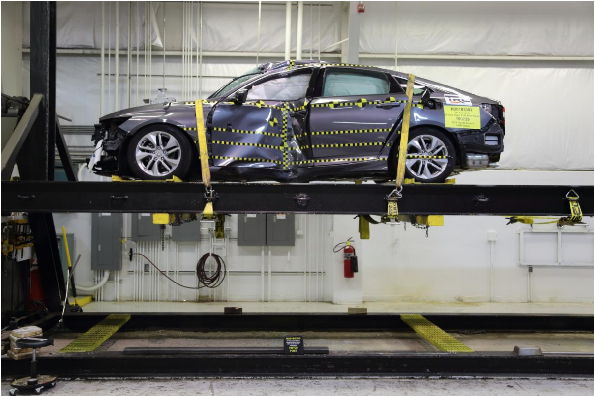
No. 064 FMVSS No. 301 Static Rollover 0 Degrees
