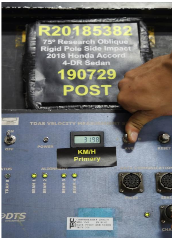
No. 063 Post-Test Primary and Redundant Speed Trap Read Out
