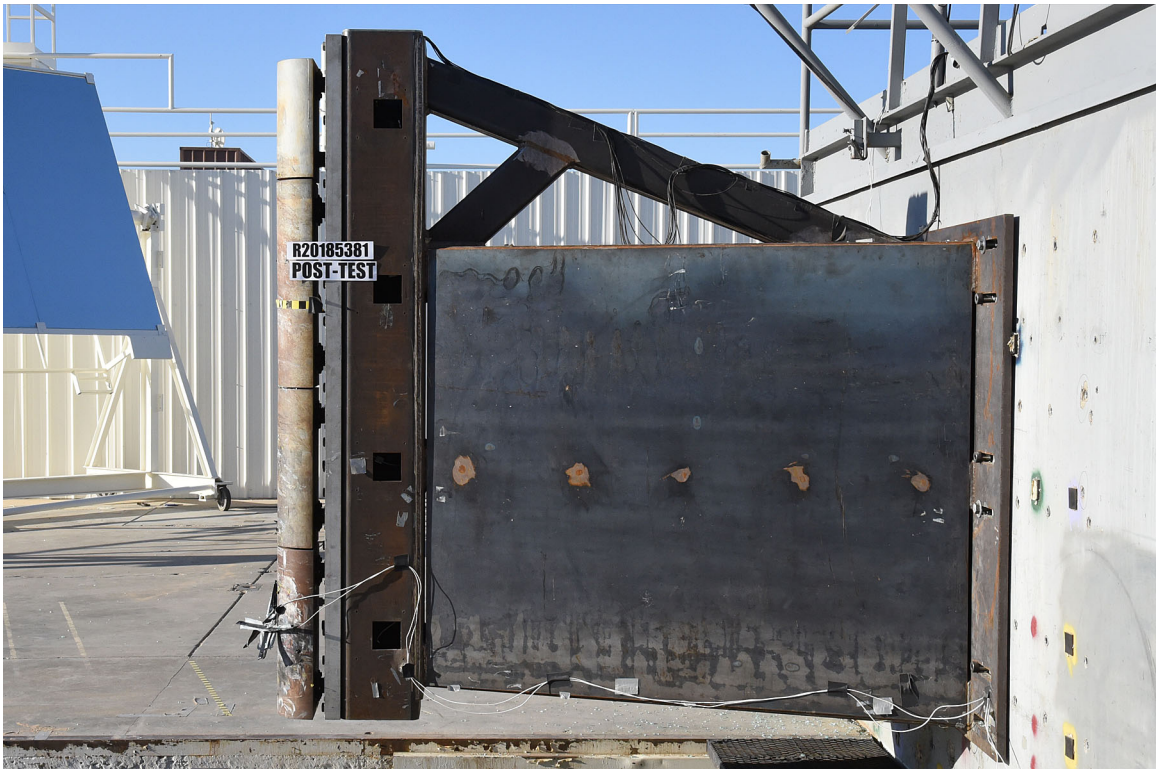
FIGURE 60. Post-Test Pole Barrier Side View
