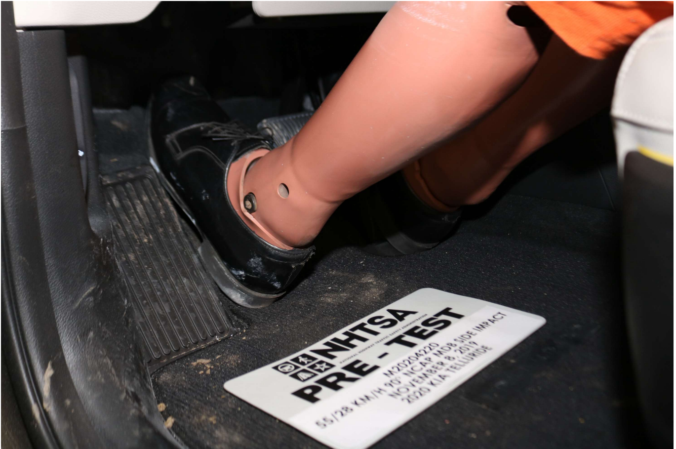
Photo No. 034 - Pre-Test Placement of Driver Dummy Feet
