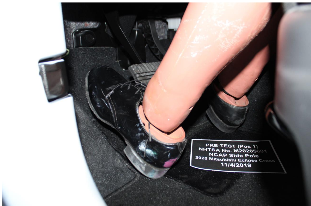
Figure A-32: Pre-Test Placement of Dummy's Feet
