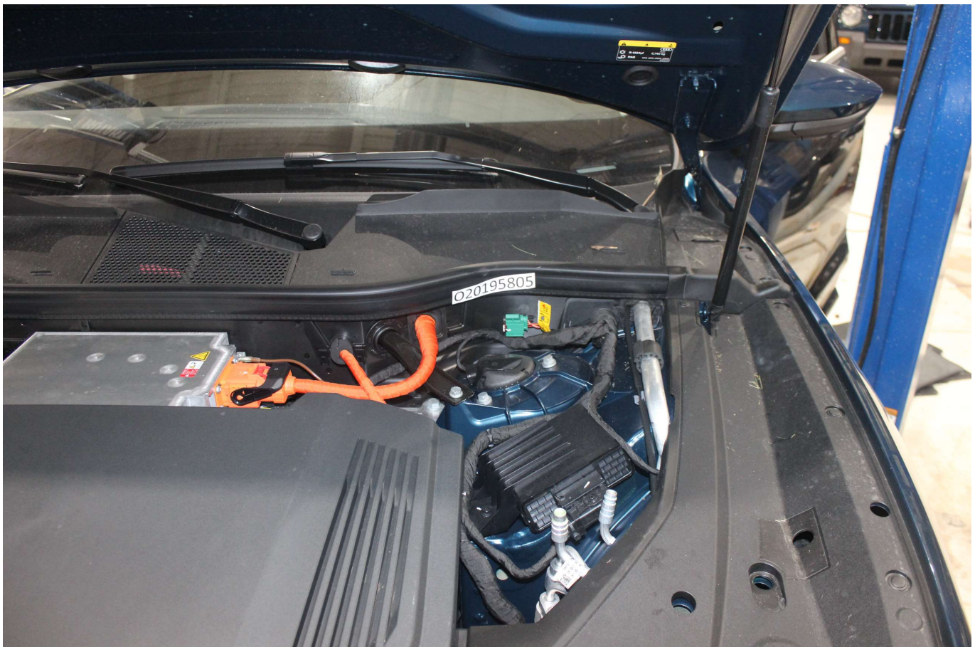
Photo No. 004 - First Responder Warning Location
