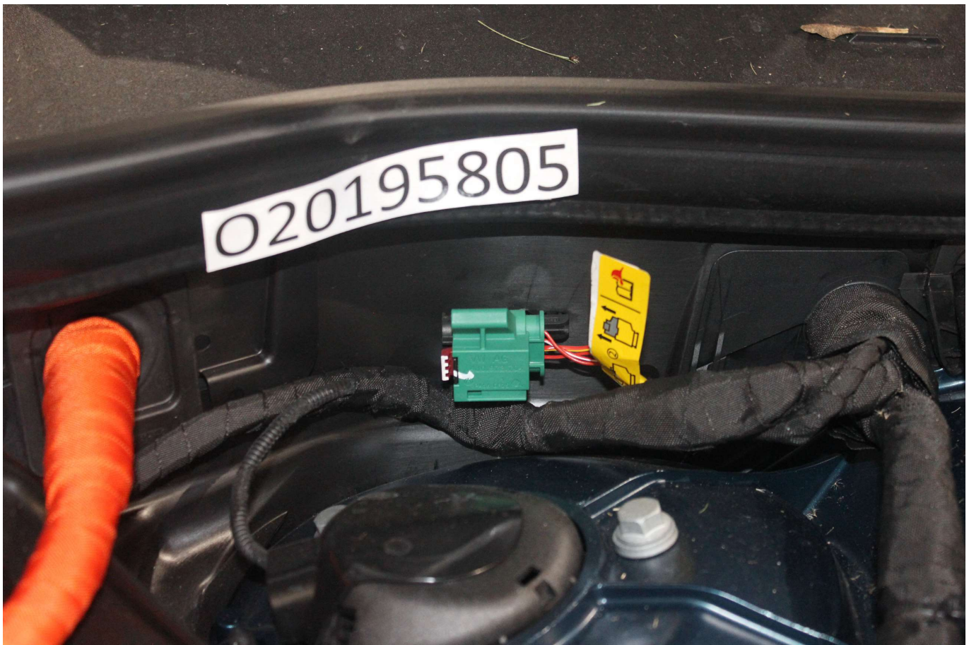
Photo No. 003 - First Responder Warning Label
