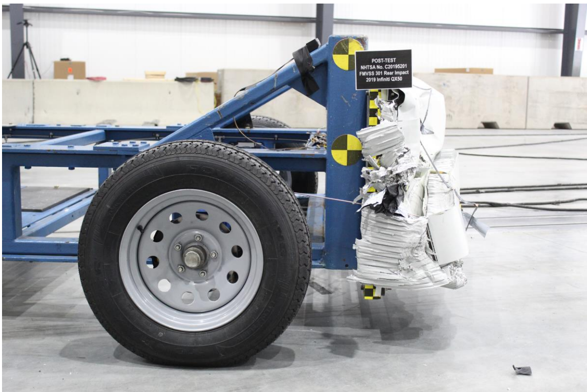
Figure A-24: Post-Test MDB Right Side View
