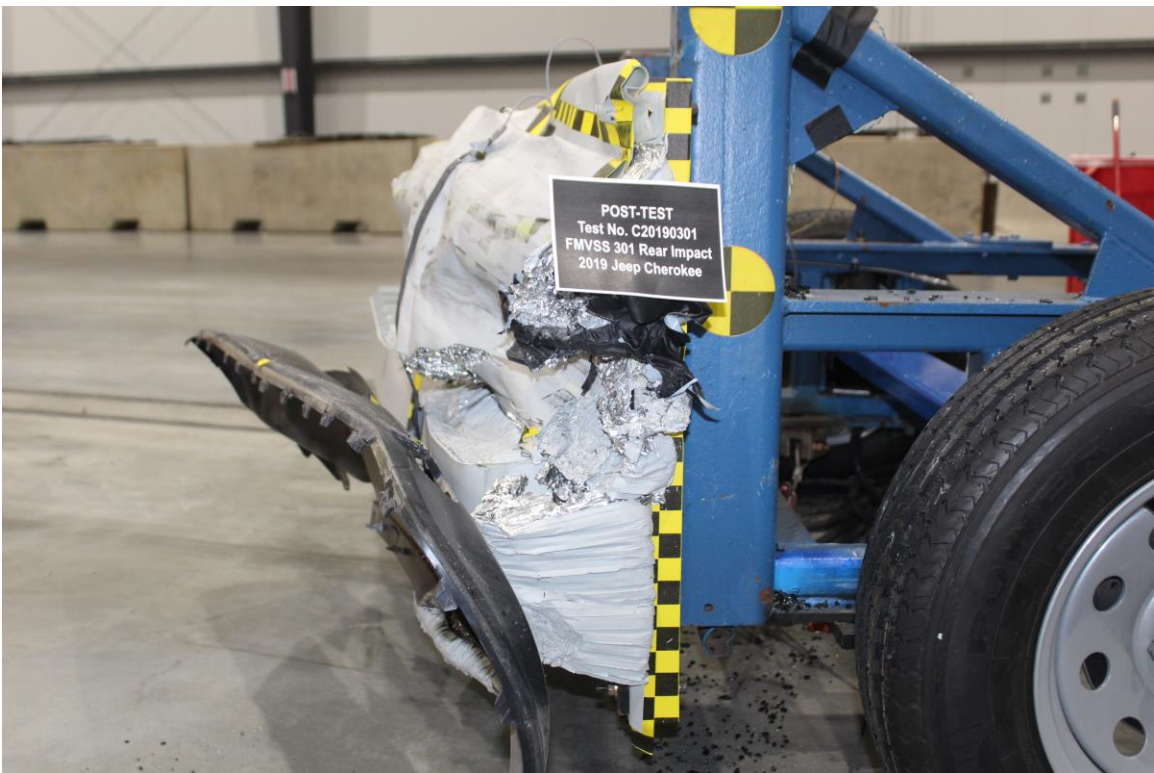
Figure A-22: Post-Test MDB Left Side View
