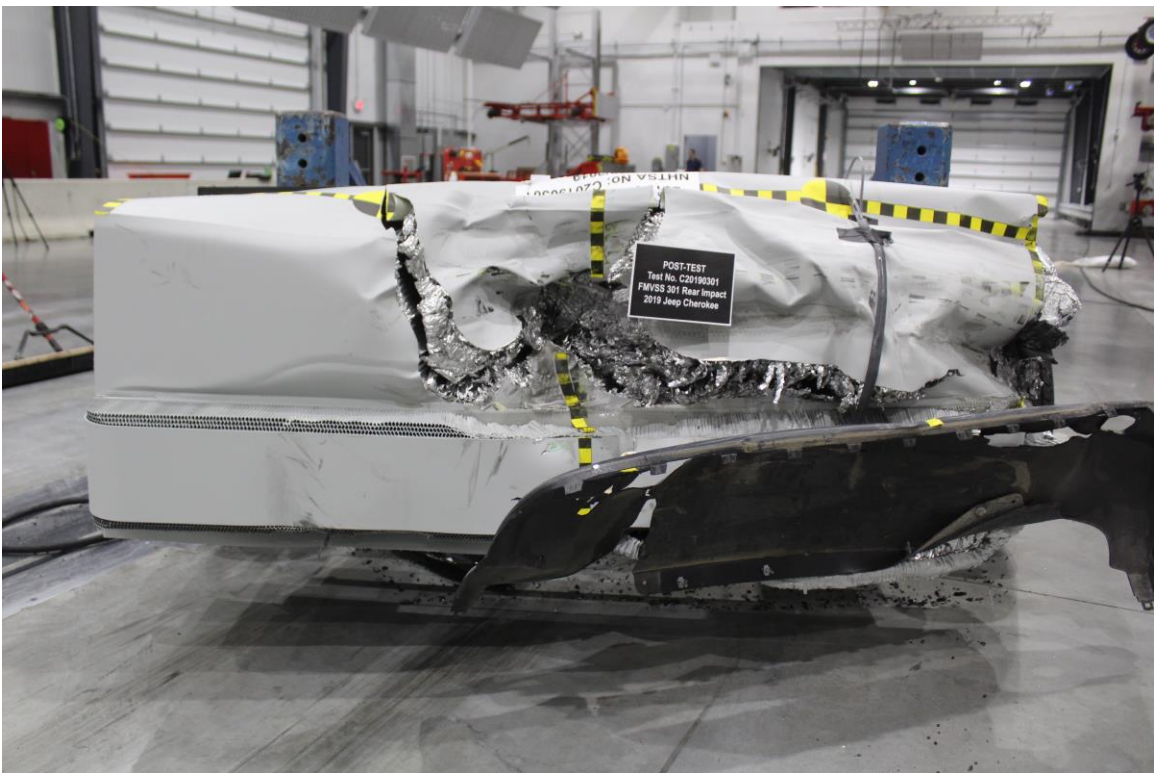
Figure A-20: Post-Test MDB Front View
