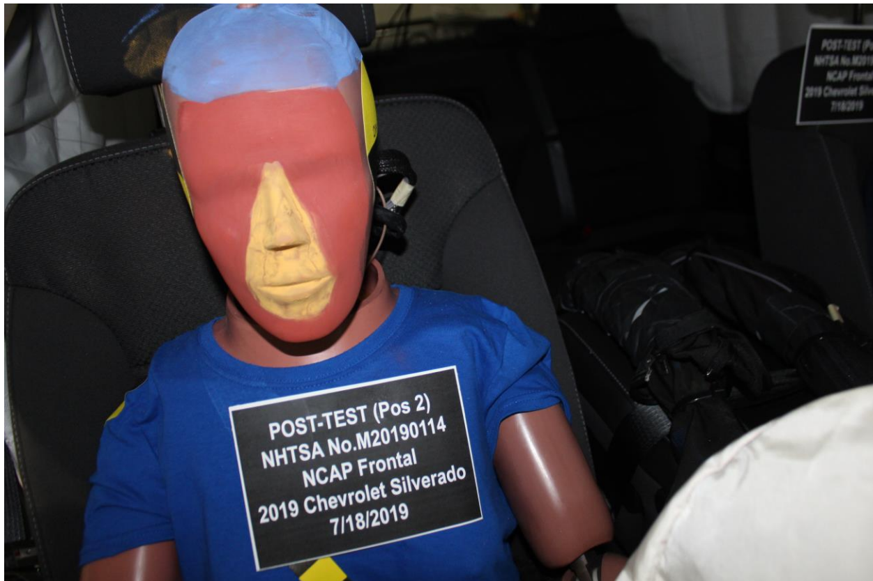
Figure A-67: Post-Test Passenger Dummy Face
