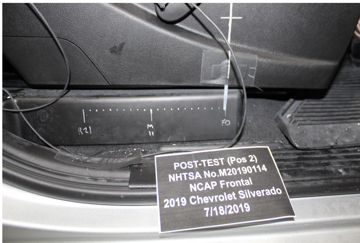
Figure A-58: Post-Test Passenger's Seat Fore-Aft Markings
