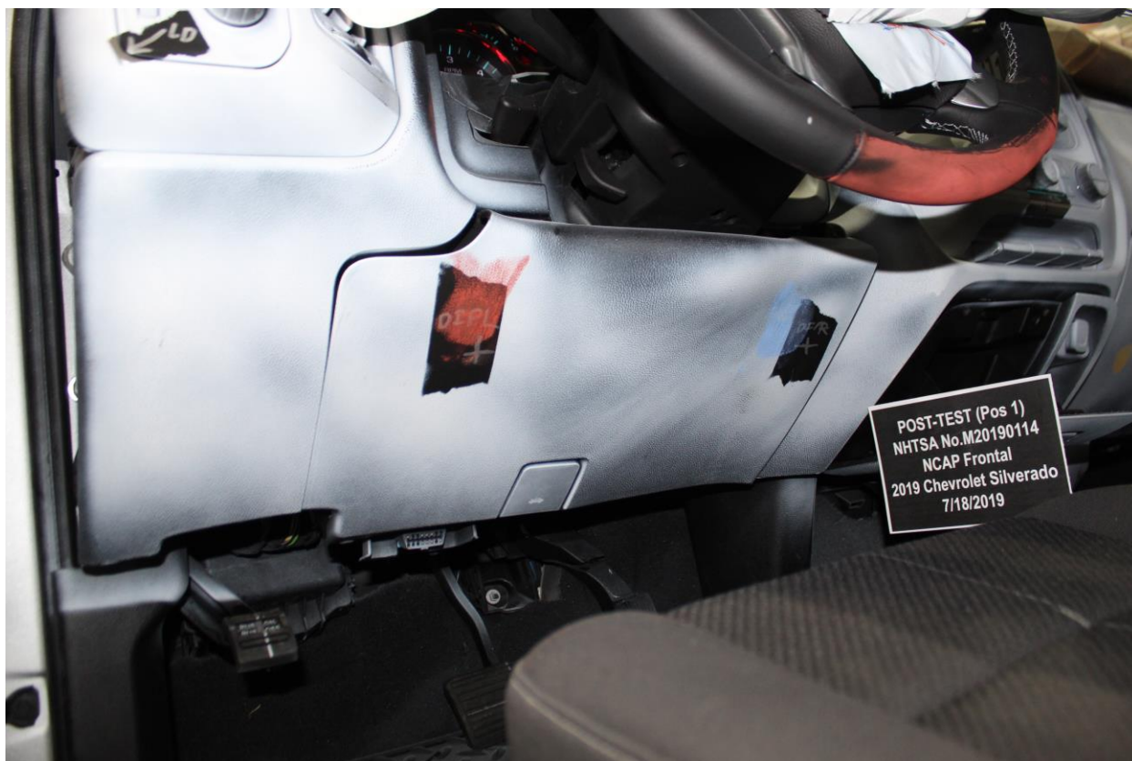
Figure A-43: Post-Test Driver's Side Knee Bolster
