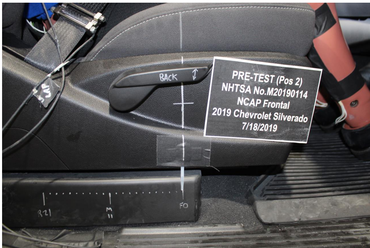
Figure A-57: Pre-Test Passenger's Seat Fore-Aft Markings
