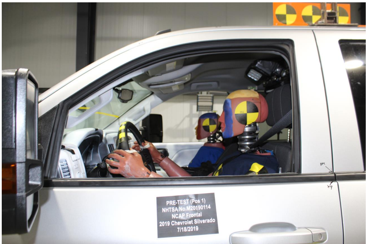
Figure A-32: Pre-Test Driver Dummy Window View
