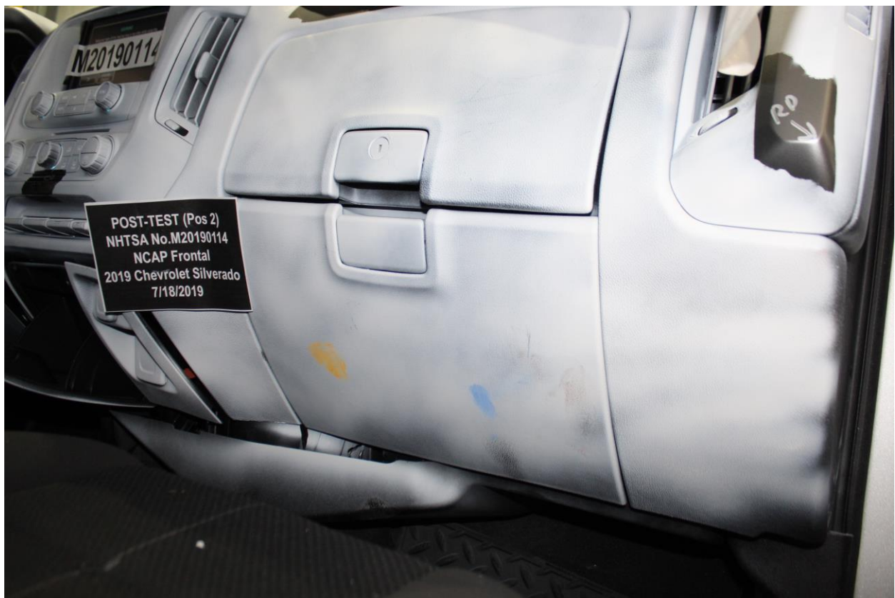
Figure A-64: Post-Test Passenger's Side Knee Bolster
