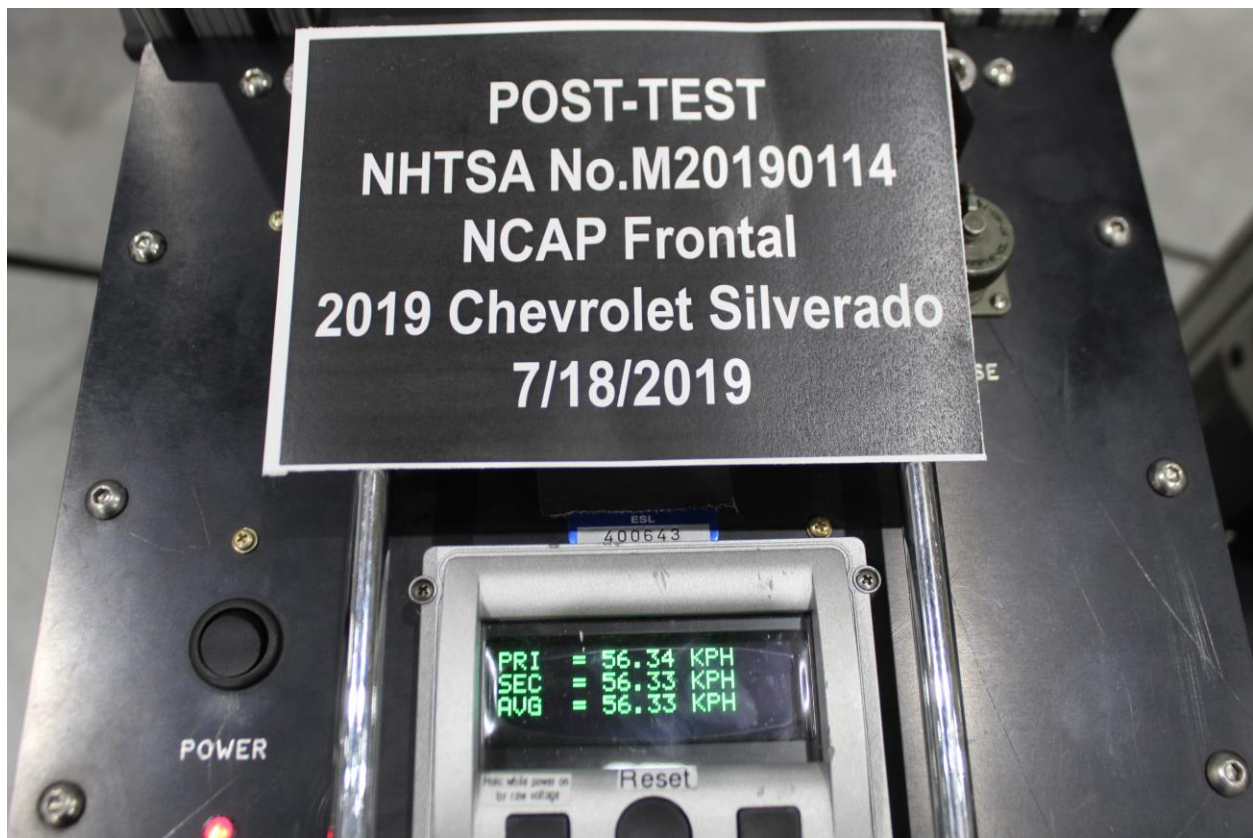
Figure A-72: Post-Test Speed Trap Read-Out
