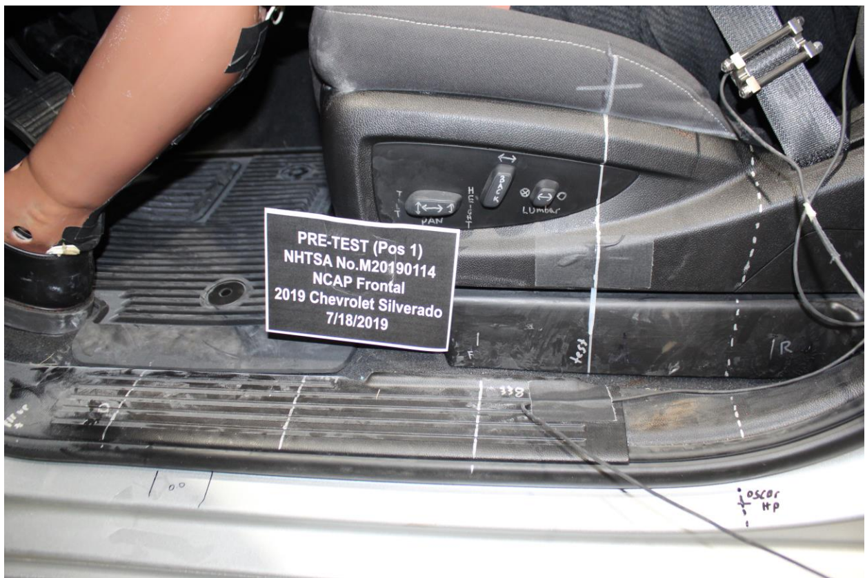
Figure A-36: Pre-Test Driver's Seat Fore-Aft Markings
