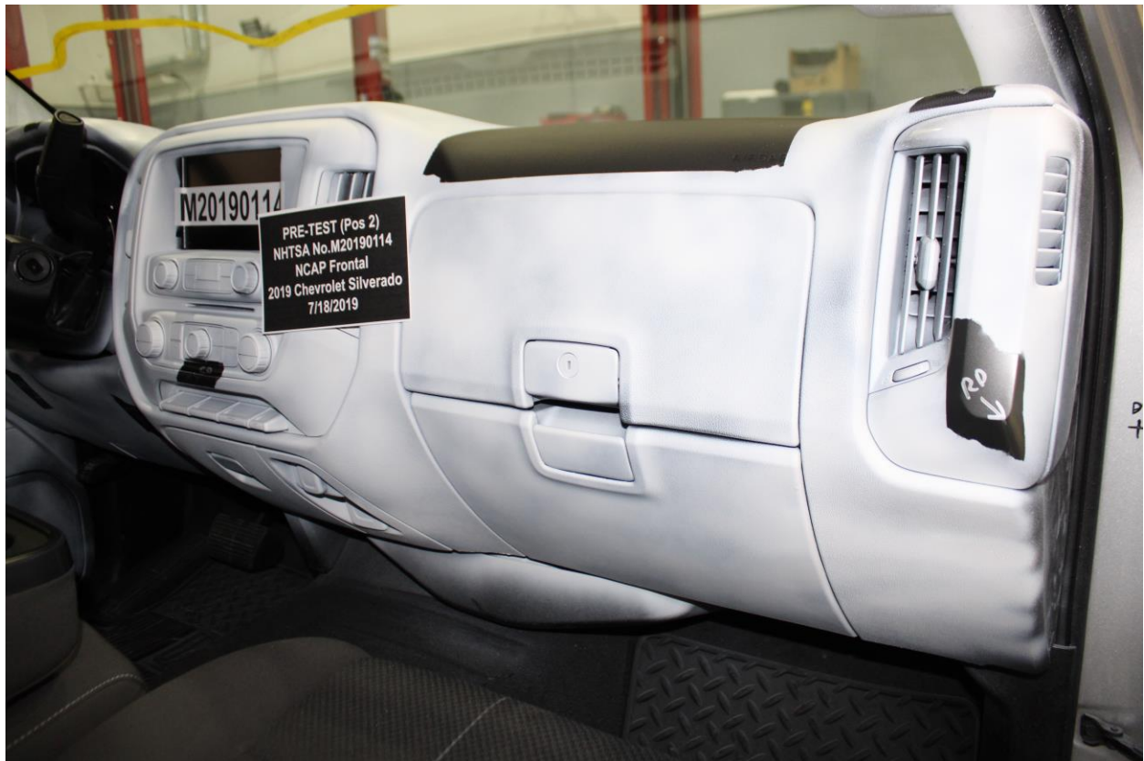
Figure A-63: Pre-Test Passenger's Side Knee Bolster
