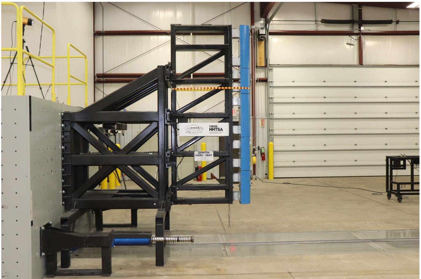
Photo No. 060 - Post-Test Pole Barrier Side View
