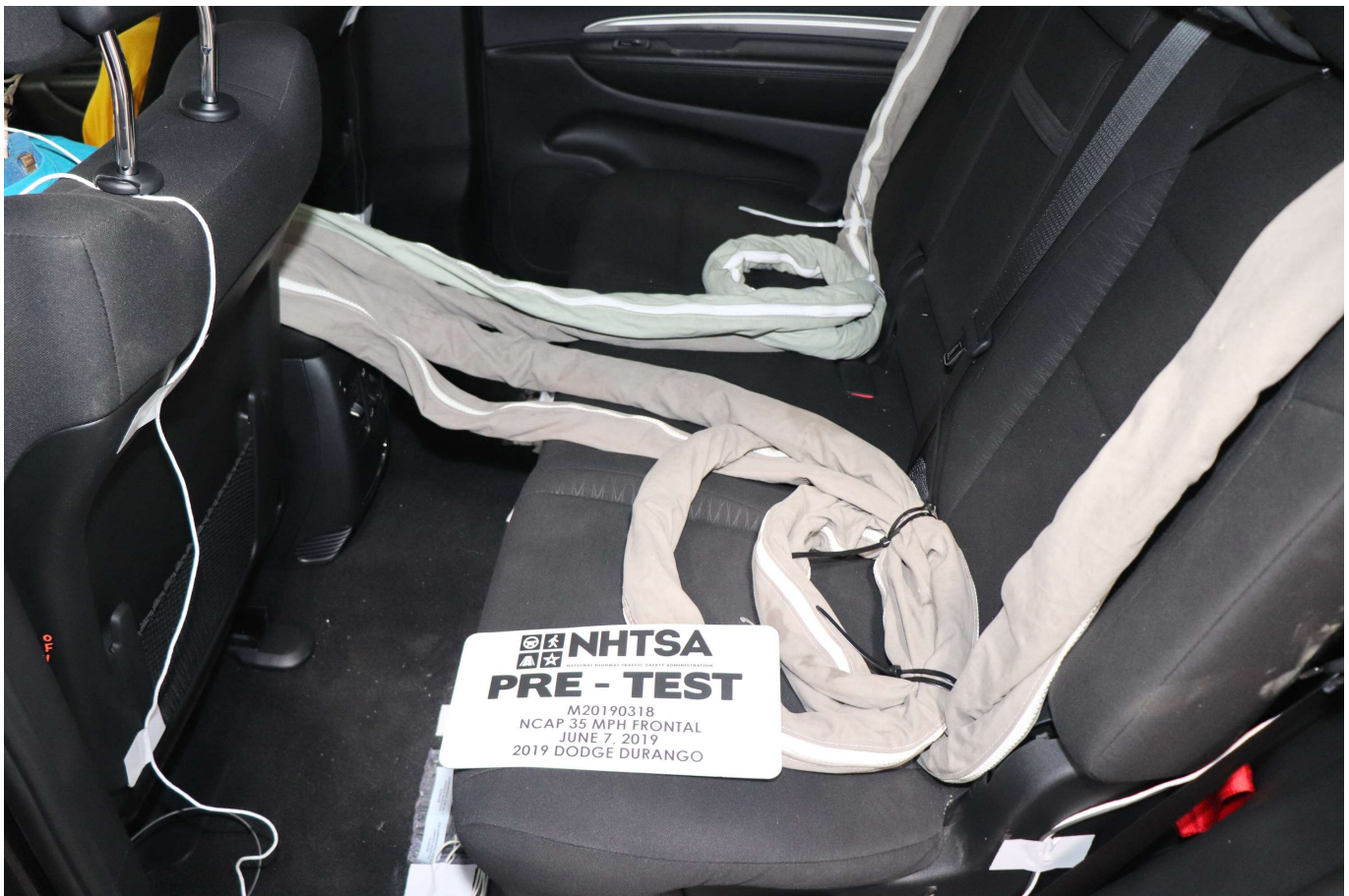
Photo No. 028 - Pre-Test Dummy Cable Routing
