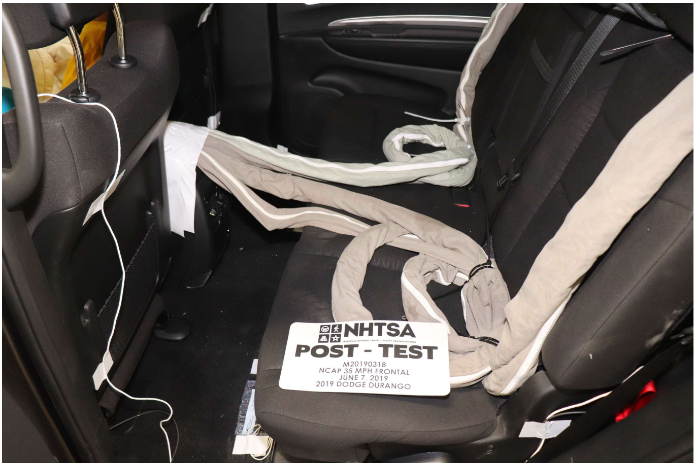
Photo No. 029 - Post-Test Dummy Cable Routing
