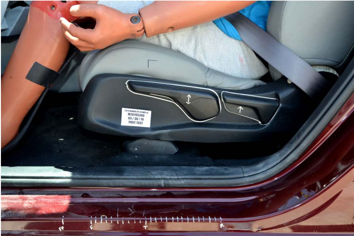
FIGURE 37. Post-Test Driver's Seat Fore-Aft Markings
