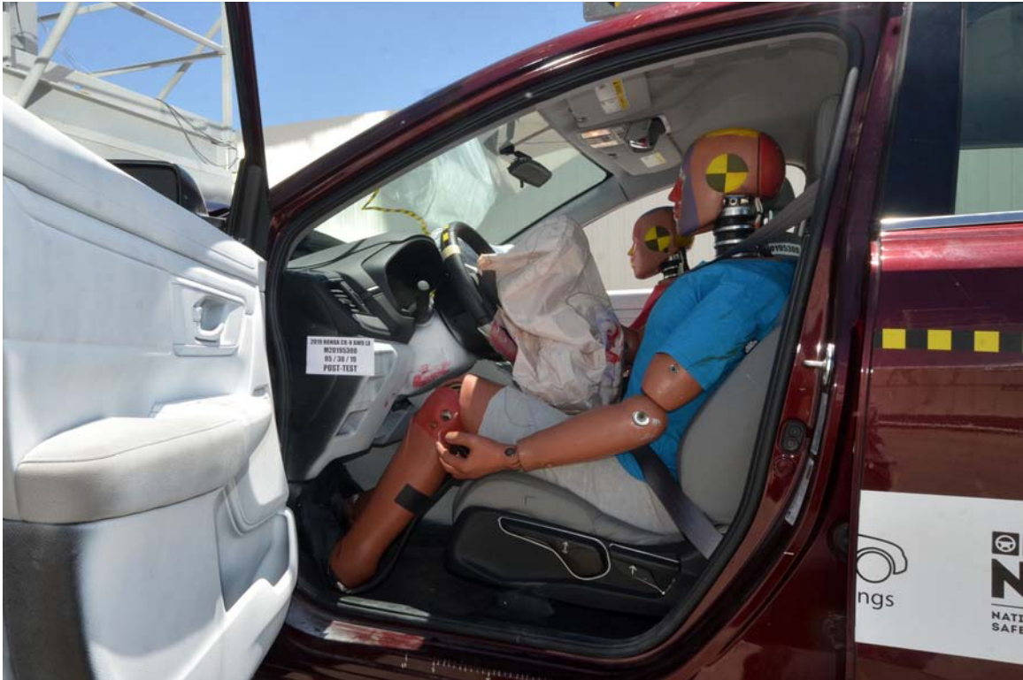
FIGURE 35. Post-Test Driver Dummy and Vehicle Interior View
