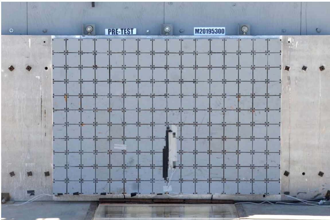
FIGURE 2. Pre-Test Load Cell Wall
