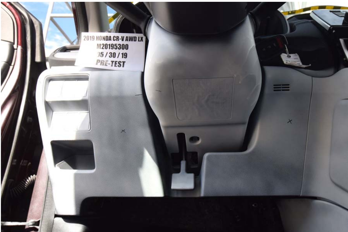
FIGURE 42. Pre-Test Driver's Side Knee Bolster
