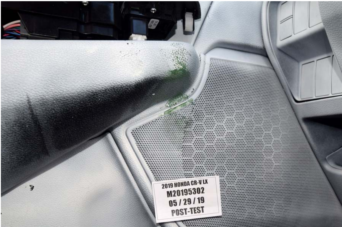
FIGURE 54. Post-Test Driver Dummy Close-Up Knee Contact View
