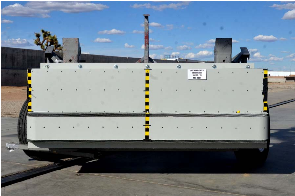
FIGURE 84. Pre-Test Front View of MDB Impactor Face
