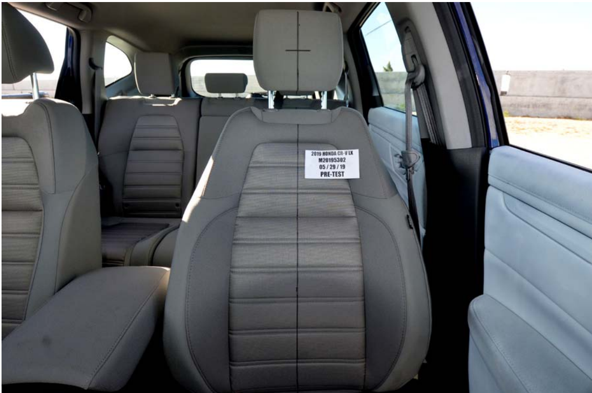
FIGURE 30. Pre-Test Frontal View of Driver Seat Back Prior to Dummy Positioning
