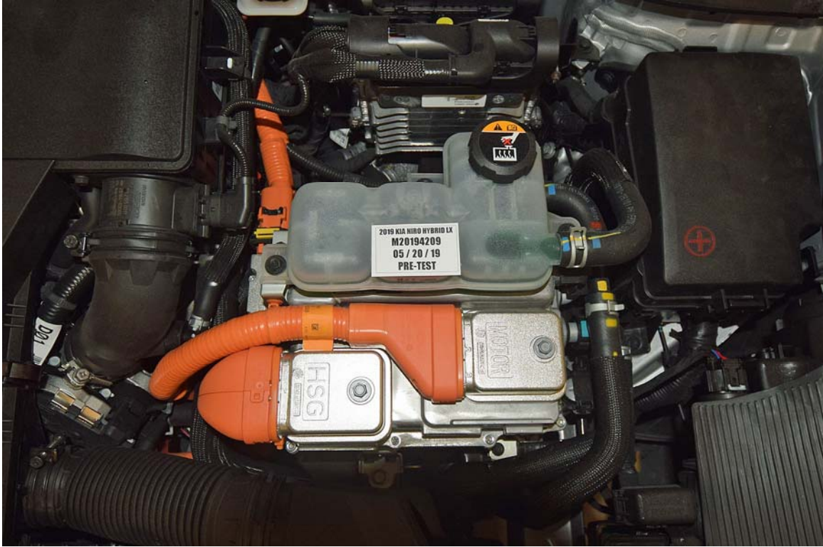
FIGURE 16. Pre-Impact View of Electric Propulsion Drive
