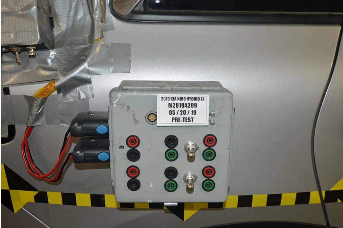
FIGURE 24. Pre-Impact View of Installed Test Interface Port
