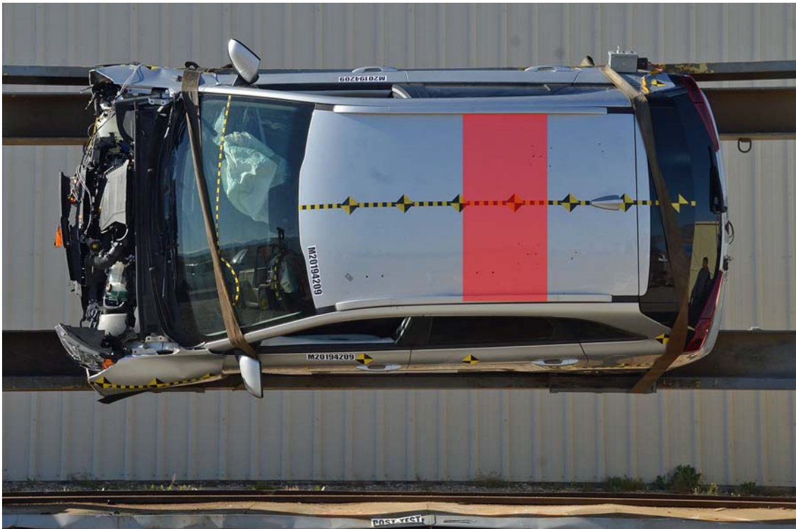
FIGURE 29. FMVSS No. 305 Static Rollover at 90°
