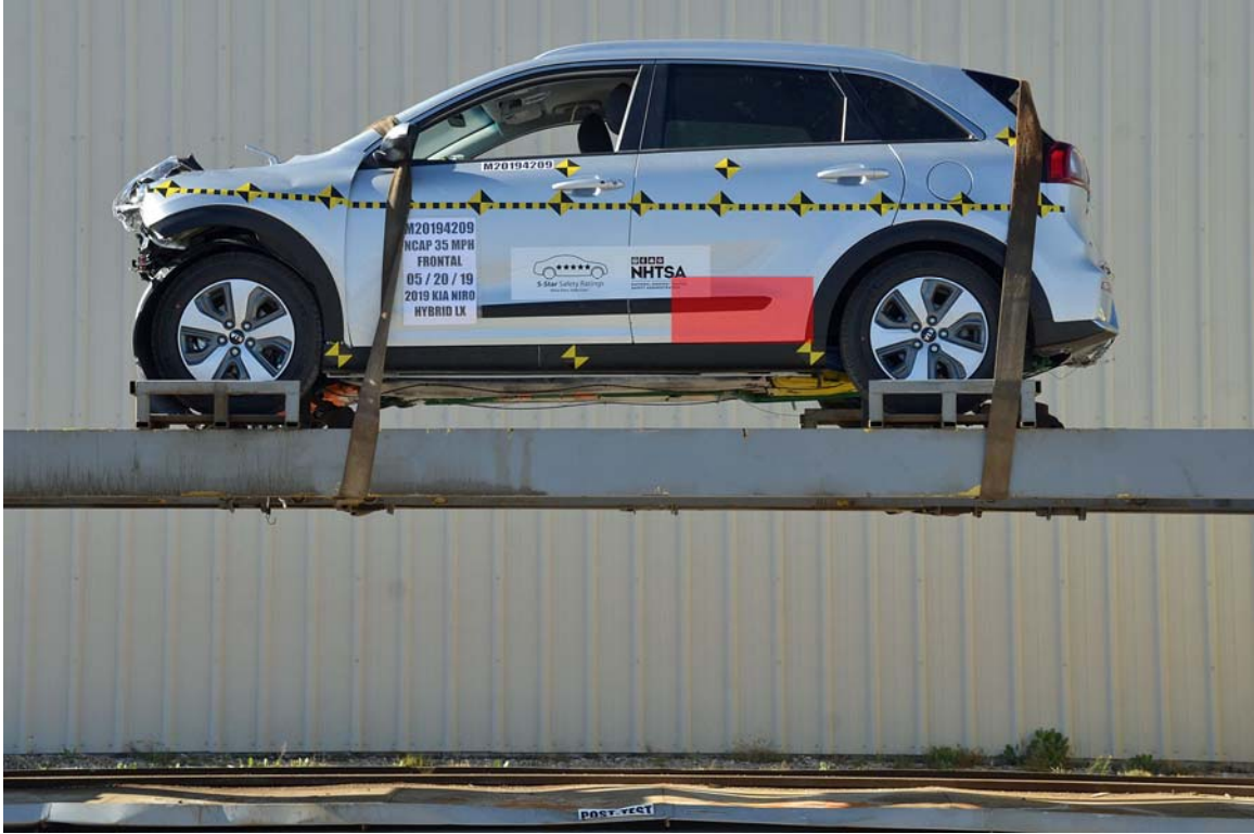
FIGURE 28. FMVSS No. 305 Static Rollover at 0°
