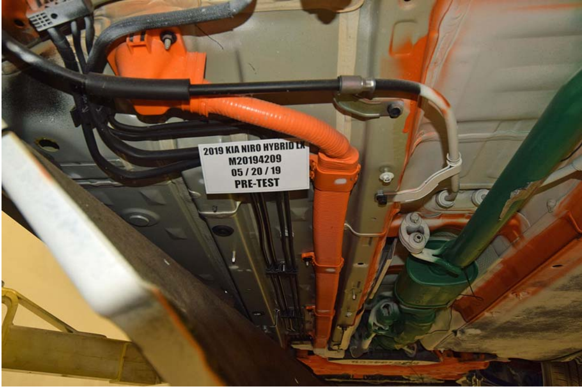
FIGURE 18. Pre-Impact View of High Voltage Interconnect(s)
