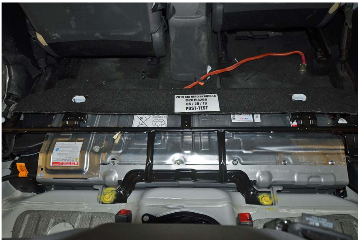
FIGURE 11. Post-Impact Rear View of Propulsion Battery
