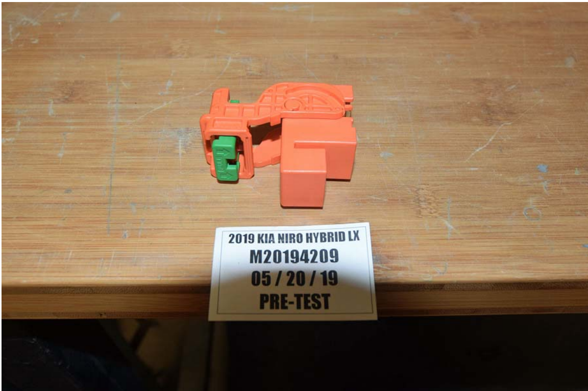
FIGURE 7. Manual High Voltage Service Disconnect Removed
