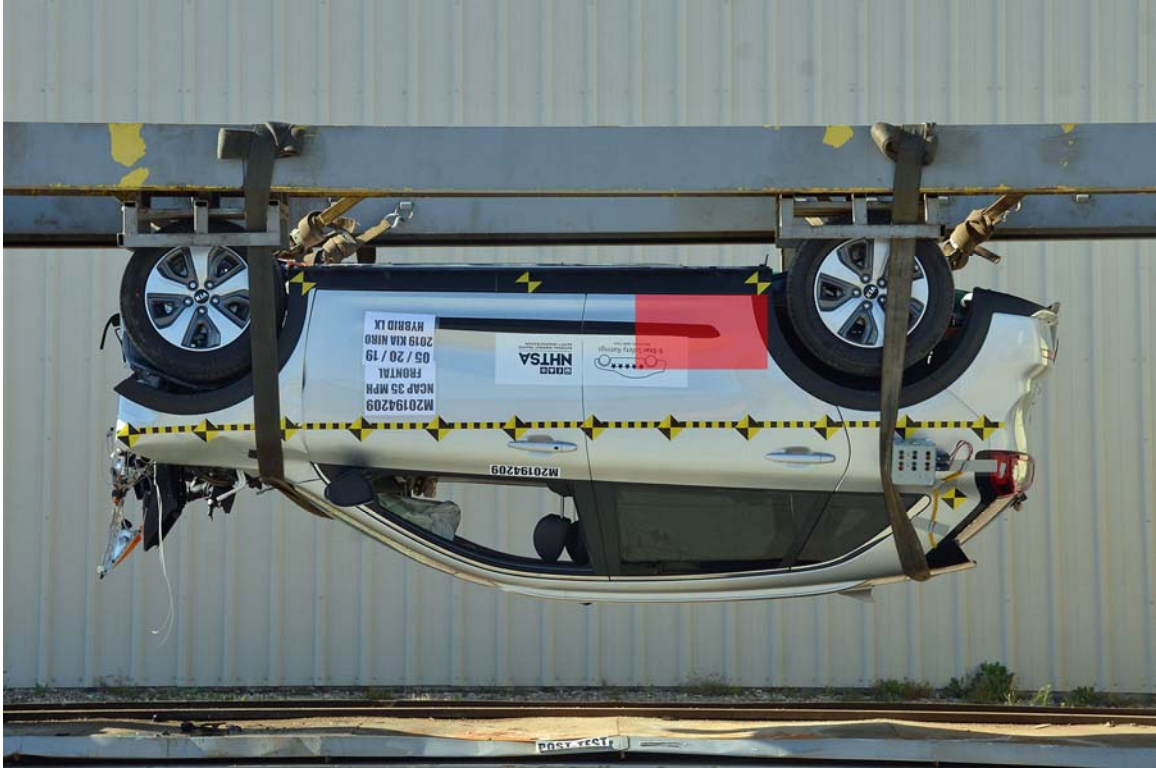
FIGURE 30. FMVSS No. 305 Static Rollover at 180°
