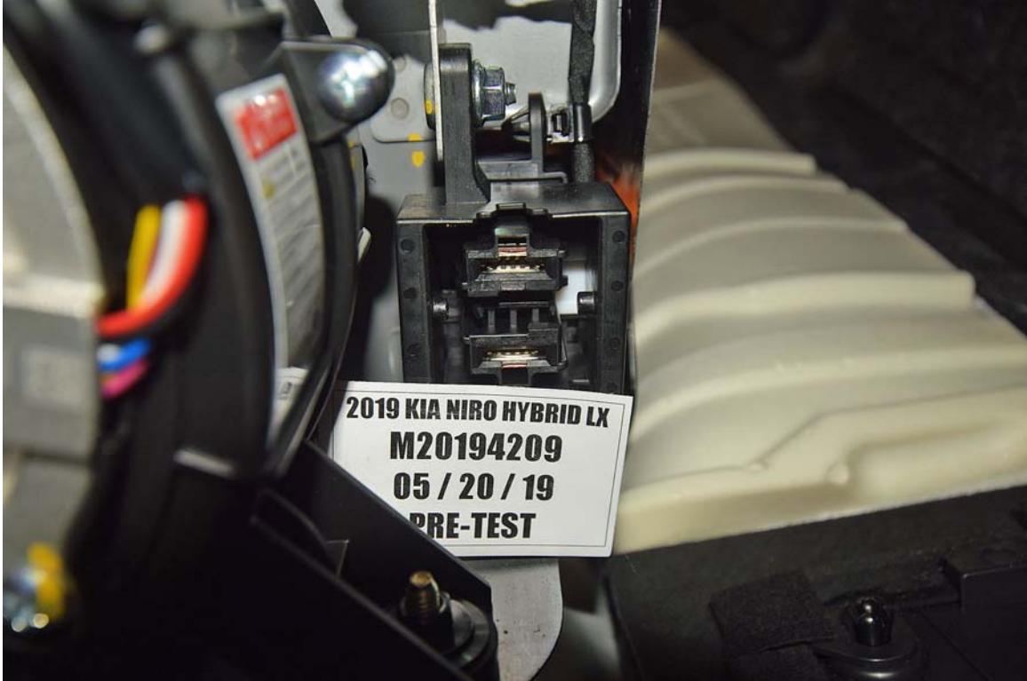
FIGURE 8. Manual High Voltage Service Disconnect Removed
