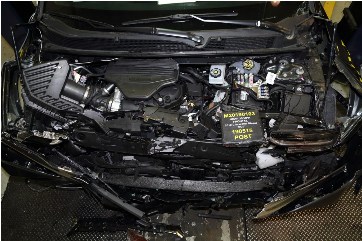
021 Post-Test Engine Compartment View
