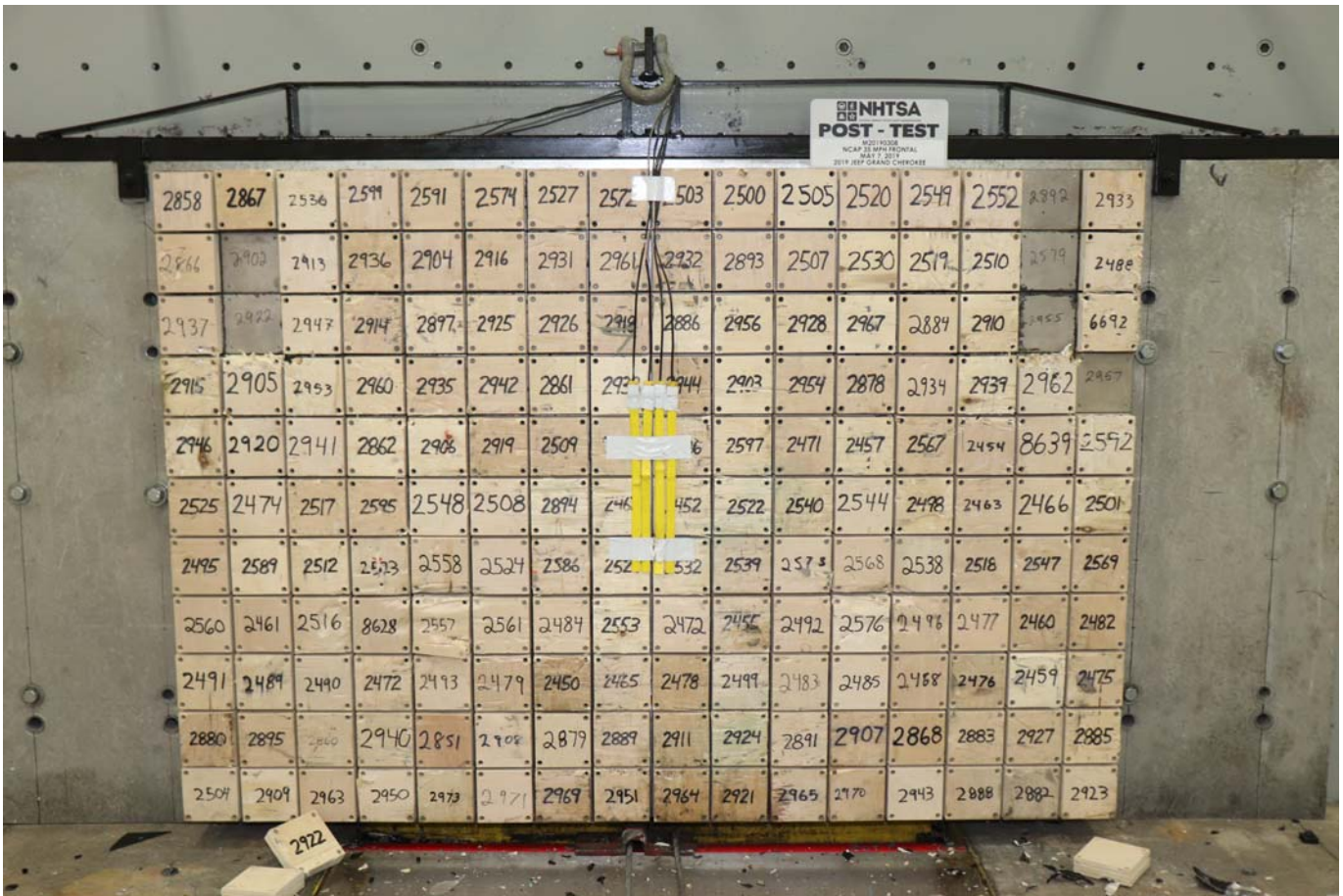
Photo No. 003 - Post-Test Load Cell Wall
