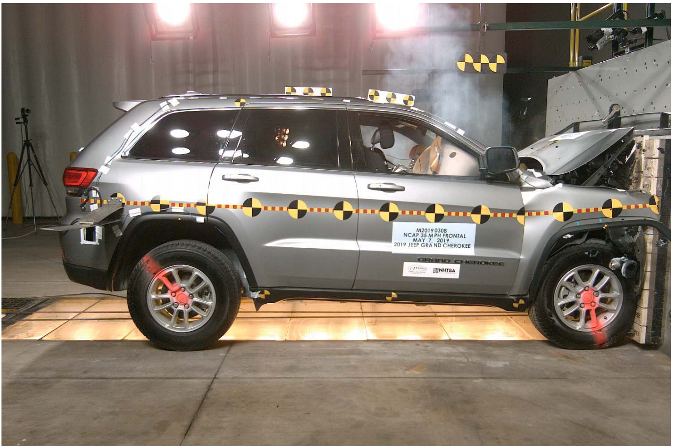
Photo No. 078 - 2019 Jeep Grand Cherokee Laredo 4x4 5-Door SUV Frontal Impact Event
