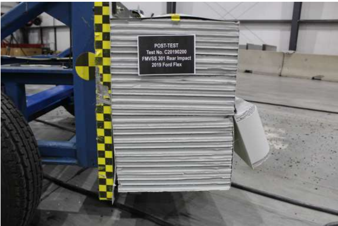
Figure A-24: Post-Test MDB Right Side View
