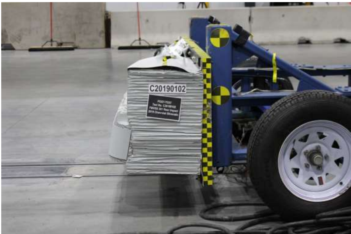
Figure A-22: Post-Test MDB Left Side View
