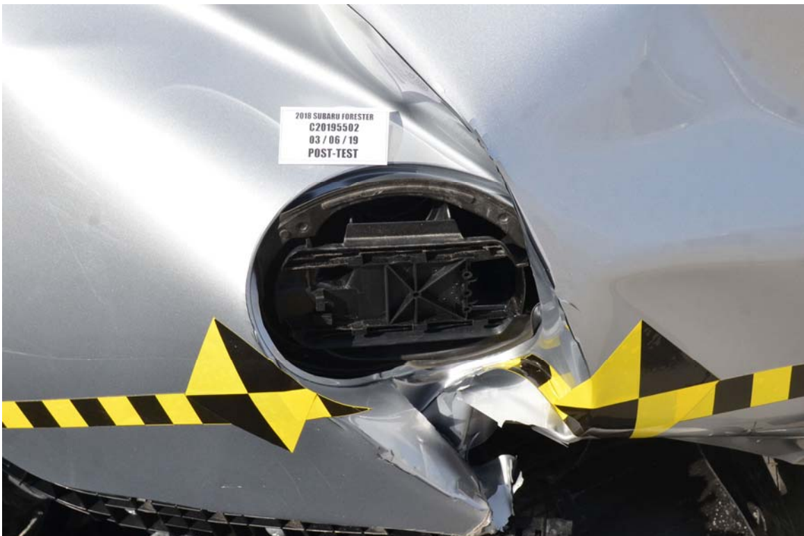
FIGURE 24. Post-Test View of Fuel Filler Cap
