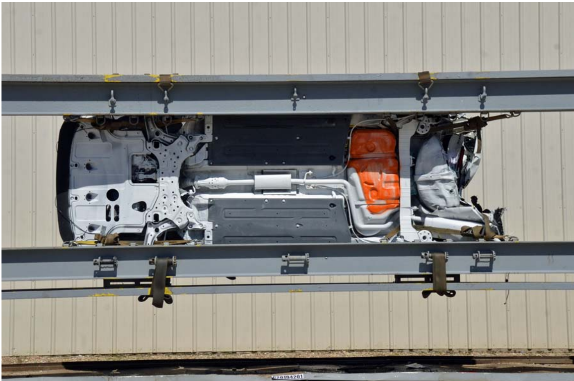
FIGURE 34. Test Vehicle at 270° on FMVSS 301 Static Rollover Device
