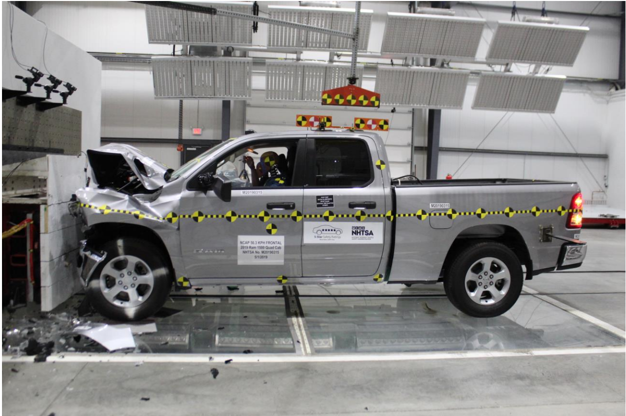
Figure A-11: Post-Test Left View of Test Vehicle
