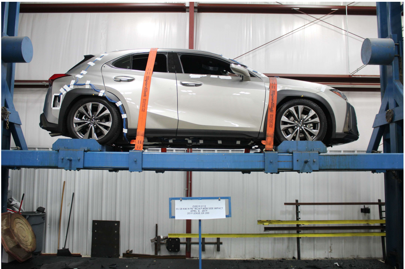
Photo No. 096 - FMVSS Photo No. 301 Static Rollover 0 Degrees
