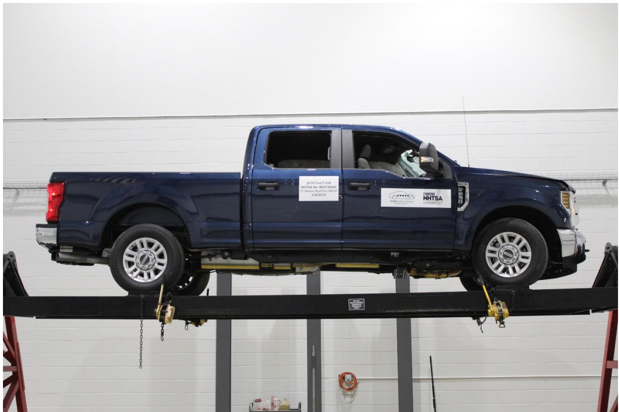
Figure A-67: FMVSS No. 301 Static Rollover 360 Degrees
