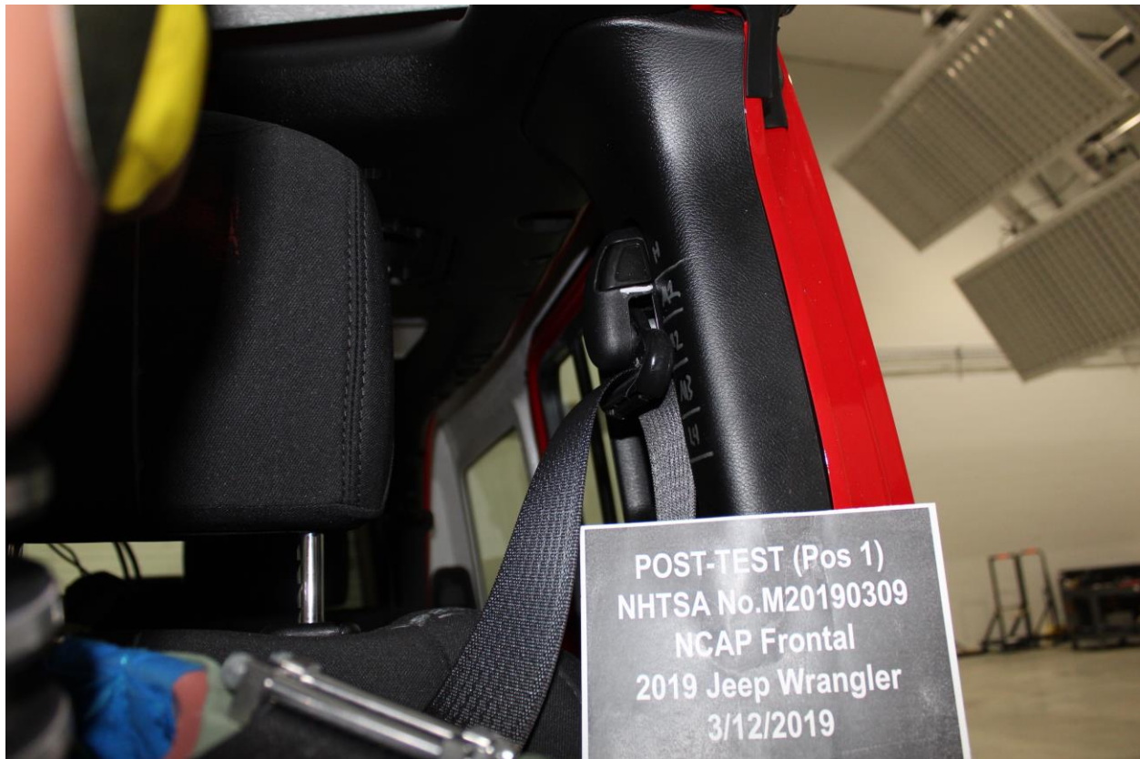
Figure A-39: Post-Test View of Belt Anchorage for Driver Dummy
