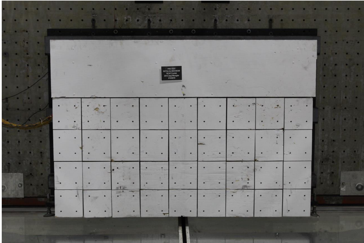
Figure A-2: Pre-Test Load Cell Wall
