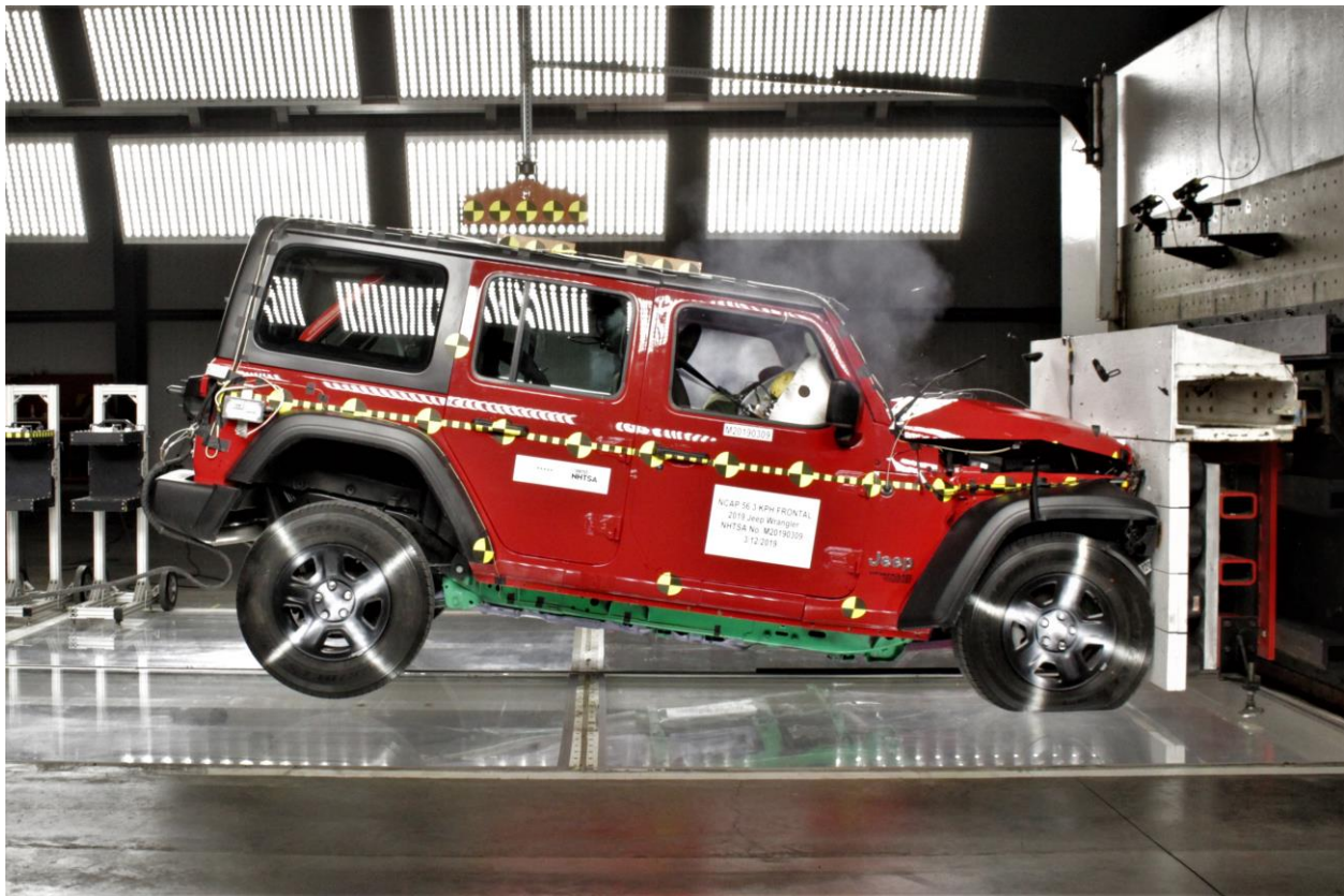
Figure A-78: 2019 Jeep Wrangler Unlimited Frontal Impact Event
