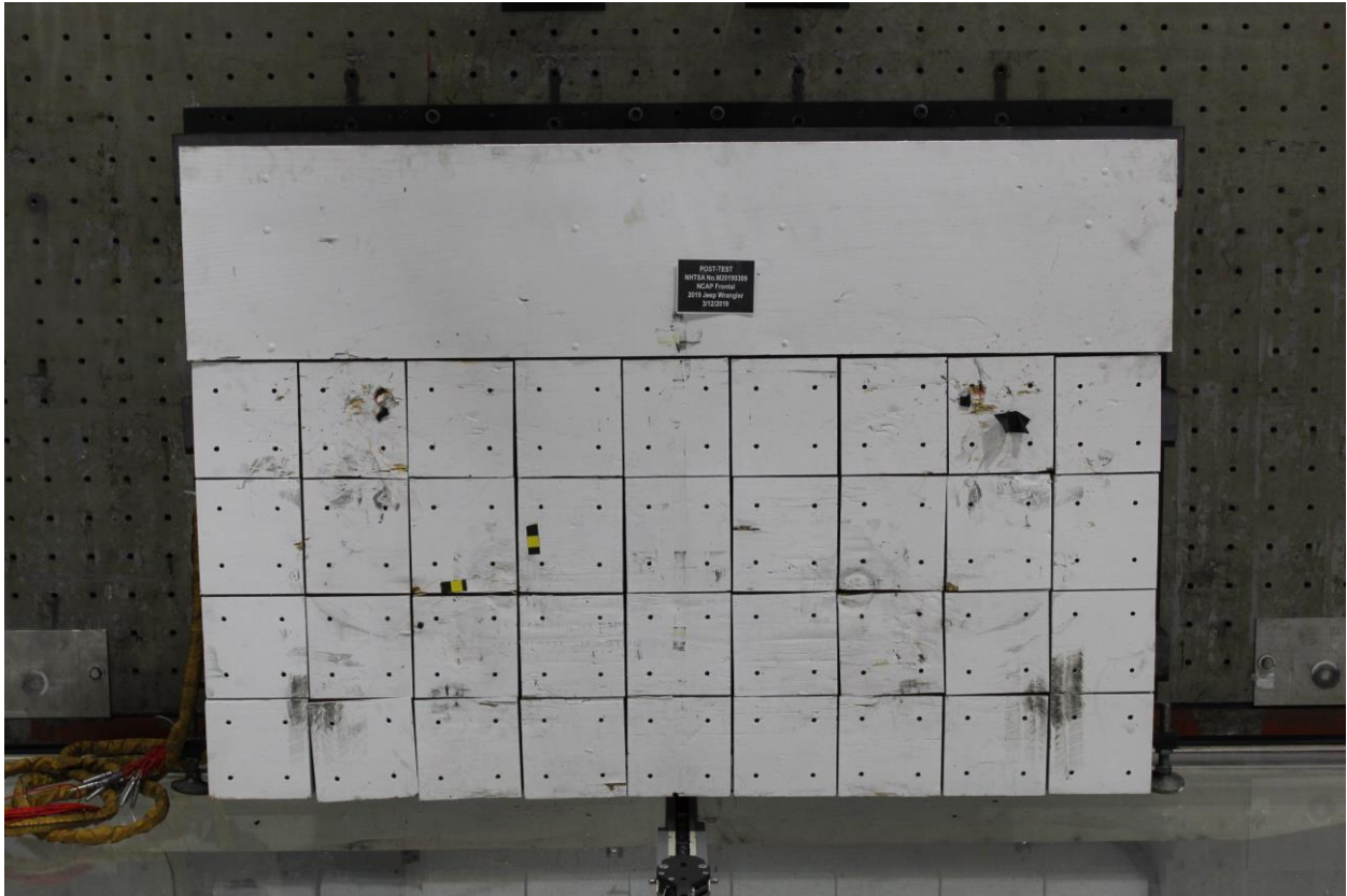
Figure A-3: Post-Test Load Cell Wall
