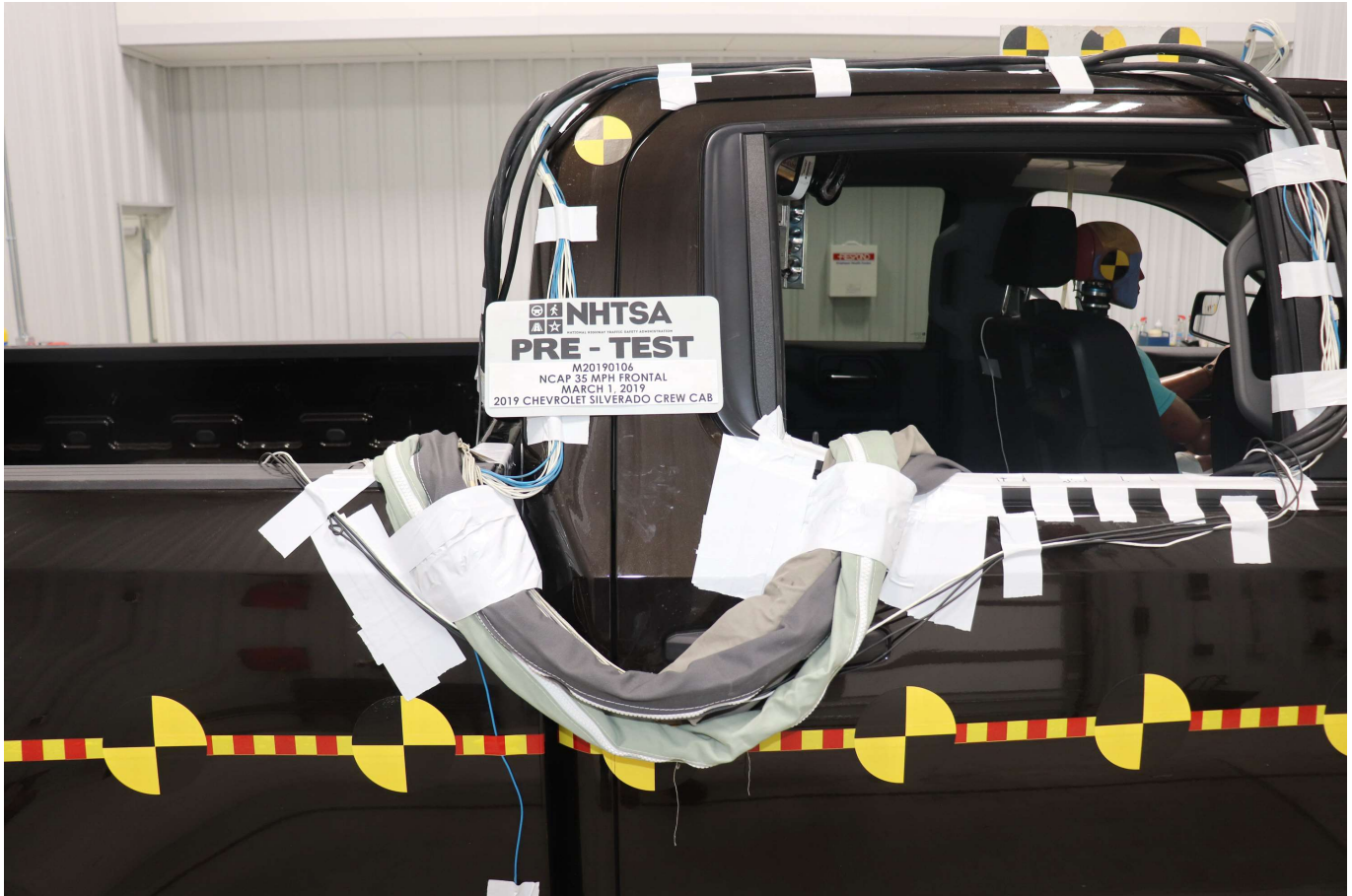
Photo No. 028 - Pre-Test Dummy Cable Routing
