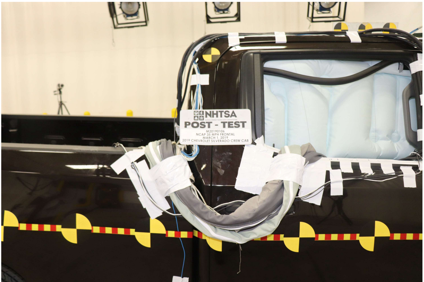
Photo No. 029 - Post-Test Dummy Cable Routing
