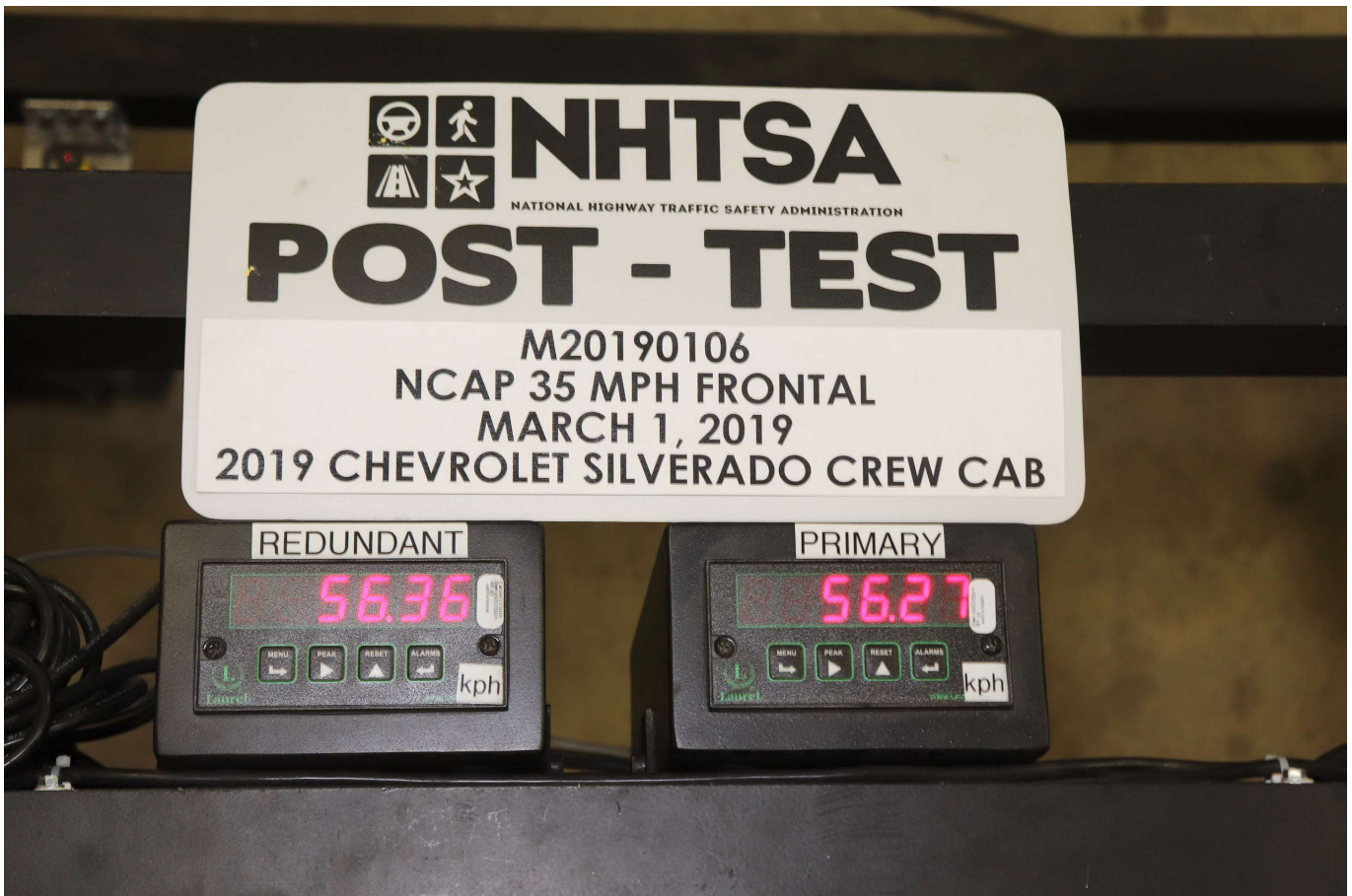
Photo No. 072 - Post-Test Speed Trap Read-Out
