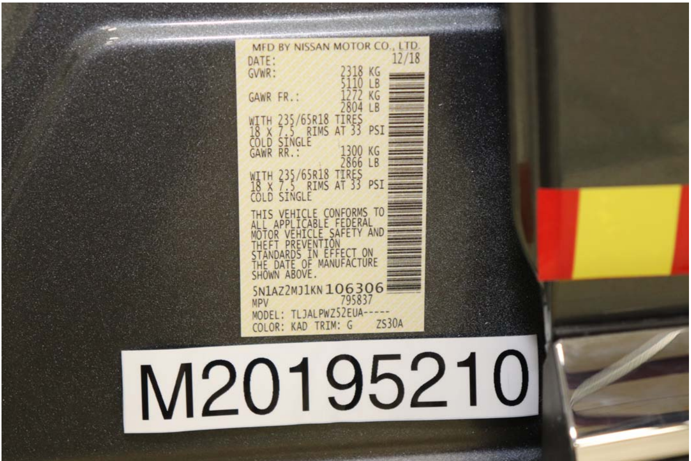
Photo No. 055 - Close-Up View of Vehicle Certification Label
