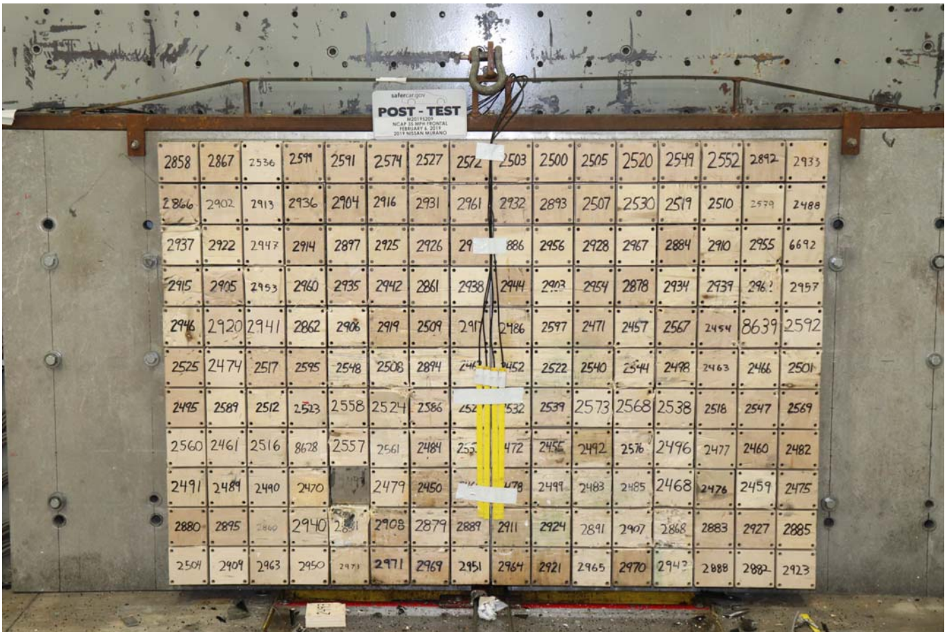
Photo No. 003 - Post-Test Load Cell Wall
