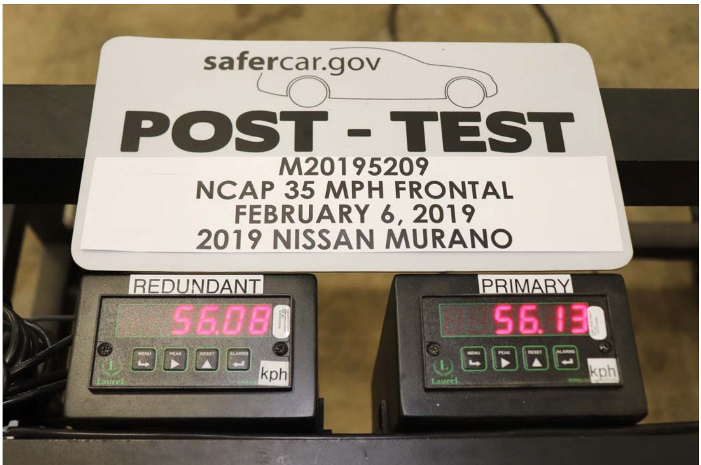
Photo No. 072 - Post-Test Speed Trap Read-Out
