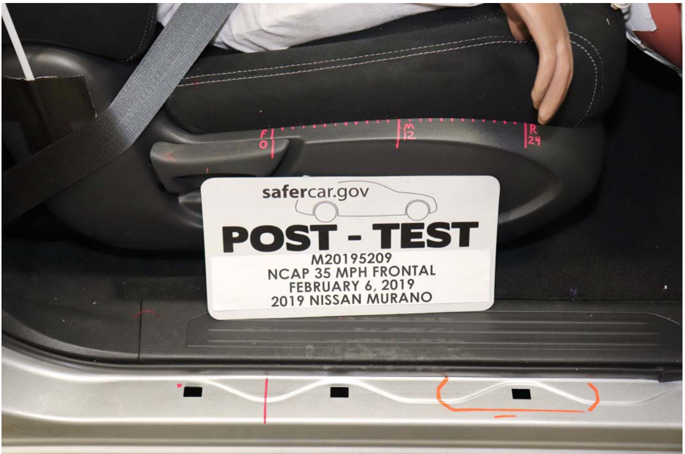
Photo No. 058 - Post-Test Passenger Seat Fore-Aft Markings
