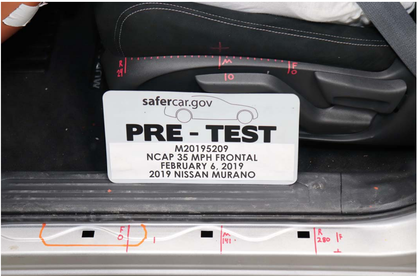
Photo No. 036 - Pre-Test Driver Seat Fore-Aft Markings
