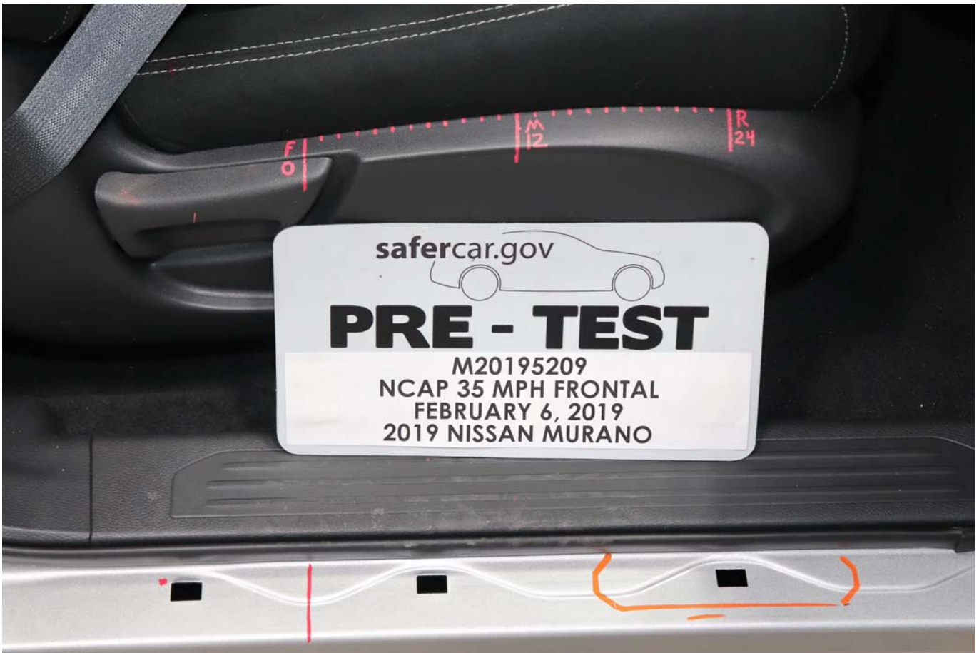
Photo No. 057 - Pre-Test Passenger Seat Fore-Aft Markings
