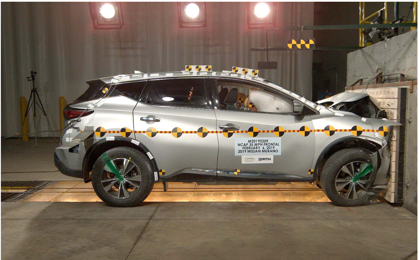
Photo No. 078 - 2019 Nissan Murano S AWD 5-Door SUV Frontal Impact Event
