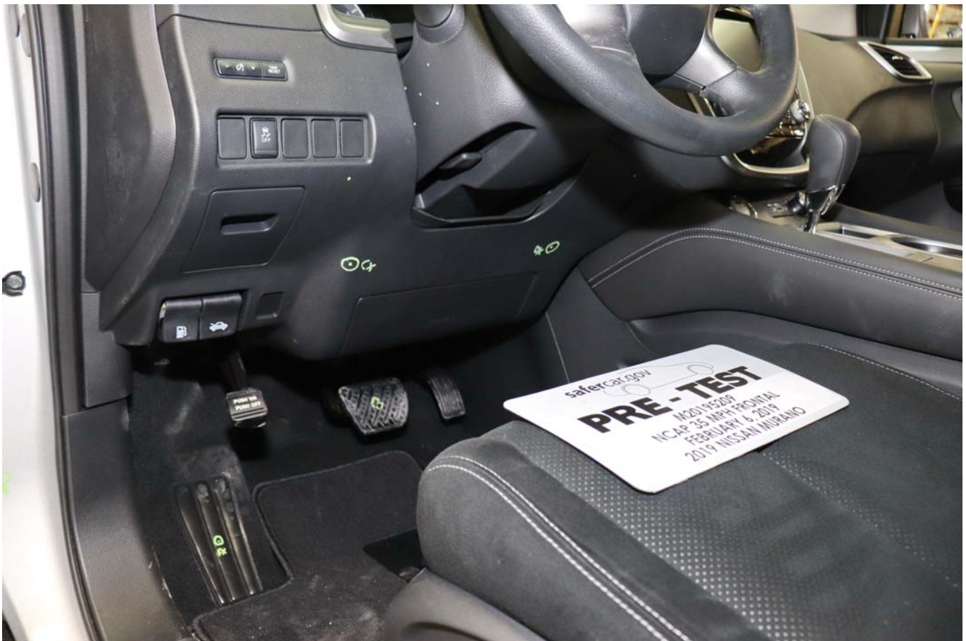
Photo No. 042 - Pre-Test Driver Side Knee Bolster
