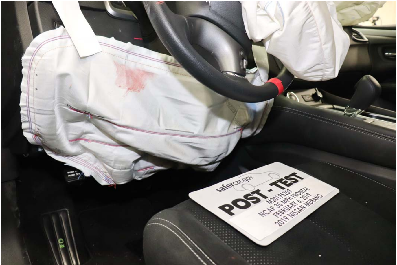
Photo No. 043 - Post-Test Driver Side Knee Bolster
