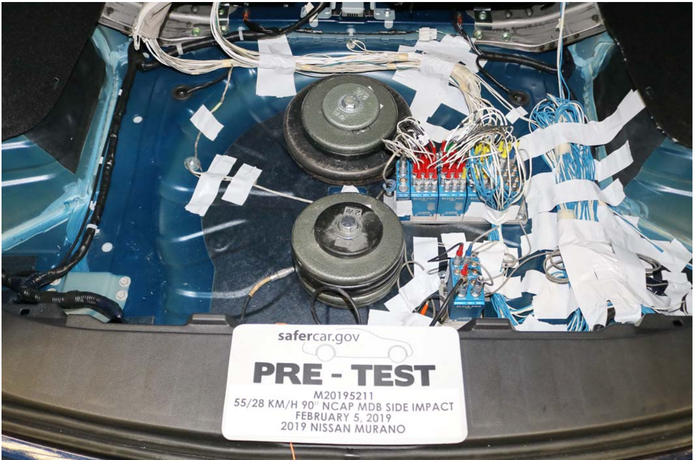
Photo No. 094 - Pre-Test Ballast View
