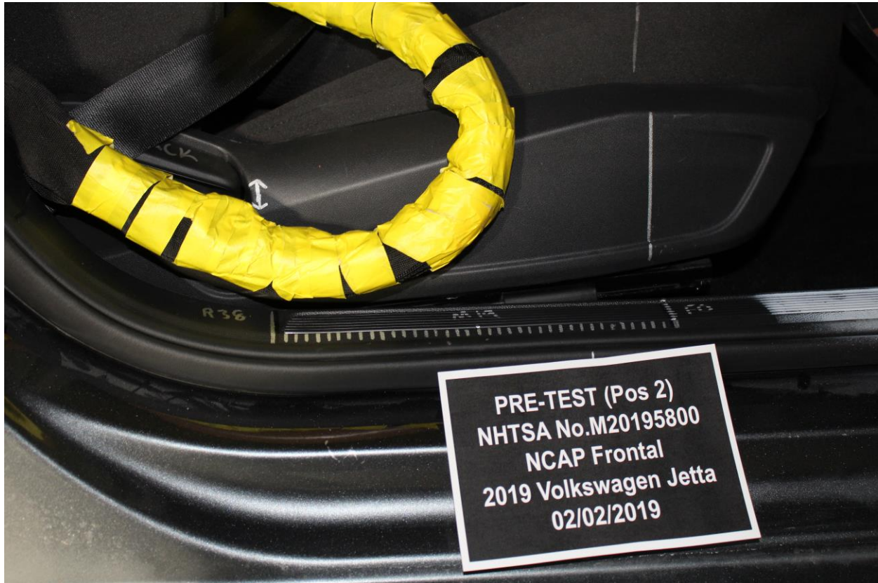
Figure A-57: Pre-Test Passenger's Seat Fore-Aft Markings
