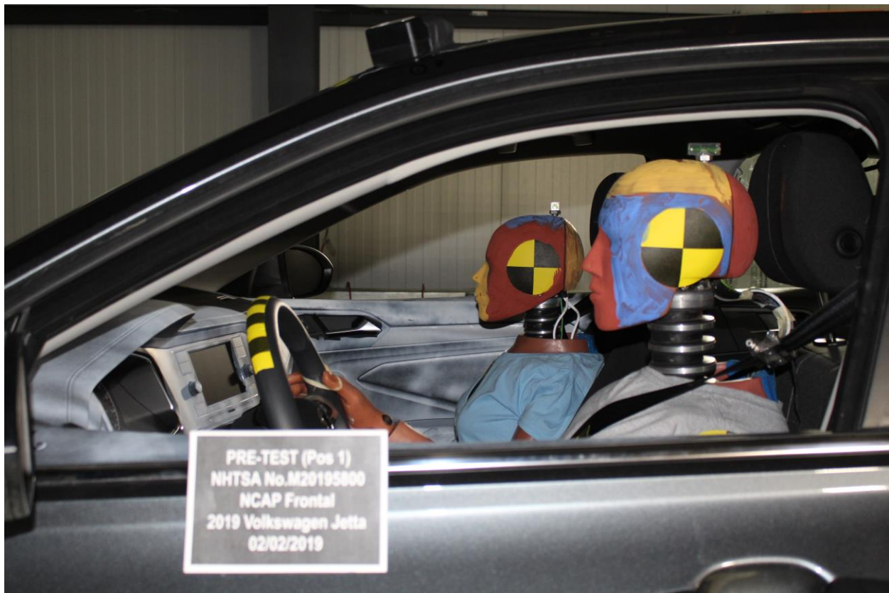
Figure A-32: Pre-Test Driver Dummy Window View
