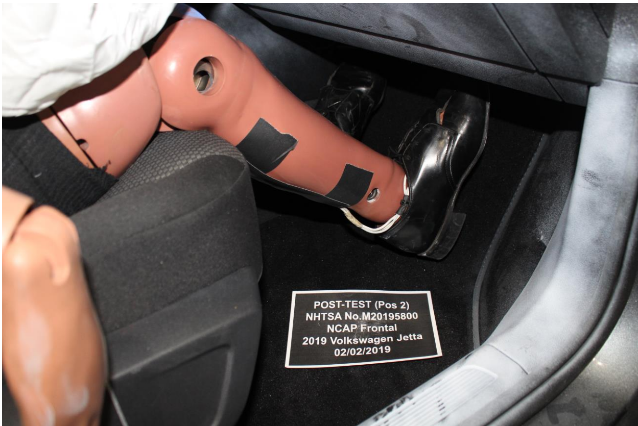
Figure A-62: Post-Test Passenger Dummy Feet
