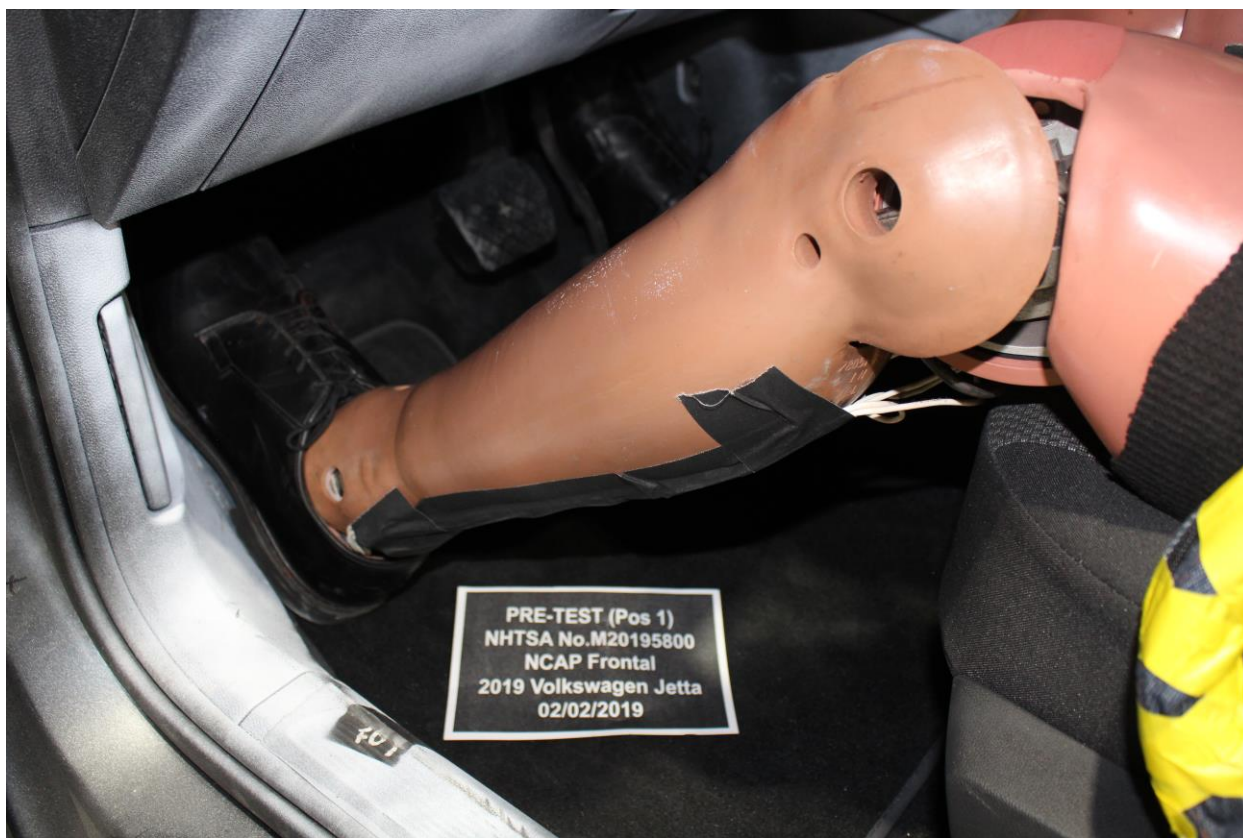
Figure A-40: Pre-Test Driver Dummy Feet
