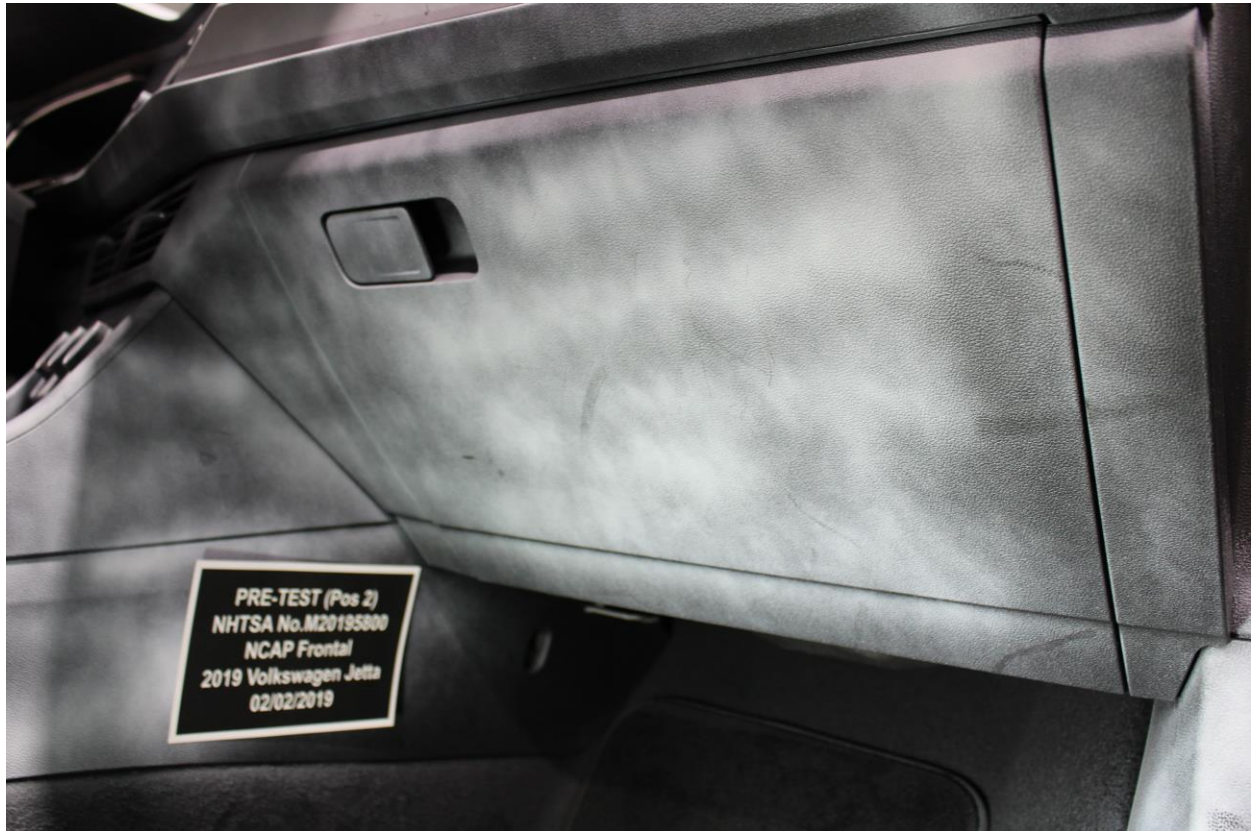
Figure A-63: Pre-Test Passenger's Side Knee Bolster
