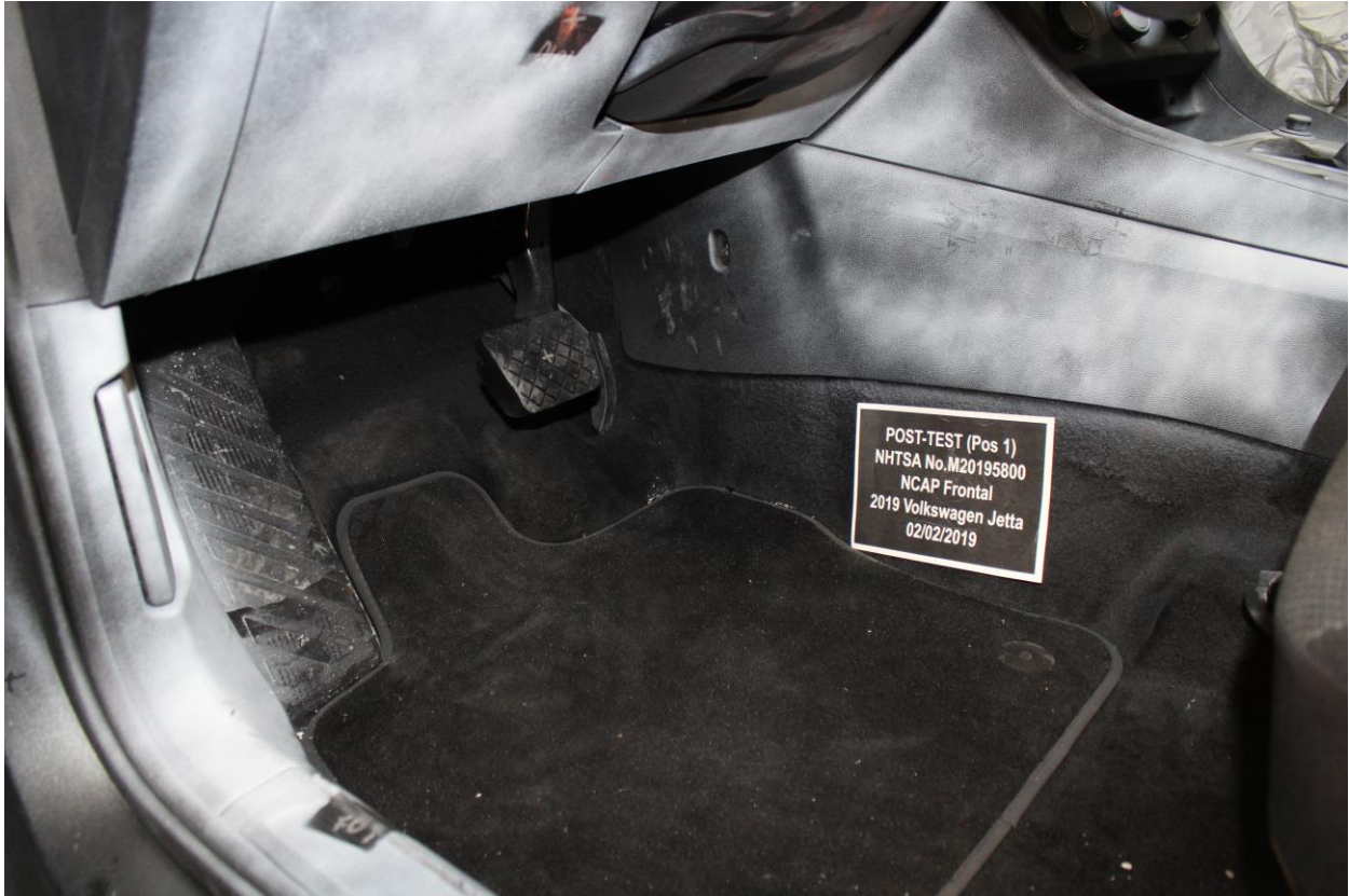
Figure A-45: Post-Test Driver's Side Floorpan
