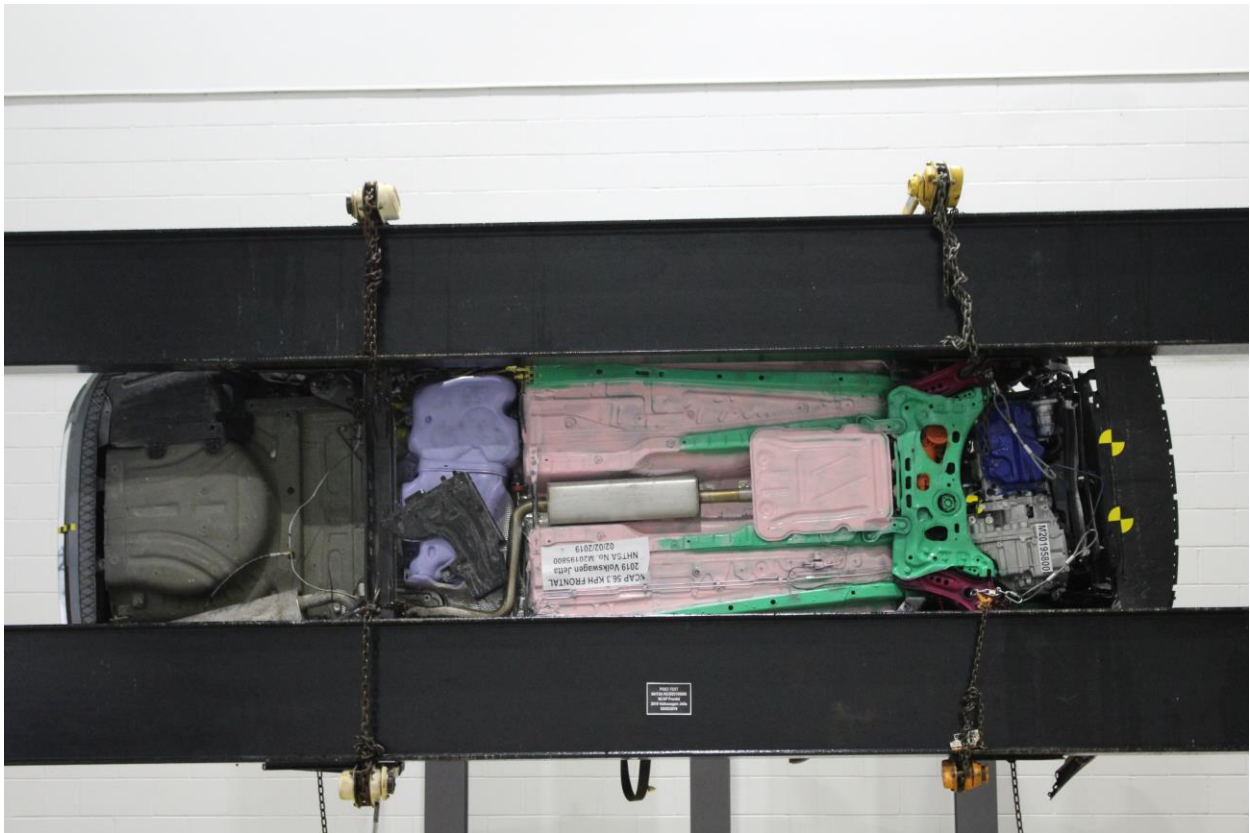
Figure A-76: Vehicle at 270° on Static Rollover Device
