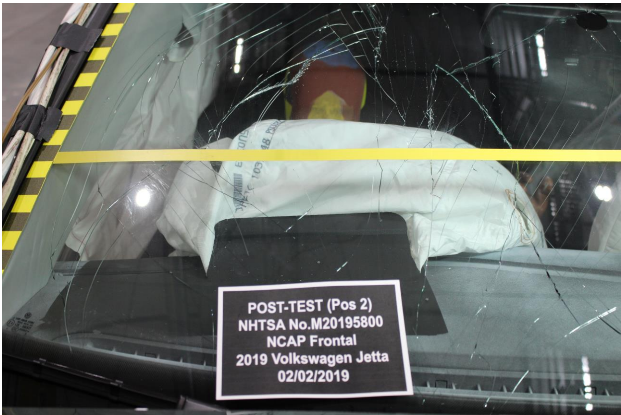
Figure A-52: Post-Test Passenger Dummy Front View
