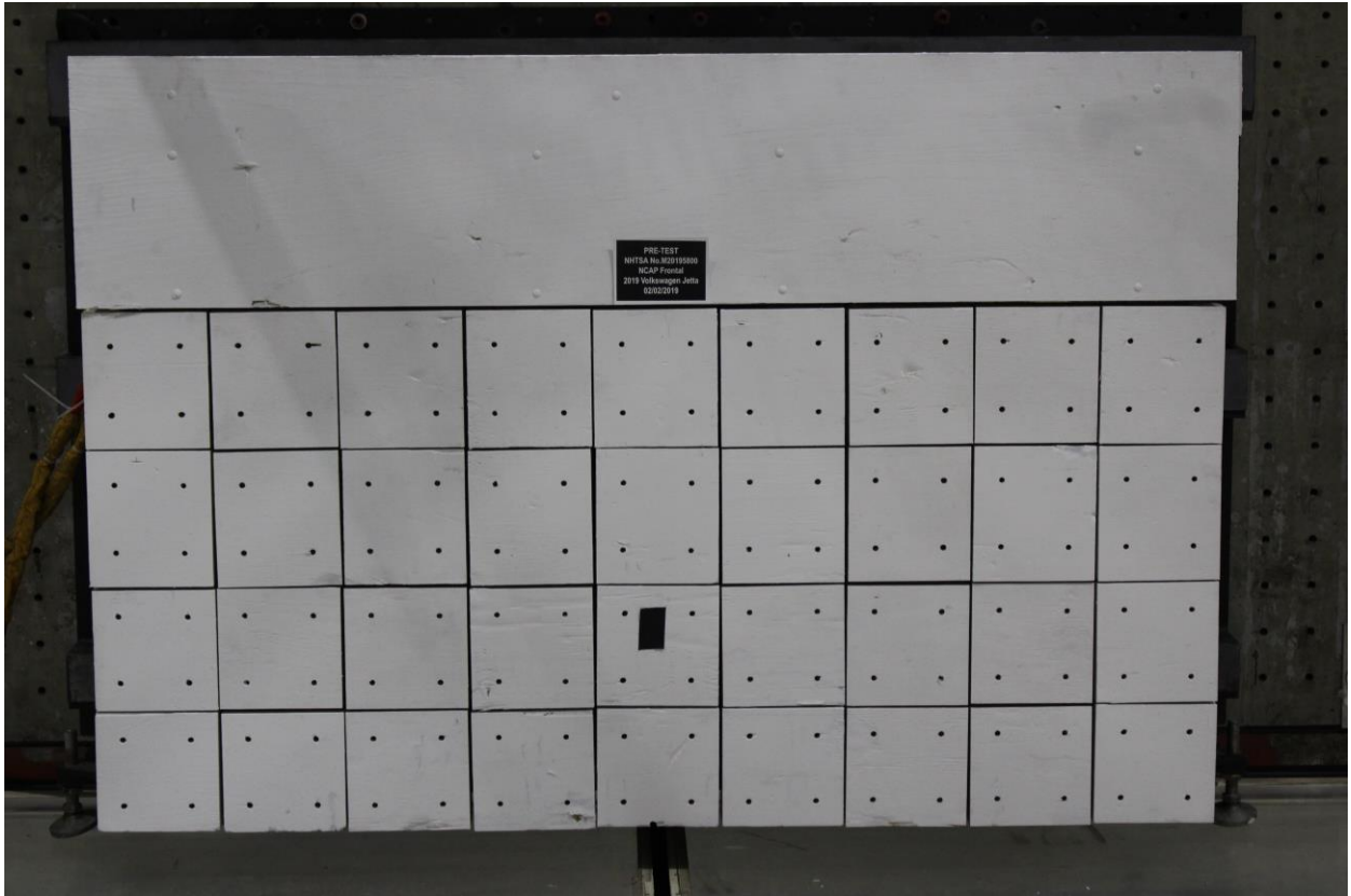
Figure A-2: Pre-Test Load Cell Wall
