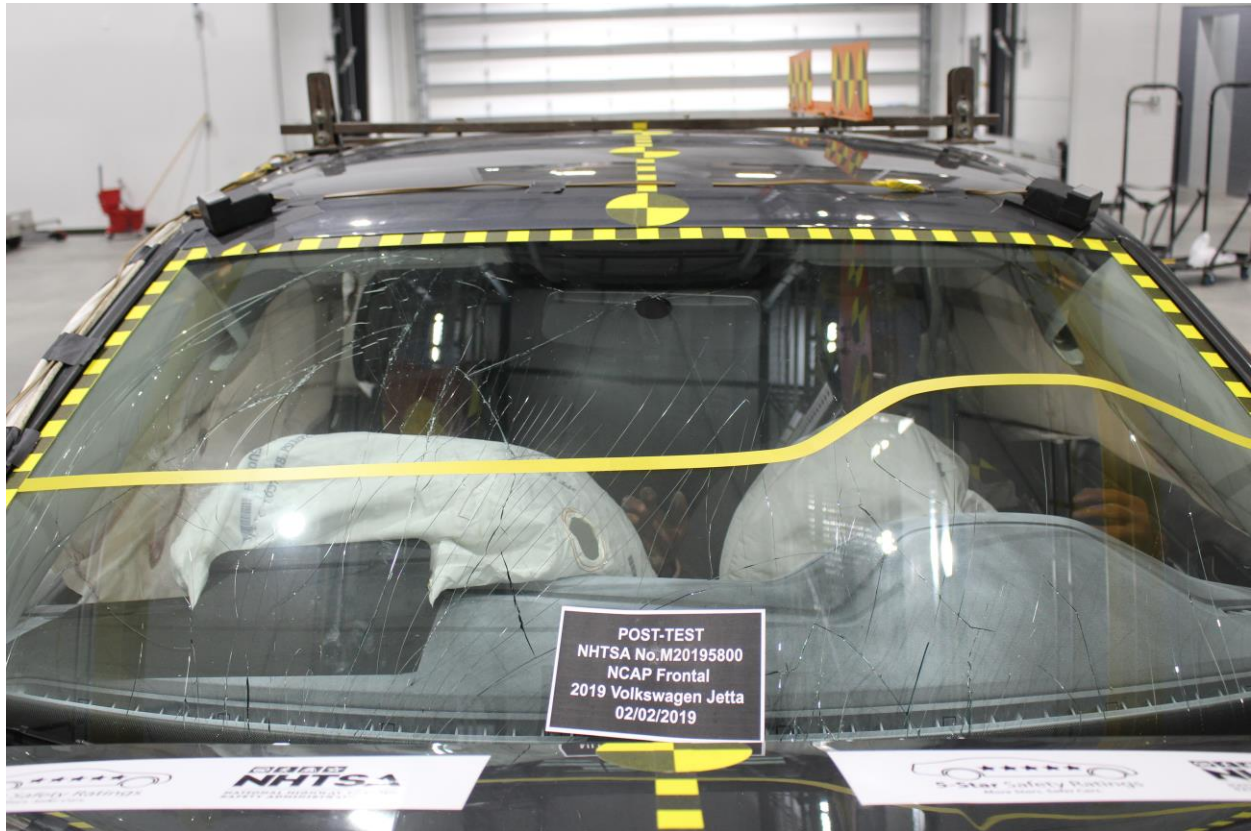
Figure A-19: Post-Test Windshield View
