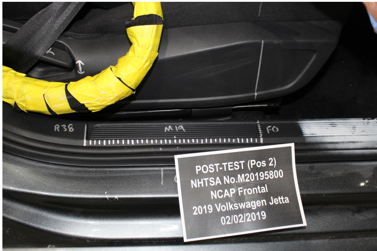
Figure A-58: Post-Test Passenger's Seat Fore-Aft Markings
