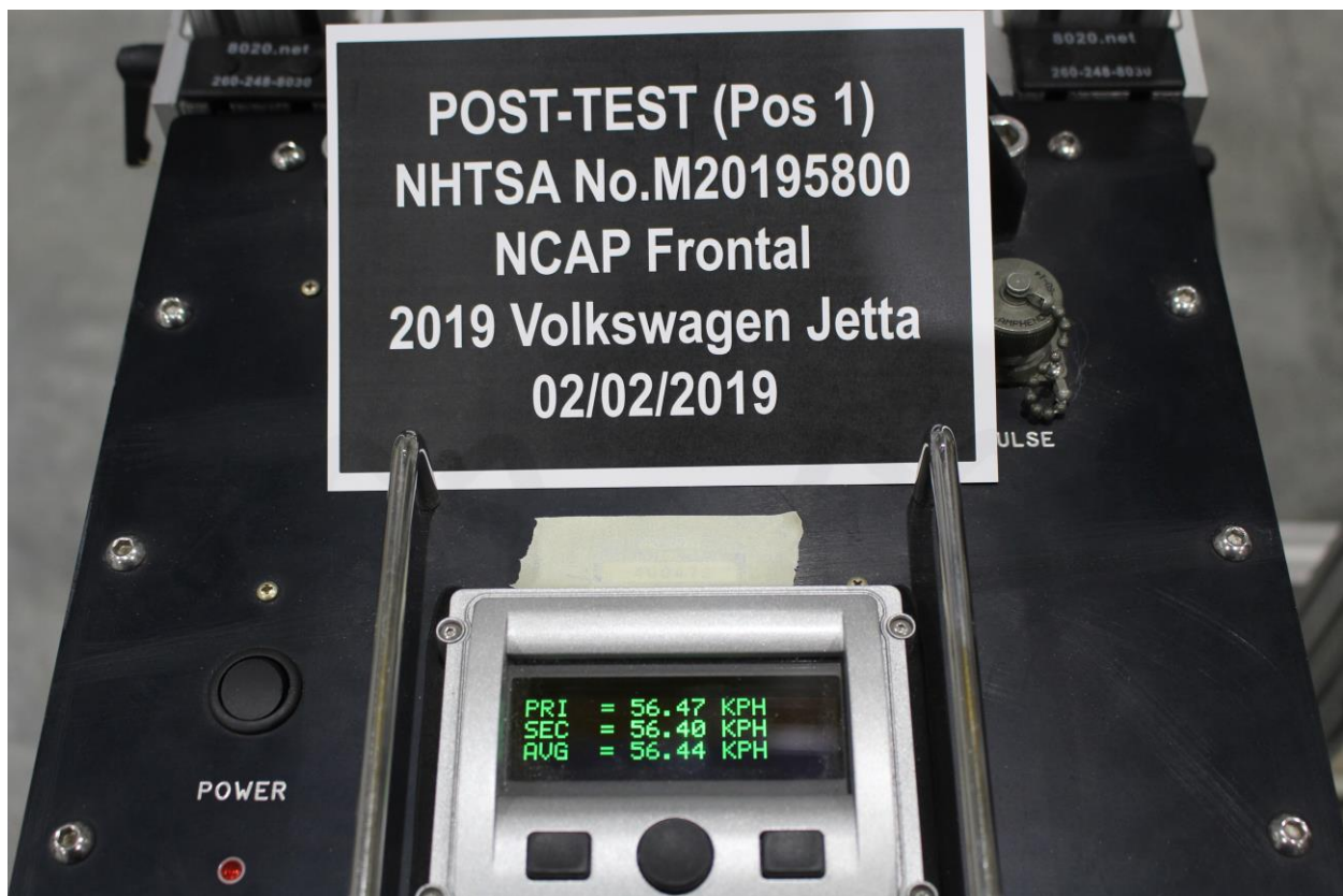
Figure A-72: Post-Test Speed Trap Read-Out
