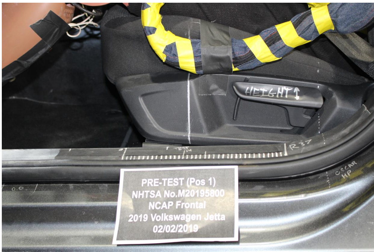
Figure A-36: Pre-Test Driver's Seat Fore-Aft Markings
