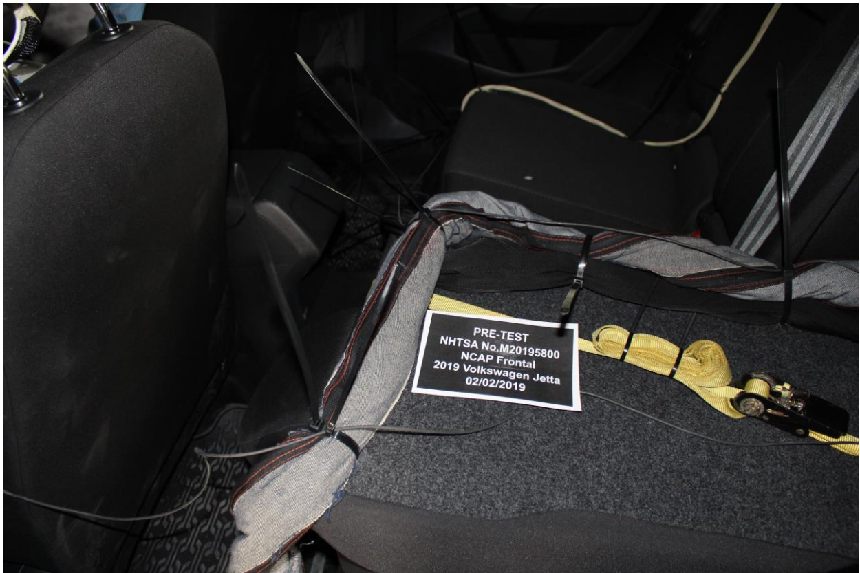
Figure A-28: Pre-Test Dummy Cable Routing
