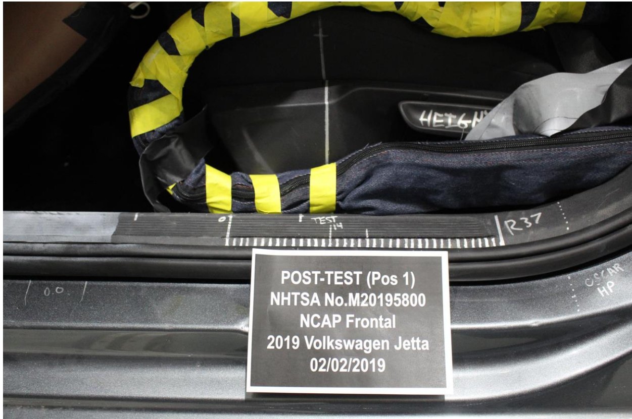
Figure A-37: Post-Test Driver's Seat Fore-Aft Markings
