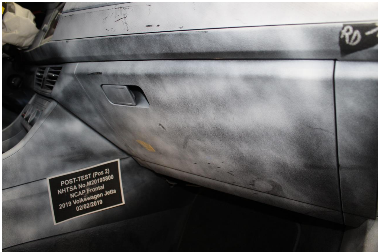
Figure A-64: Post-Test Passenger's Side Knee Bolster
