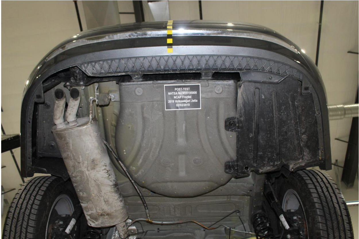
Figure A-27: Post-Test Rear Underbody View
