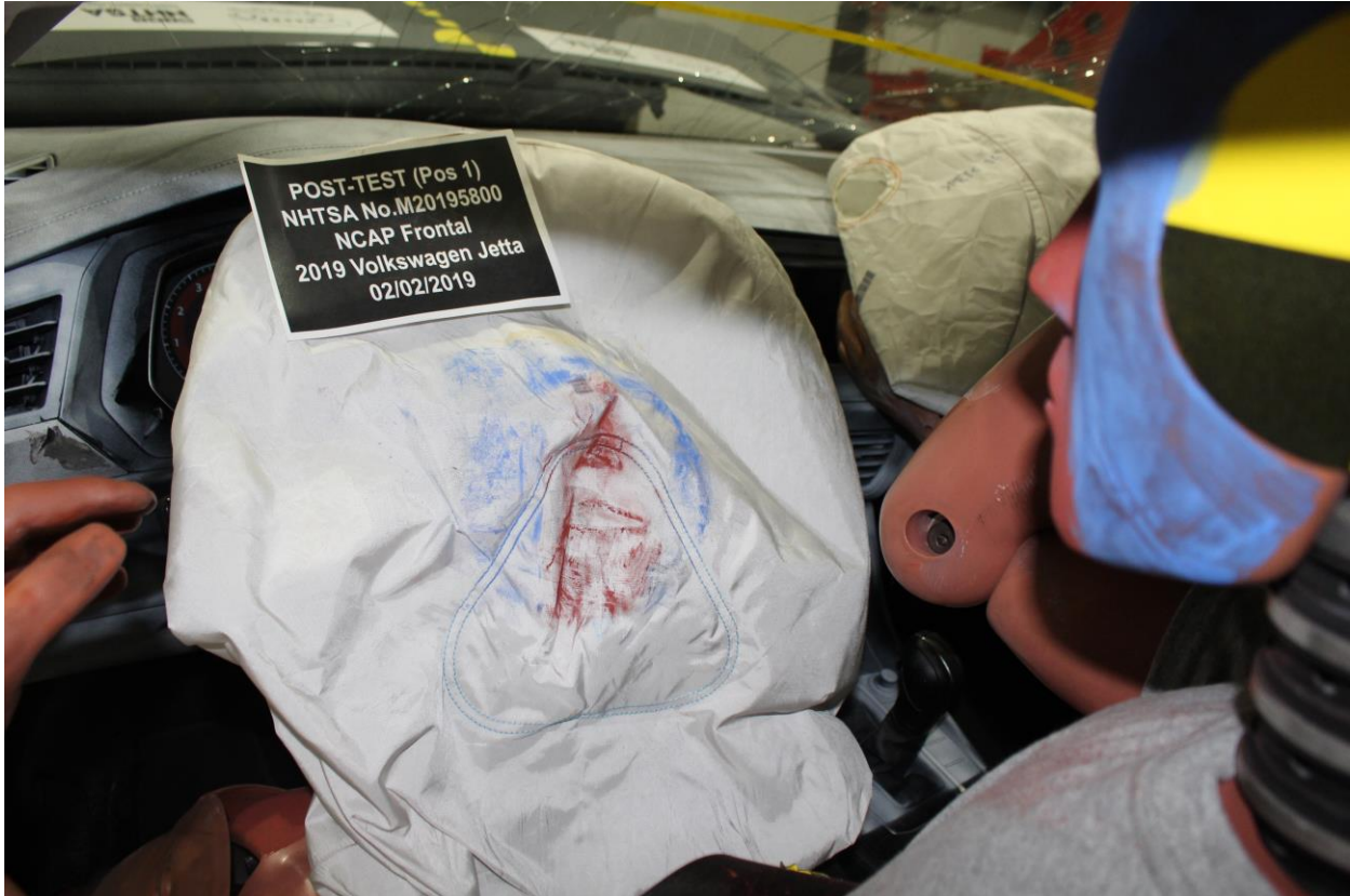
Figure A-47: Post-Test Driver Dummy Contact With Airbag
