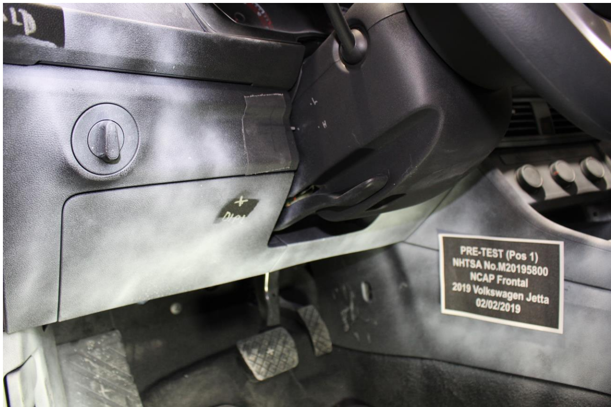
Figure A-42: Pre-Test Driver's Side Knee Bolster
