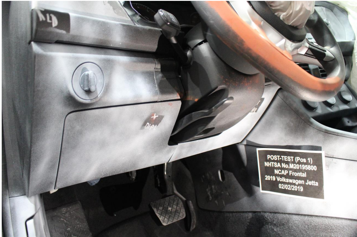
Figure A-43: Post-Test Driver's Side Knee Bolster
