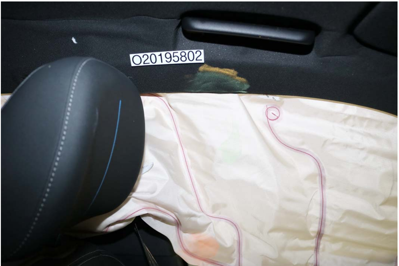
Photo No. 049 - Post-Test Driver Dummy Close-up Head Contact with Side Airbag View
