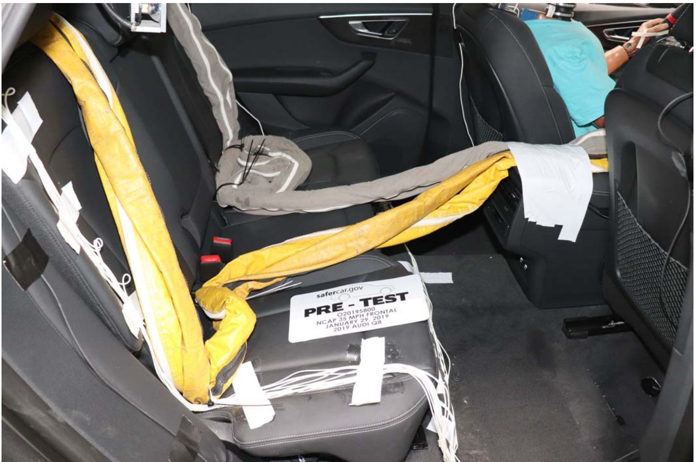
Photo No. 028 - Pre-Test Dummy Cable Routing
