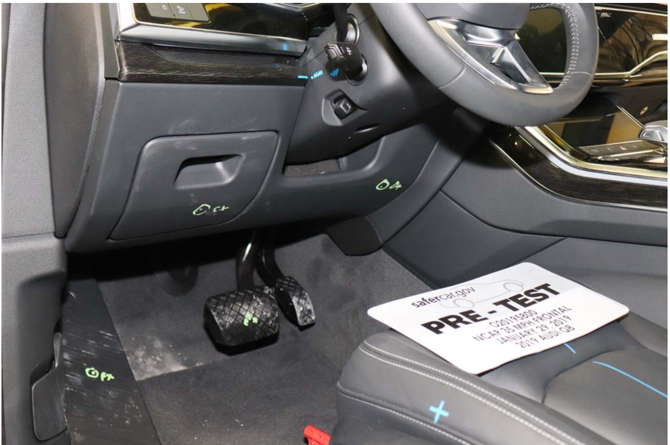
Photo No. 042 - Pre-Test Driver Side Knee Bolster
