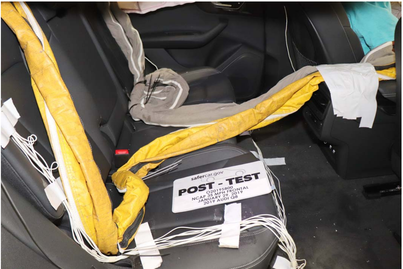
Photo No. 029 - Post-Test Dummy Cable Routing
