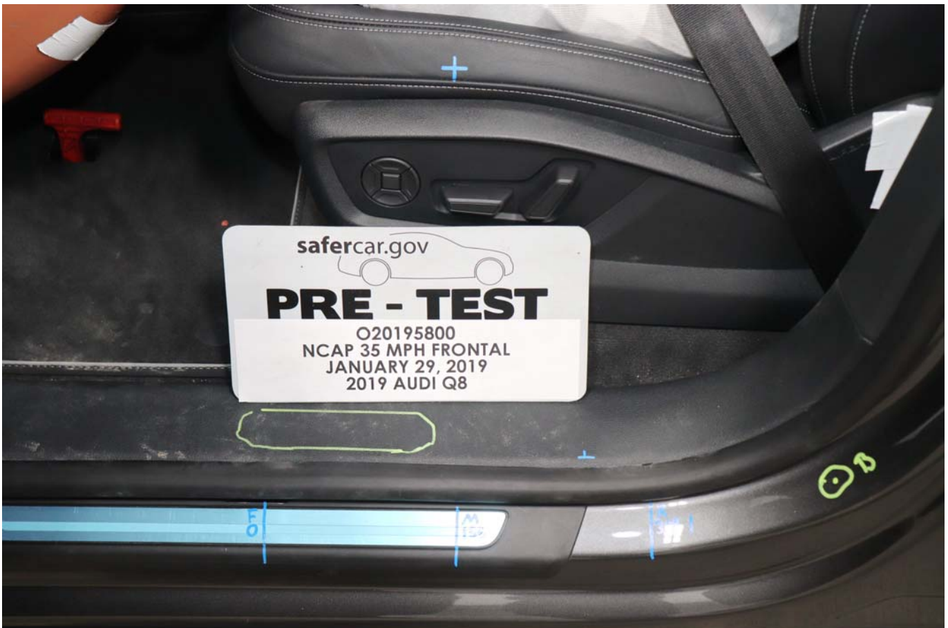
Photo No. 036 - Pre-Test Driver Seat Fore-Aft Markings
