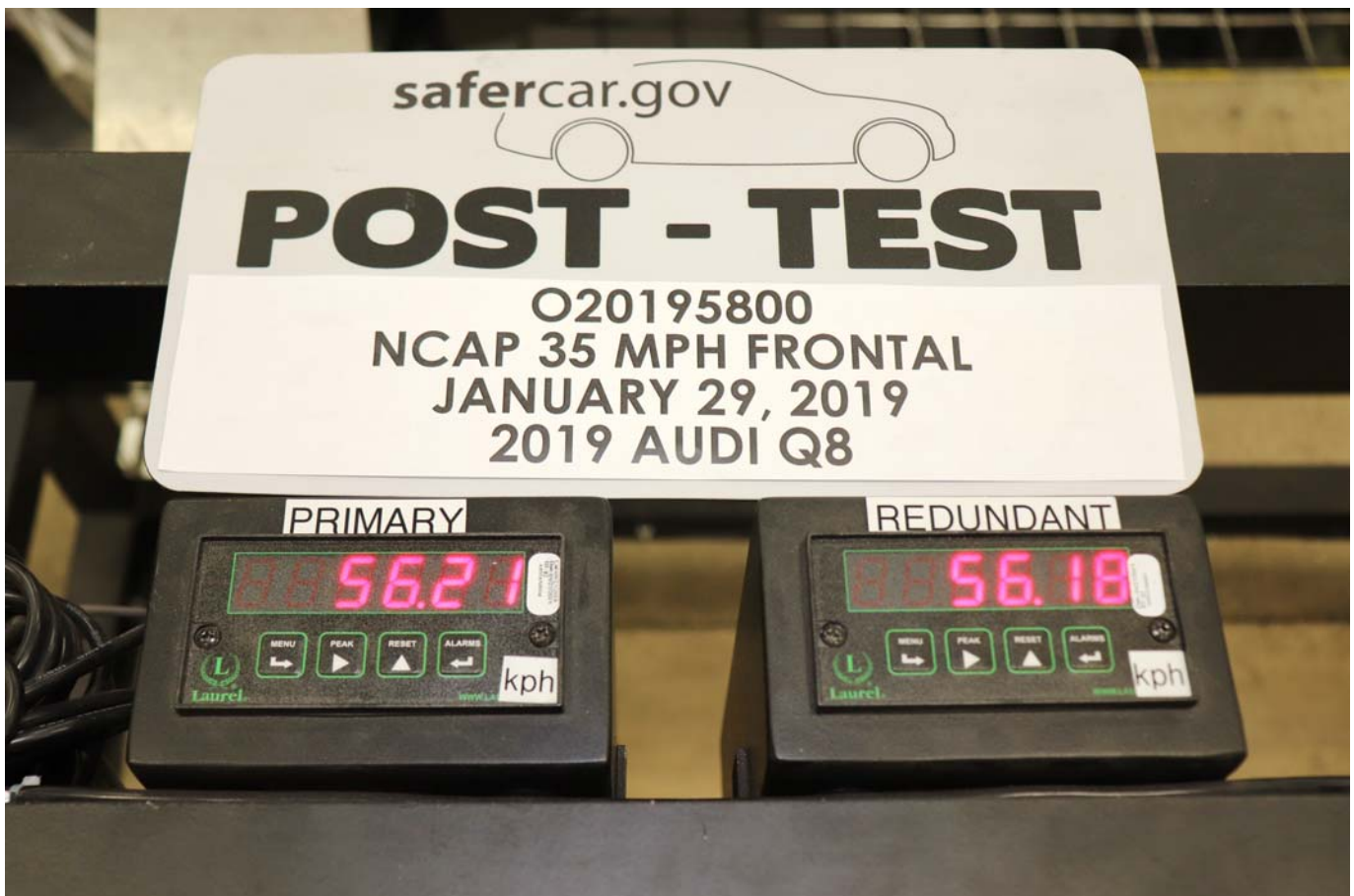
Photo No. 072 - Post-Test Speed Trap Read-Out
