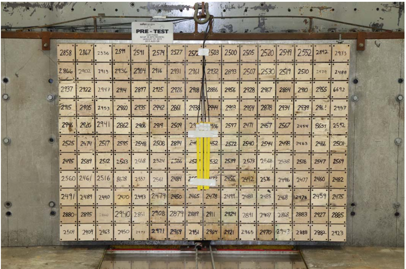
Photo No. 002 - Pre-Test Load Cell Wall
