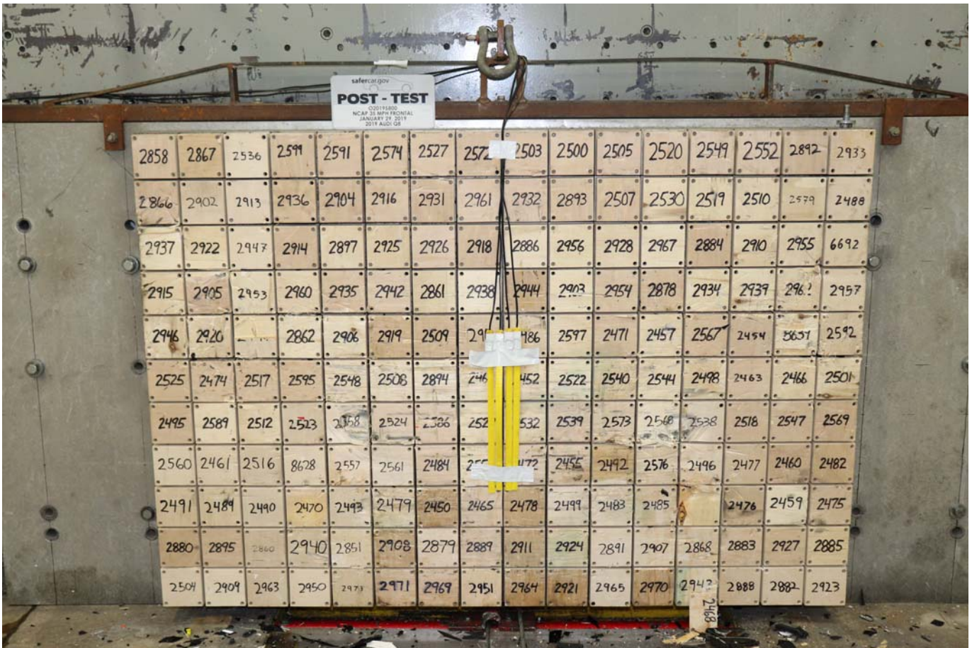
Photo No. 003 - Post-Test Load Cell Wall
