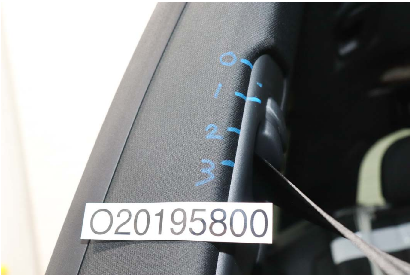
Photo No. 059 - Pre-Test View of Belt Anchorage for Passenger Dummy
