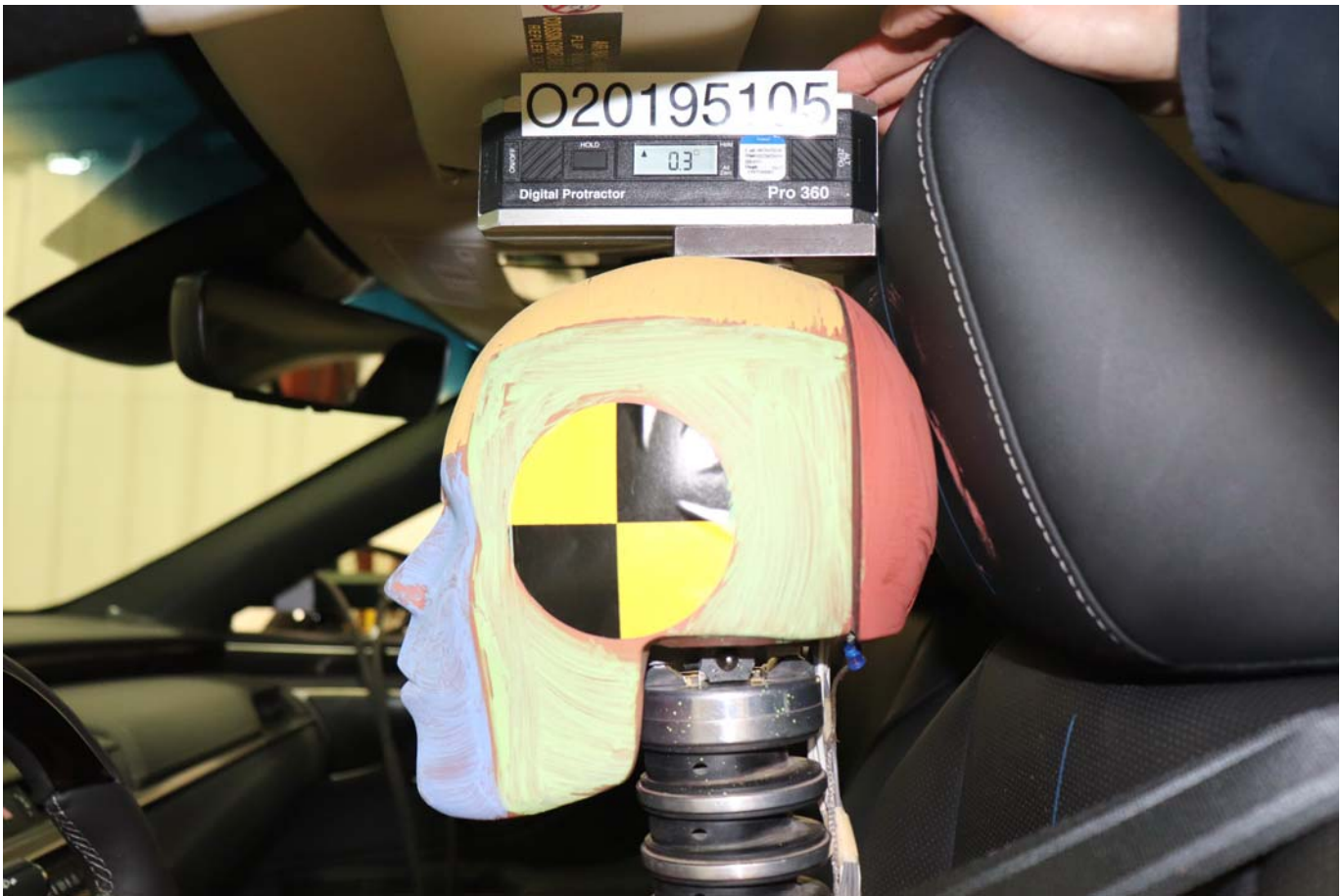
Photo No. 031 - Pre-Test Left Side View of Dummy Head Showing Dummy Head is Level
