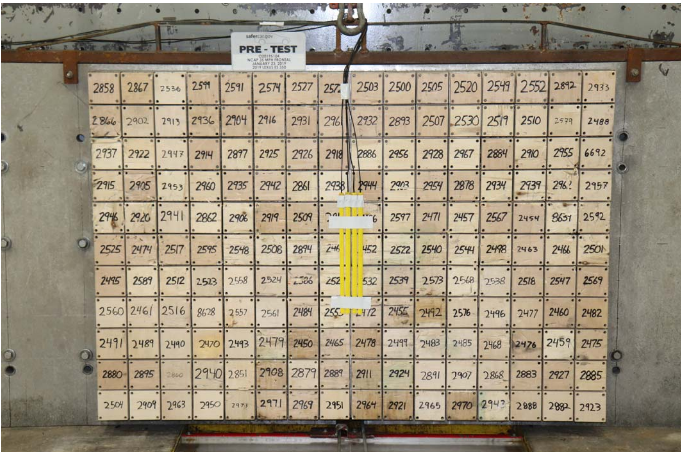
Photo No. 002 - Pre-Test Load Cell Wall
