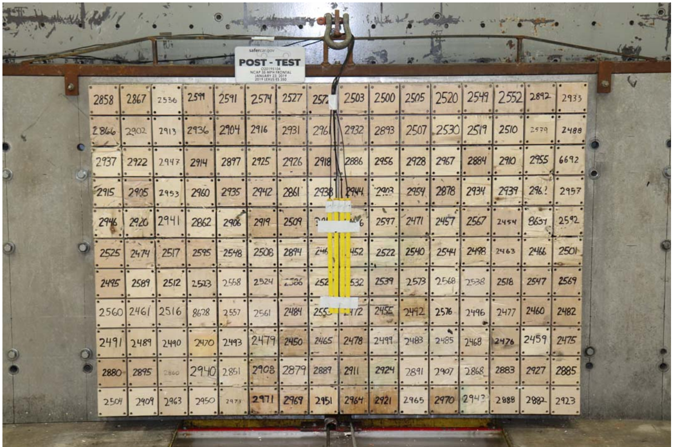
Photo No. 003 - Post-Test Load Cell Wall
