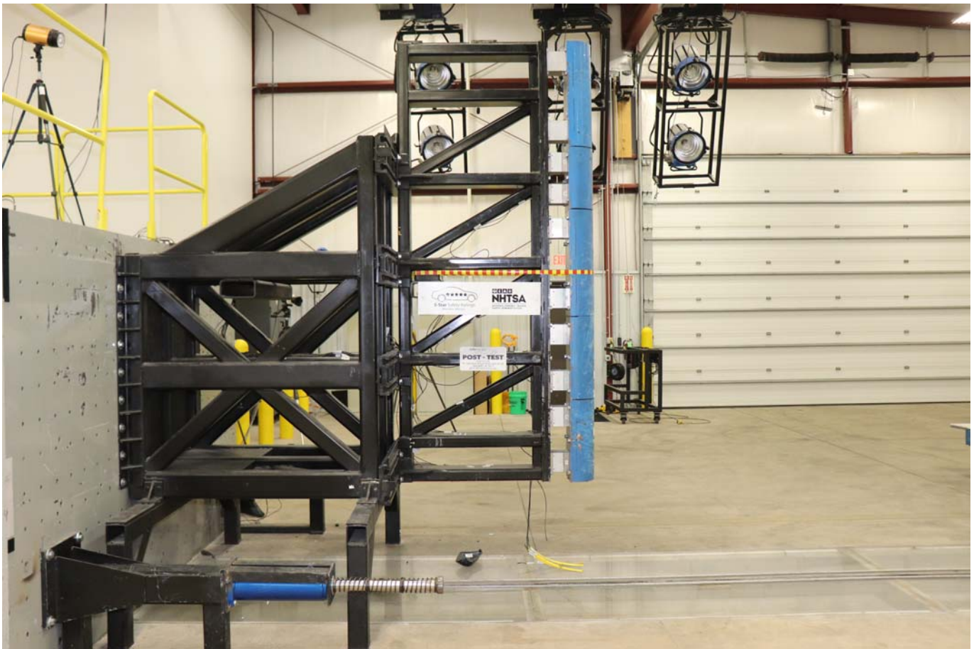
Photo No. 060 - Post-Test Pole Barrier Side View
