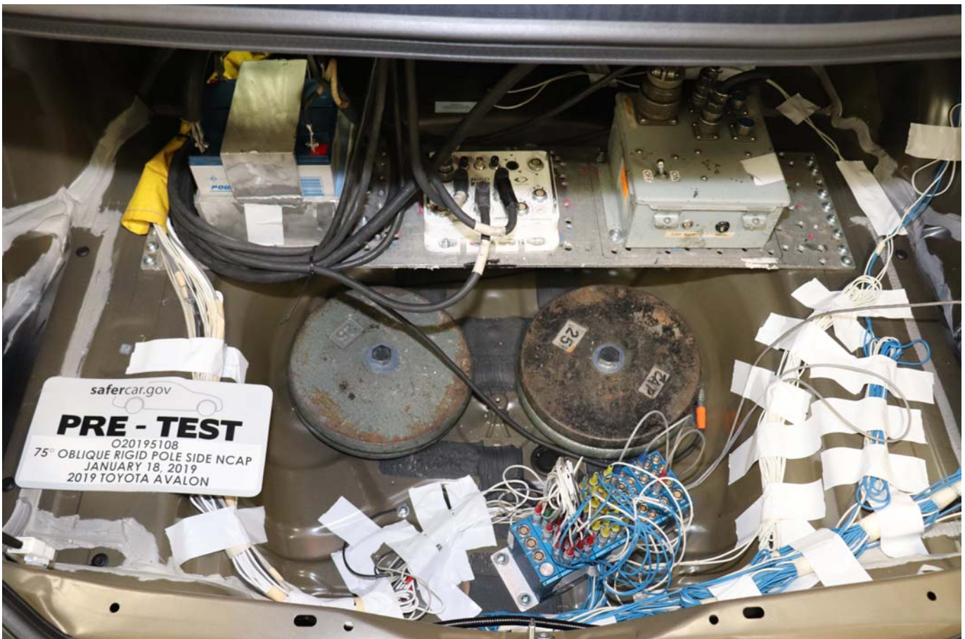
Photo No. 061 - Pre-Test Ballast View
