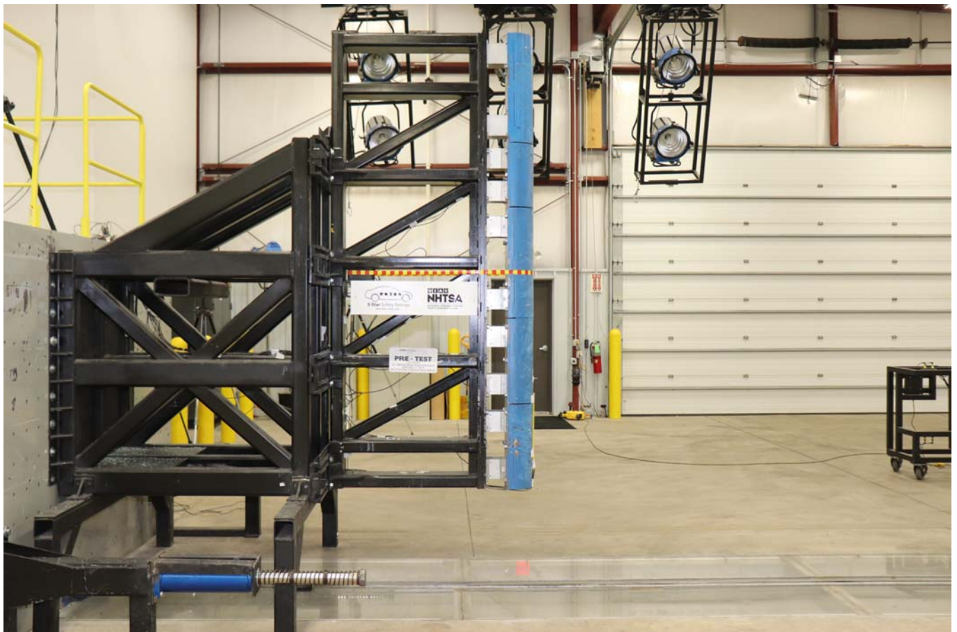
Photo No. 059 - Pre-Test Pole Barrier Side View
